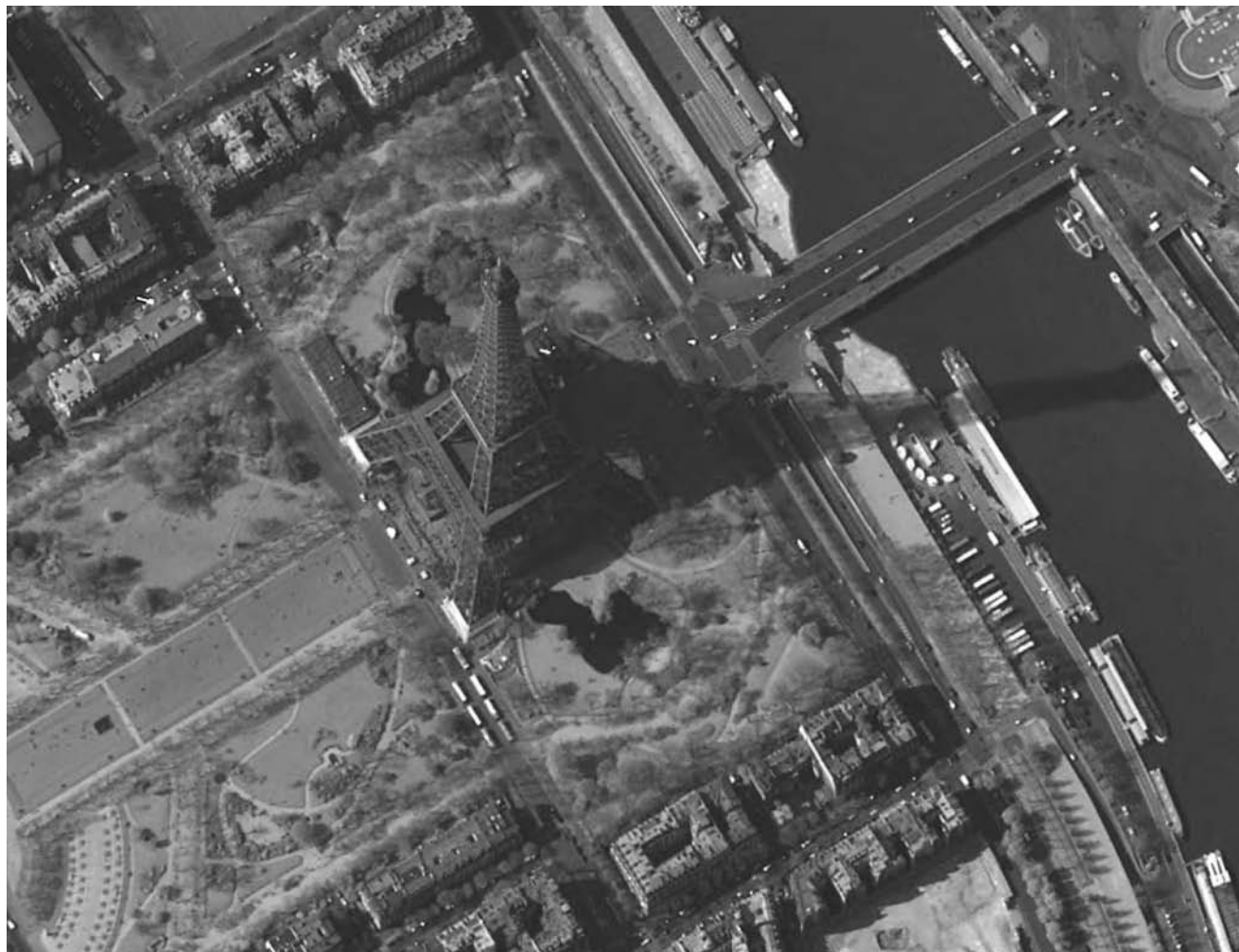
FIGURE 3 Panchromatic image of the Eiffel Tower, Paris, France, with resolution of 61 cm. (Courtesy DigitalGlobe.)
