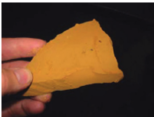
High quality lignin extracted from black liquor (kraft pulp mill)
