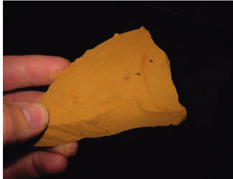
Figure 3.10 Typical LignoBoost softwood lignin from the demo plant. Reproduced with permission from Tomani (2010).
