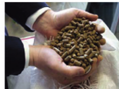
Pellets directly from the pieces of a kraft lignin cake
