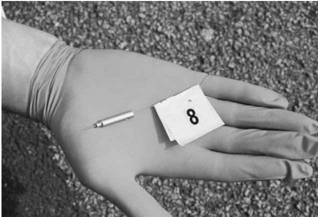
Fig. 7.1. The barb of a Taser with attached wire connected to the gun. (Image courtesy of Dr. J. Bond, Northampton Police, UK.)
