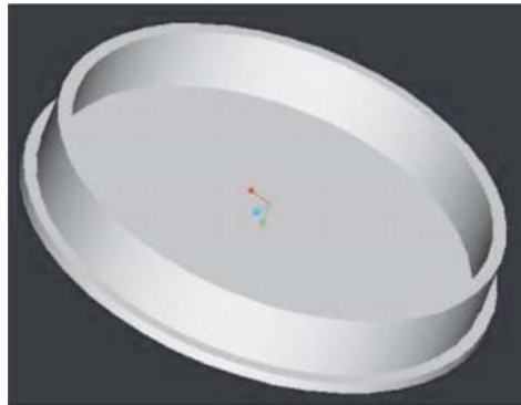
Figure 4: Illustration of Pro-E version of base. After the motor was put into the motor box, the base was fitted into the bottom of the box. The motor housing was sealed to prevent motor from humidity
