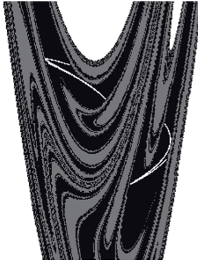
Fig. 1.30. Three basins of attraction for the Hénon map x_{n+1} = ay_n + 1 - x_n^2 , y_{n+1} = bx_n , with a = 0.475 .
