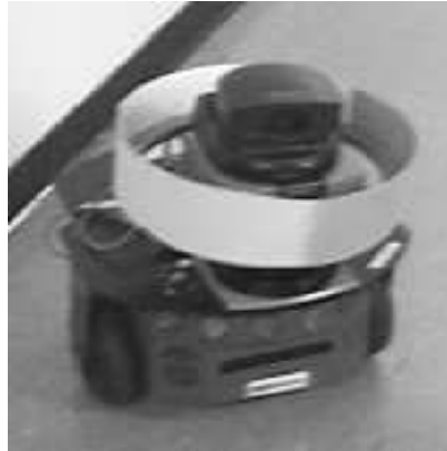
Figure 1: Prototype Pioneer 2DX robot with color markings
