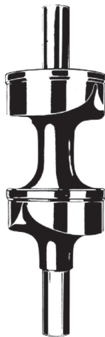
Fig. 17.10 Double port plug for a quick-opening valve.
