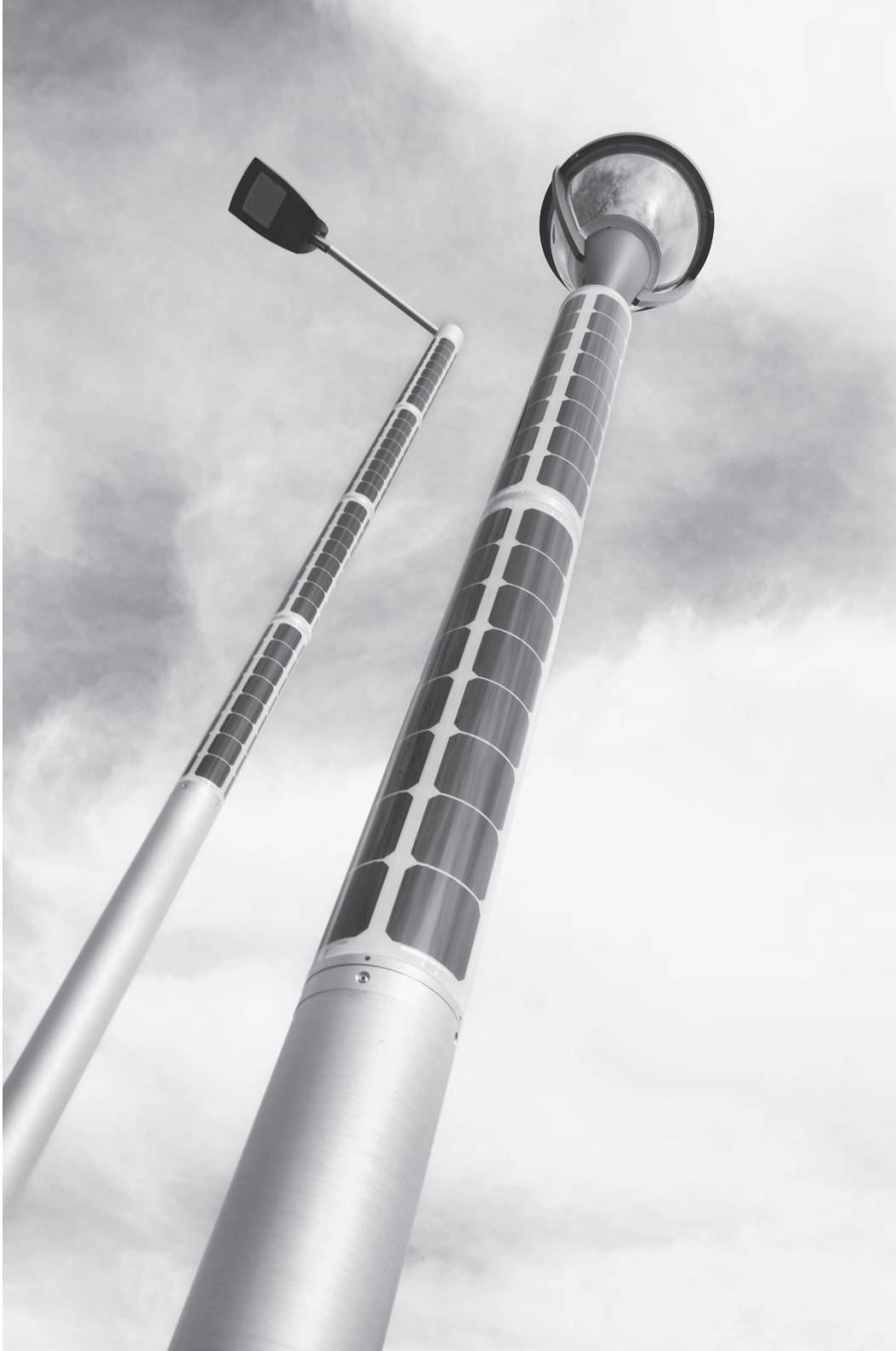
Figure 7.8 Solar panels and streetlights are usually elevated; here the structural Soluxio solar light post also functions as a panel. By rotating the cylindrical pole, the PV cells can be oriented for maximum solar input, avoiding the all-too-common flat panels stuck at awkward angles on top of the luminaire. ( Product and Photo: FlexSol Solutions. )
