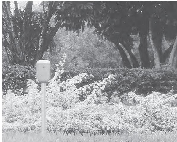
Figure 4.29 Small, solar powered, and radio controlled, LEIT irrigation controllers were among the first to save electricity as well as fuel used in site visits. (Photo: Altec Co. [now DIG Corp.] )
