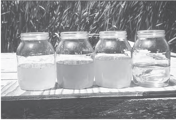
Figure 4.33 Increasing clarity is visible in water from Arcata CA's constructed wetlands, sampled at progressive stages of wastewater treatment. From left: inflow to system; outflows from oxidation pond, treatment marsh, and enhancement marsh. (Photo: Professor Joe Meyer, University of Wyoming.)
