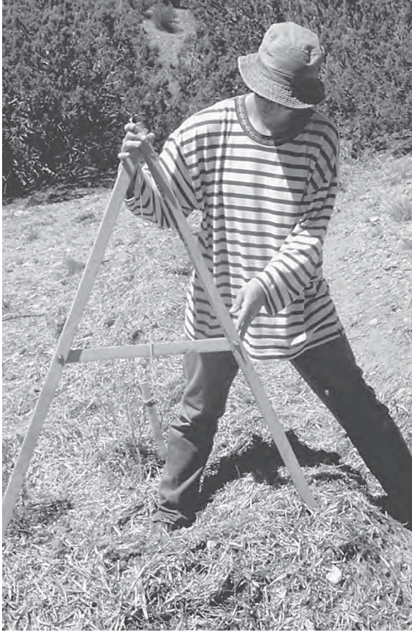
Figure I.7 The Egyptian A-frame is a simple, site-friendly way of establishing level and the fastest way to lay out points along a contour line. (Photo: Kim Sorvig.)
