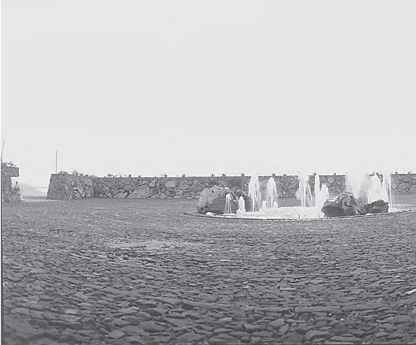
Figure 6.3 Stone from site excavation, reused in walls and paving at Club de Golf Malinalco, makes a stunning argument for inventive use of site “waste.” (Project: Mario Schjetnan. Photo: Courtesy of Grupo de Diseño Urbano.)
