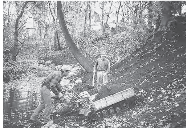
Figure 7.13 Motorized wheelbarrows, like this Honda PowerWagon or the newer Power Carrier, can do heavy work with decreased site impact, as in Sweet Brook’s restoration. (Project: NY DEP. Photo: Dean Cavallaro.)
