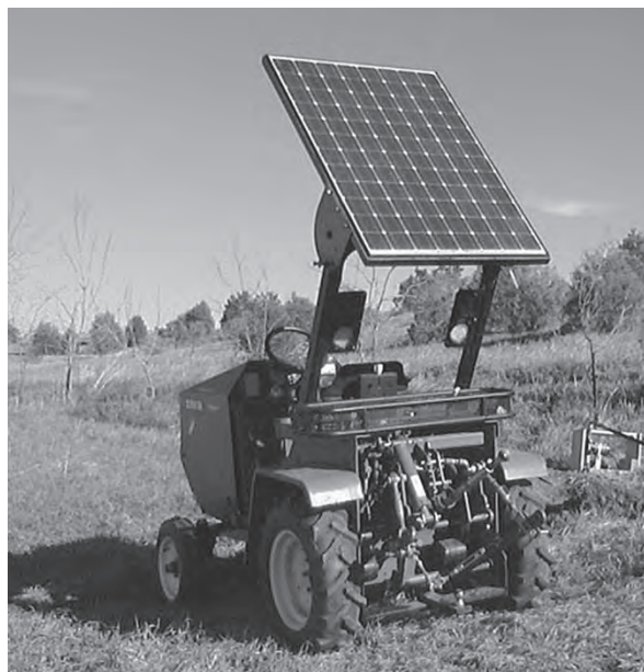
Figure 7.1 The Sun Horse tractor generates its own power with a PV-panel canopy. When not in use, it is often parked near the 12V pump at rear, right, powering irrigation during the night. Both 12V and 110V outlets can power other tools in the field. (Product: FreePowerSystems. Photo: Tom Lopez.)
