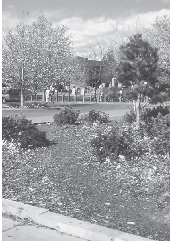
Figure 10.4 “Desire lines” occur at the point pedestrians see their destination. These lines can be counteracted by visual screening (barriers seldom work)—or they can be opportunities to link design to real use patterns. (Photo: Kim Sorvig.)
