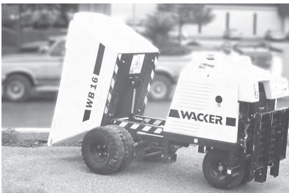
Figure 7.12 “Site dumpers” can be an efficient compromise between hand labor and full-size tractors. (Photo: Kim Sorvig.)
