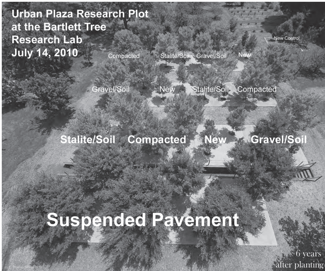
Figure 3.29 Identical saplings were planted in suspended pavement (Silva and Strata products, front row) and various sand- and rock-based supportive soils. The trees in cellular suspended pavement are noticeably larger, as visible in this photo after several years' growth. (Project and Photo: Dr. Tom Smiley, Bartlett Tree Experts.)
