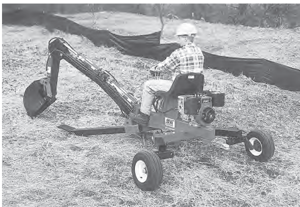
Figure 7.15 Not all machines need to be self-propelled. Trencherman backhoes, by NorthStar, are towed to work; the bucket levers the machine around the site. As of 2017, such machines were found online or at auction; Northern apparently discontinued the model, one of the risks of innovative and sustainable design in a culture that doesn't see the point. (Photo: Northern Tool and Equipment, manufacturer of NorthStar machinery.)
