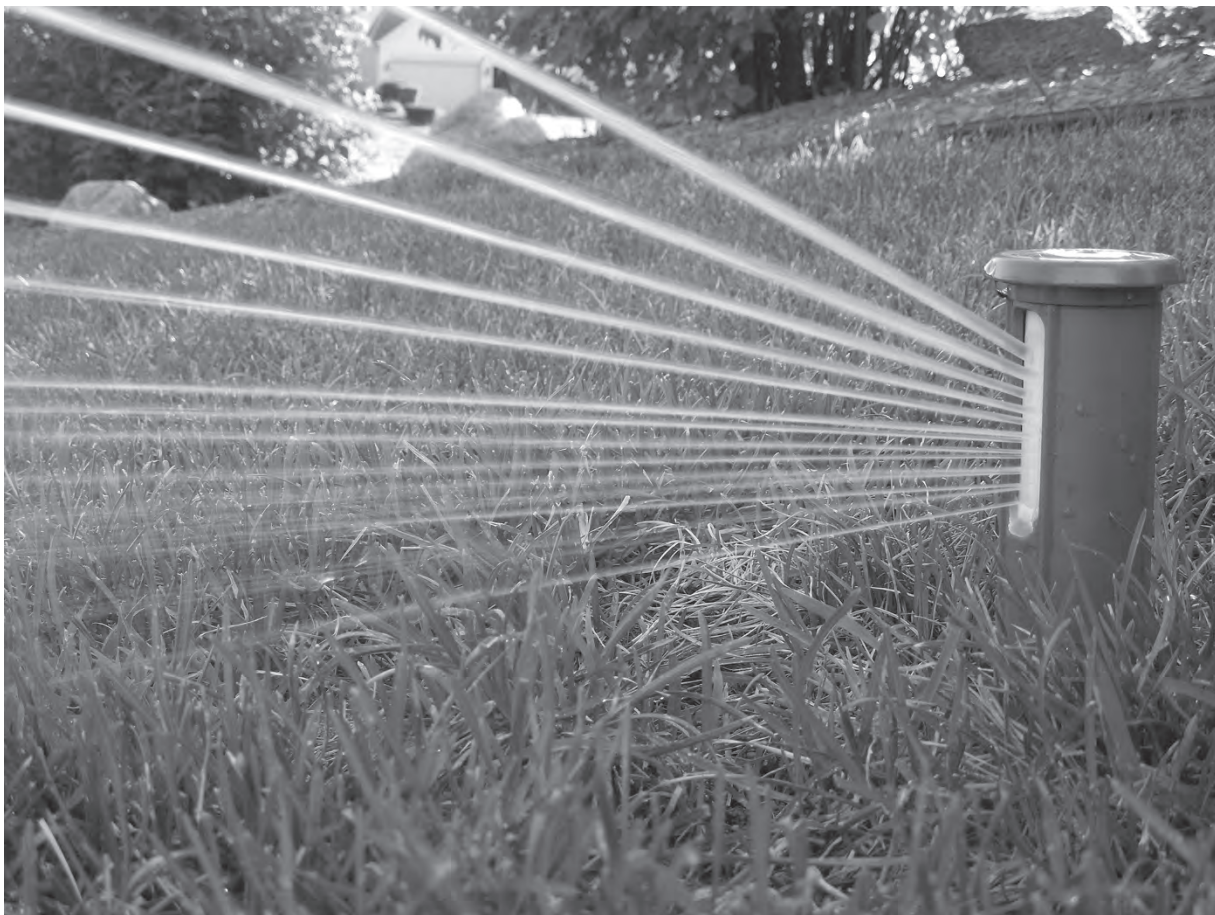
Figure 4.27a, b Centrally located in each irrigation zone, the IrriGreen “Genius” sprinkler is set to variable-length sprays to fit irregular outlines (top) and varied volumes per jet to achieve even coverage (bottom). ( Product and Photos: IrriGreen. )
