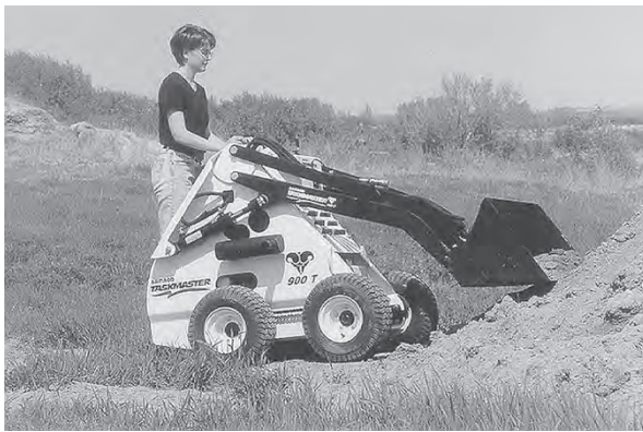
Figure 7.11 This mini skid steer, from Ramrod, fits where larger machines can’t, and has an unusually wide range of attachments. Size generally corresponds to decreased fuel use and ground pressure. (Photo: Ramrod Equipment.)
