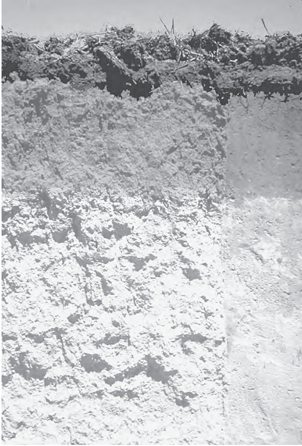
Figure 2.15 In this test pit, living organic topsoil contrasts clearly with light-colored subsoil. A precious resource, topsoil is created from subsoil only by major resource inputs, either from humans or from time. (Photo: Natural Resources Conservation Service.)
