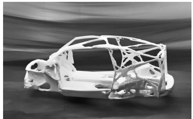
Figures 3-10a, 3-10b, and 3-10c: Engineers at Daimler-Chrysler created a 70-mpg car by mimicking the shape of a coral-reef dweller called boxfish. They lightweighted the skeleton of the car with a software program that uses principles learned from bone growth.
