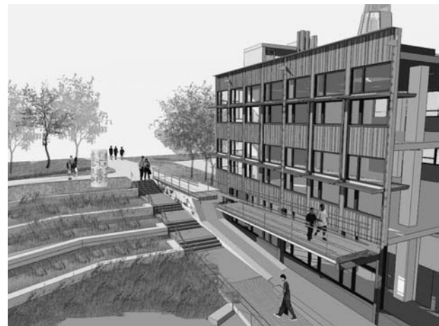
Figure 14-3: Rainwater overflow down sloped spillway into pond and rain garden, Sidwell Friends Middle School
