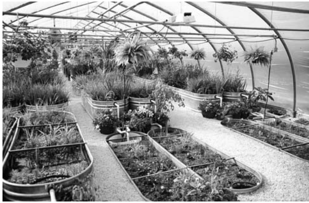
Figure 3-18: Eco-machines from John Todd Ecological Design, Inc. mimic the patterns of nature's water-purifying ecosystems to clean sewage to pure water.
