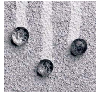
Figures 3-8a and 3-8b: Façade paint manufactured by STO is self-cleaning with rainfall thanks to the Lotus-effect®.
