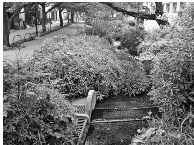
Figure 10-53: Kitazawagawa River Nature Path, Setagaya Ward, Tokyo, follows a reconstructed urban stream brought to grade level and fed by the clean effluent of a local sewage treatment plant. The warm water and its high nutrient content ensures vigorous plant growth along the stream channel.
