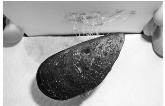
Figure 3-7b: The mussel glue recipe has been mimicked and is being used in all the hardwood plywood produced by Columbia Forest Products, North America's largest manufacturer of hardwood plywood and veneer. The waterproof glue in PureBond™ panels replaces current glues that contain urea formaldehyde, a chemical that degrades indoor air quality.
