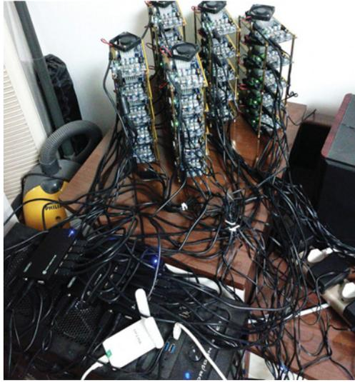
**Figure 6.2** Homemade FPGA Mining Rig
