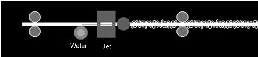
Fig. 2.9: Simplest way to produce air-texturised yarn
