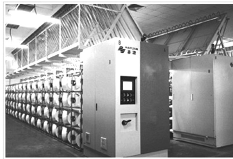
Fig. 2.19: V-type draw texturing machine
