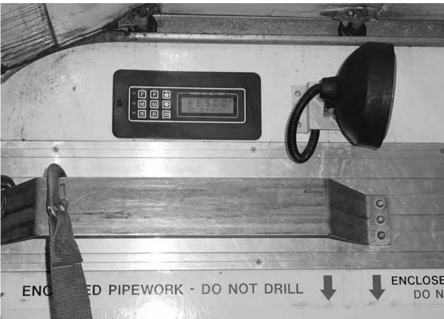
Figure 3.3b Compartment temperature setting
