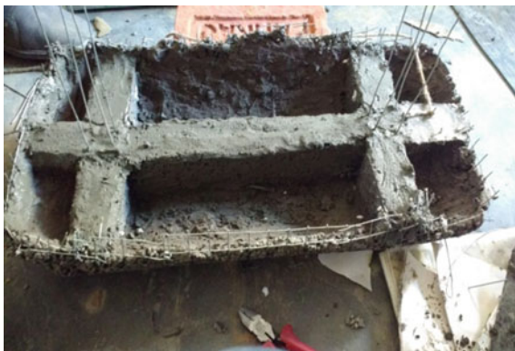
Fig. 3 Modified footing with voids inside
