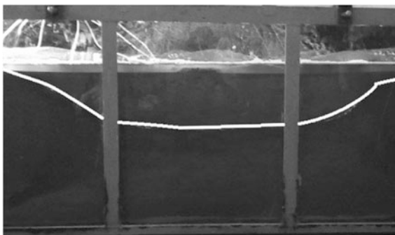
Final Failure - Reinforcement at Base of Embankment
