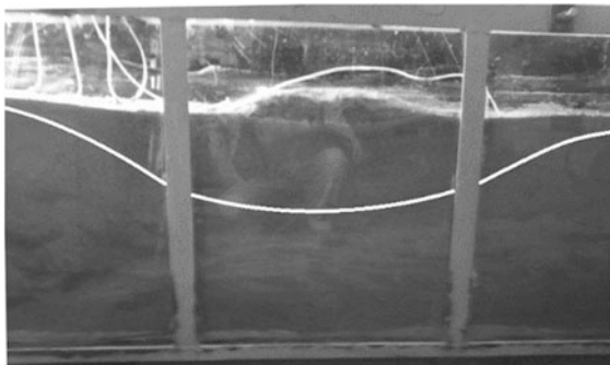
Final failure - No Reinforcement
