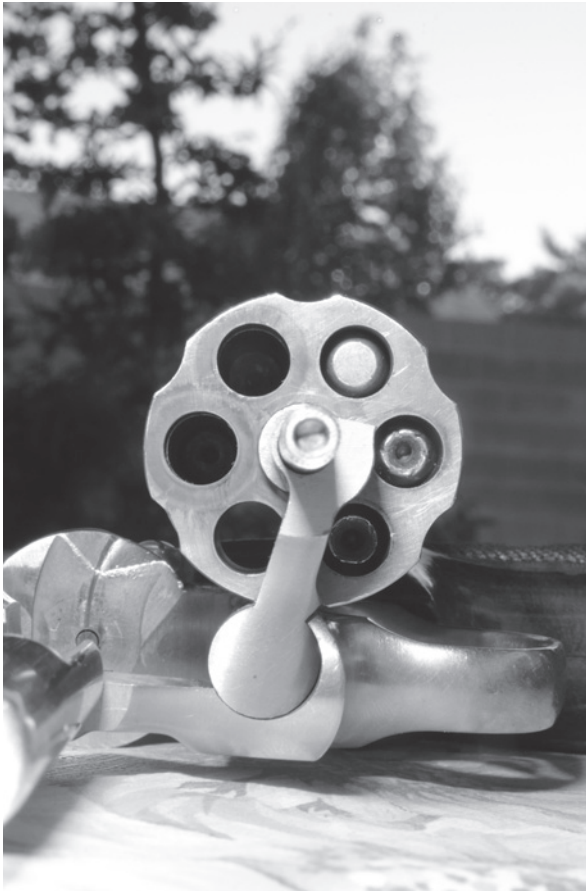
Figure 8.13 Photograph showing the ammunition from the front of the cylinder as well as visible flares/halos around two of the chambers.
