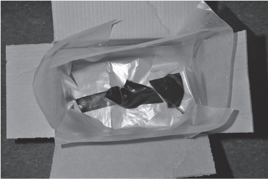
Figure 3.7 Correctly packaged duct tape. This photograph shows utilization of wax paper as a liner on the inside of a cardboard box. The tape will not adhere well to the wax paper and can easily be removed by a latent print examiner.
