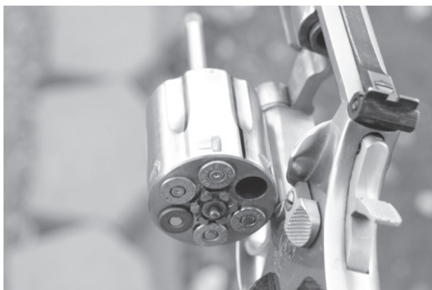
Figure 8.11 Photograph showing the top of the cylinder, scribed on either side of the top strap for orientation of the cylinder.
