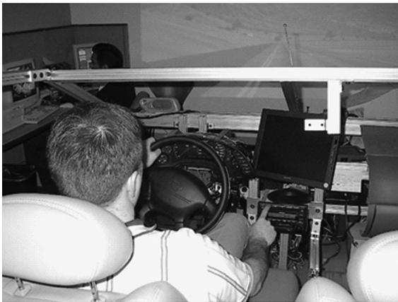
**FIGURE 22.10** Subject operating a radio while driving in a vehicle simulator.
