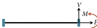
Figure 1.23 Three possible “actions” corresponding to deformations on three DOFs on right end.
