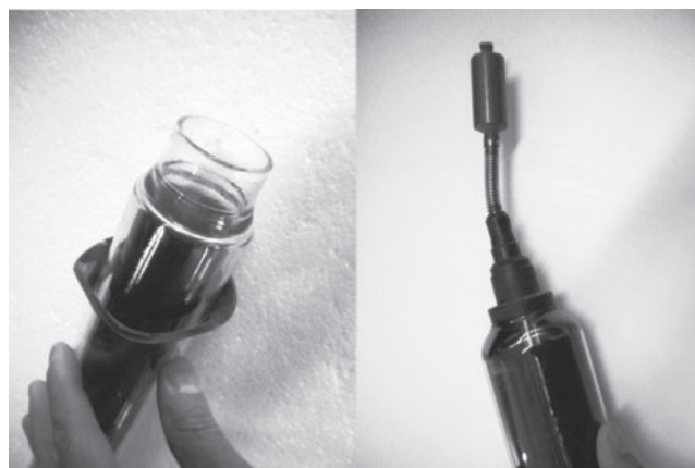
Figure 4-5. An evacuated-tube solar collector consists of two glass tubes welded together or an evacuated glass tube enclosing the absorber plate and a heat pipe assembly to remove the heat, as shown in this close-up photograph of the heat-pipe condenser bulb. (Photo by the author)
