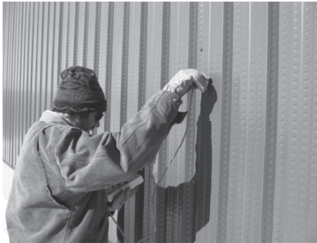
Figure 5-14. Photograph of Greg Barker measuring pressure drop with a cup held over a hole in the transpired solar collector. (Photograph courtesy of Ed Hancock).
