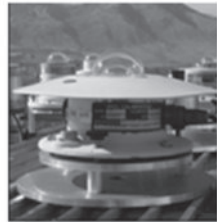
Figure 2-16. Instruments used to measure solar radiation include pyrheliometer to measure direct beam, shaded pyranometer to measure diffuse, and pyranometer to measure global insolation. (Photo by Tom Stoffel, courtesy of DOE/NREL, Pix# 06821, 06231, 06232)
