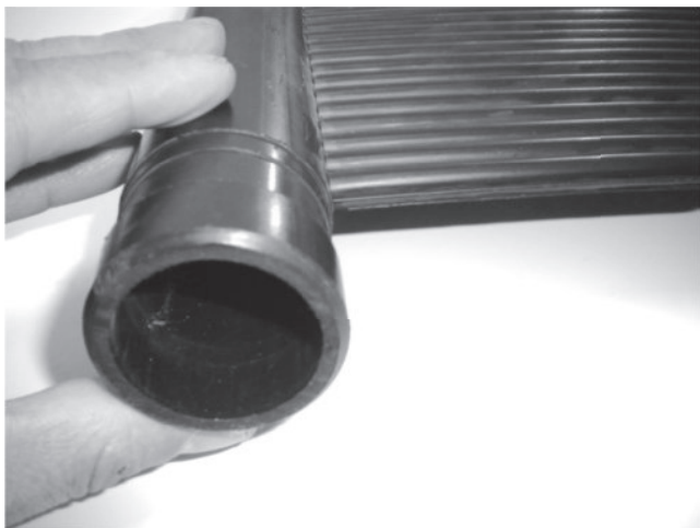
Figure 4-3. An unglazed solar collector for heating swimming pool water is made of flow passages extruded in plastic, as shown in this close-up photograph. (Photo by the author)
