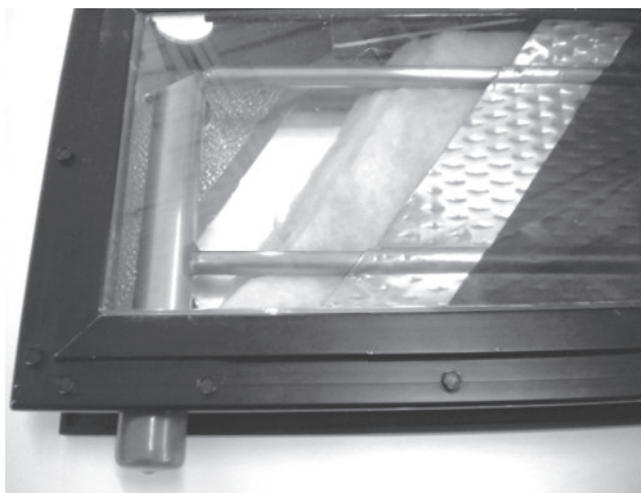
Figure 4-4. A glazed flat-plate solar liquid-heating collector includes a cover glass, absorber plate with selective surface, riser tubes, manifold and insulation, as shown in this cut-away sample. (Photo by the author)
