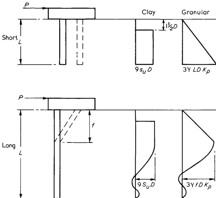
Fig.6.19 Failure mechanisms for short and long restrained piles, after Broms (1965)
