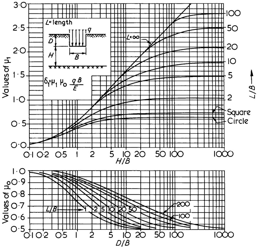
Fig. 3.6 Diagrams for the factors  $\mu_0$  and  $\mu_1$  used in the calculation of the immediate average settlement of uniformly loaded flexible areas on homogeneous isotropic saturated clay, after Janbu, Bjerrum and Kjaernsli (1956)
