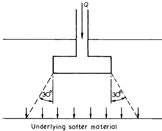
Fig.4.5 Spread of load onto underlying layer
