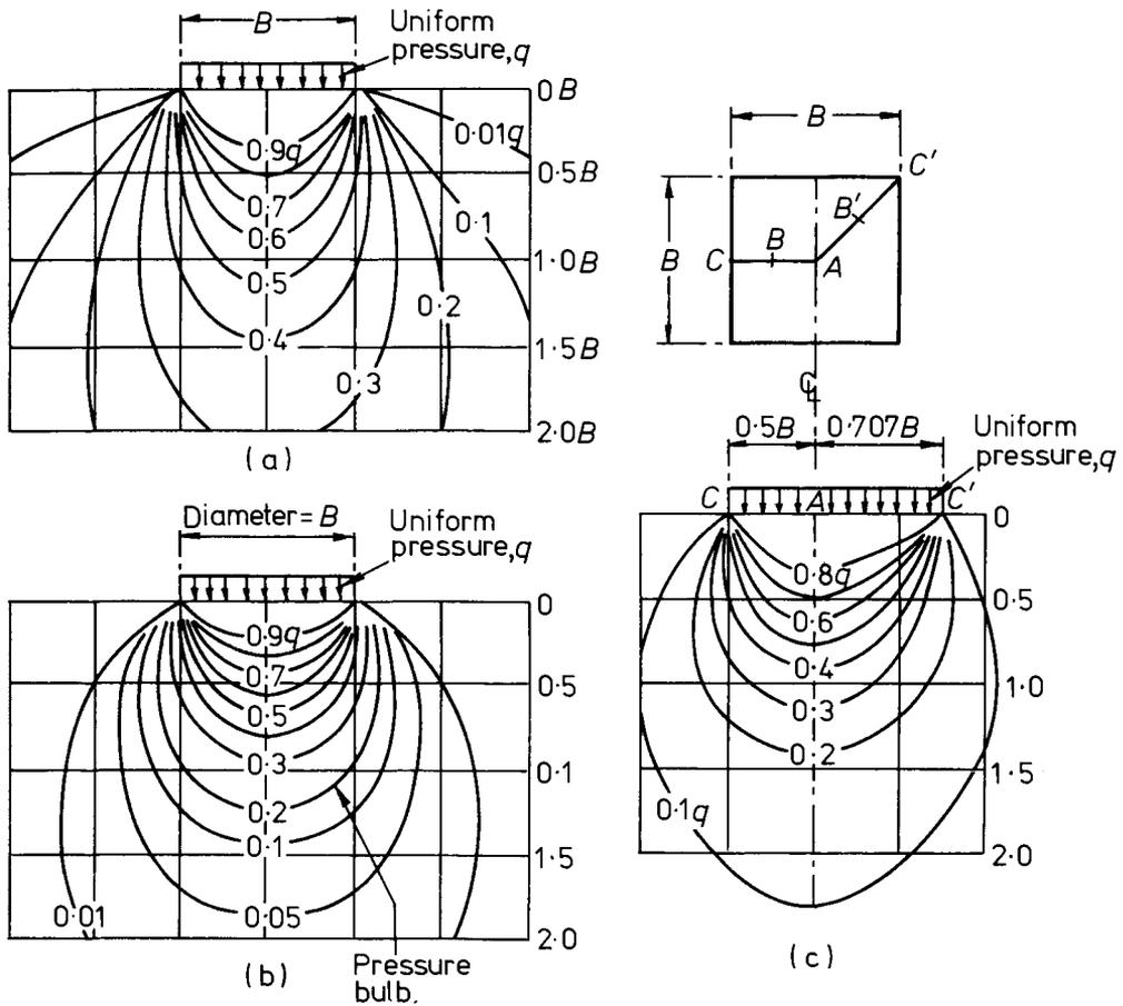
Fig.3.1 Vertical stresses under uniformly loaded flexible footings resting on a deep wide homogeneous isotropic elastic solid, after Teng (1962): (a) strip footing; (b) circular footing; (c) square footing
