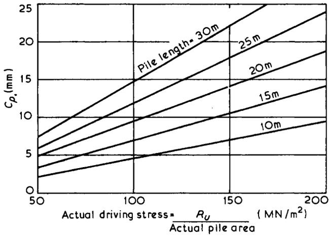
Fig. 6.11 Determination of temporary elastic compression  $C_p$ , for steel piles, after BSP Pocket Book (1969)
