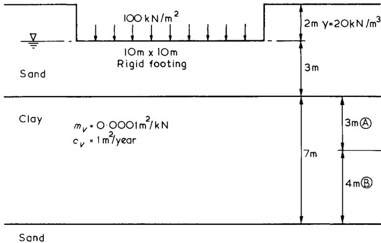
Fig.5.7 Example of calculation of primary consolidation settlement
