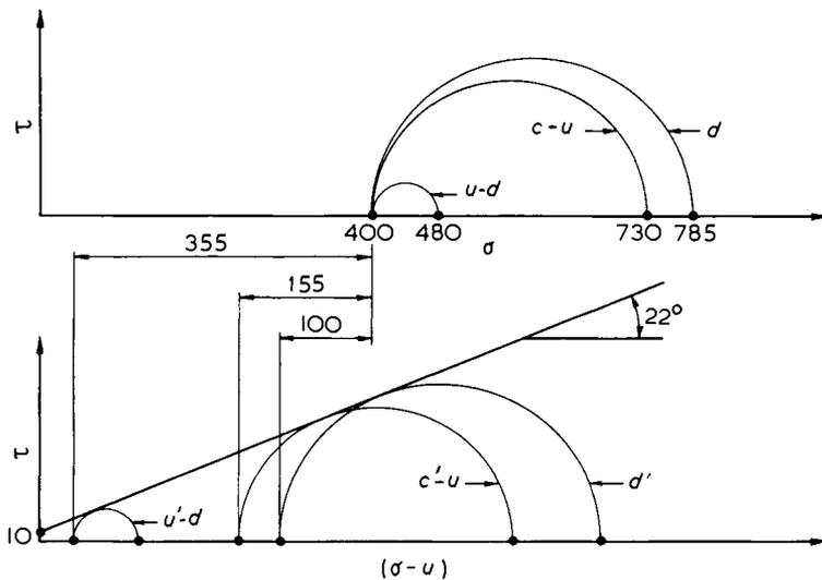
Fig.2.13 Correlation between undrained (*u-d*), consolidated-undrained (*c-u*) and drained (*d*) triaxial compression tests for specimen number 2
