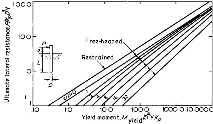
Fig. 6.24 Ultimate lateral resistance for long piles in granular soils, after Broms (1965)
