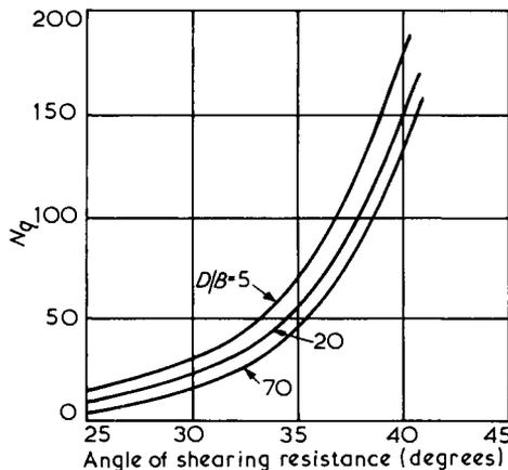
Fig. 6.6 Relationship between  $N_q$  and  $\phi'$ , after Berezantsev (1961)
