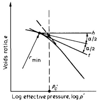
Fig.5.4 (a) Relationship between voids ratio and effective pressure; (b) relationship between voids ratio and the logarithm of effective pressure
