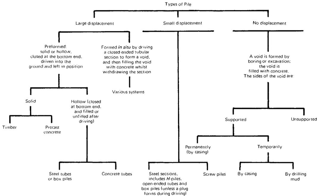
*Fig. 6.1 Classification of piling systems*
