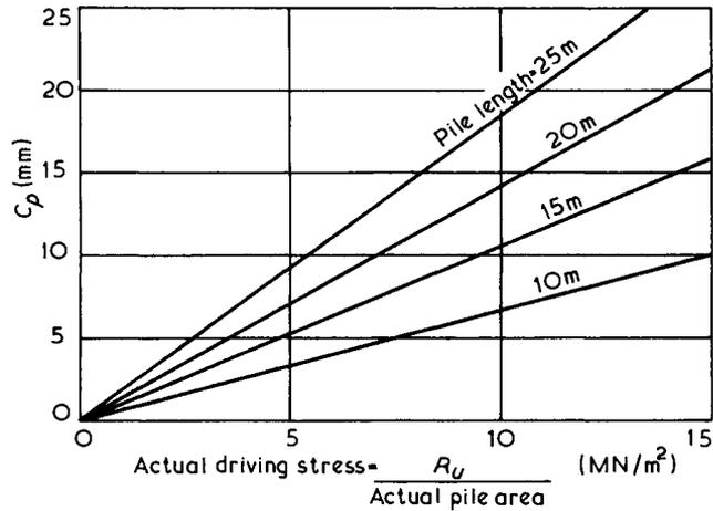
Fig.6.10 Determination of temporary elastic compression  $C_p$ , for concrete piles, after BSP Pocket Book (1969)
