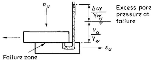
Fig.2.3 Stresses at undrained failure in the direct shear box
