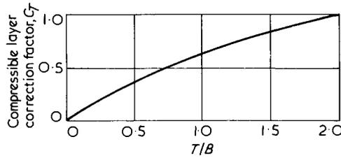
Fig. 5.28 Correction factor for thickness of compressible material, after Parry (1971)
