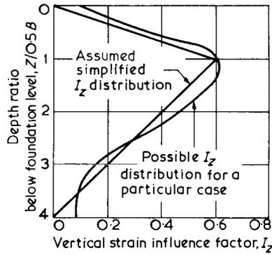
Fig.5.21 Variation of strain influence factor with depth, after Schmertmann (1970)
