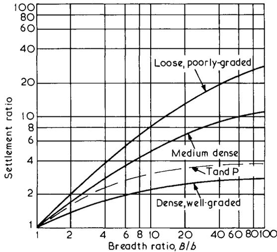
Fig.5.20 Relationship between settlement ratio and foundation to plate size ratio, after Terzaghi and Peck (1948) and Bjerrum and Eggestad (1963)
