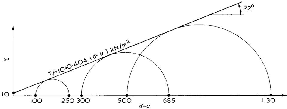
Fig. 2.12 Failure envelope for drained triaxial compression test
