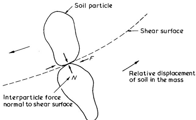
Fig.2.1 Forces arising at inter-particle slip
