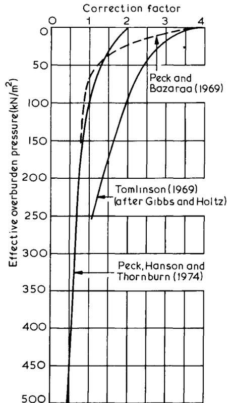
Fig.5.25 Correction factor for influence of effective overburden pressure on SPT 'N' value, after Tomlinson (1969), Peck and Bazaraa (1969) and Peck, Hanson and Thornburn (1974)
