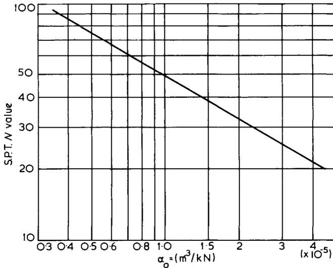
Fig. 5.31 Determination of  $\alpha_o$ , for high SPT 'N' values, after Alpan (1964)
