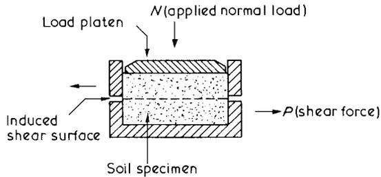
Fig.2.2 A schematic section through the direct shear box
