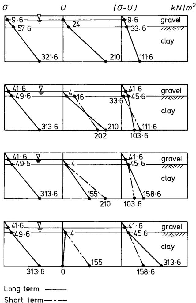
Fig.1.5 Solution to worked example, section 1
