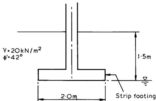
Fig.4.3 Example of bearing capacity calculation
