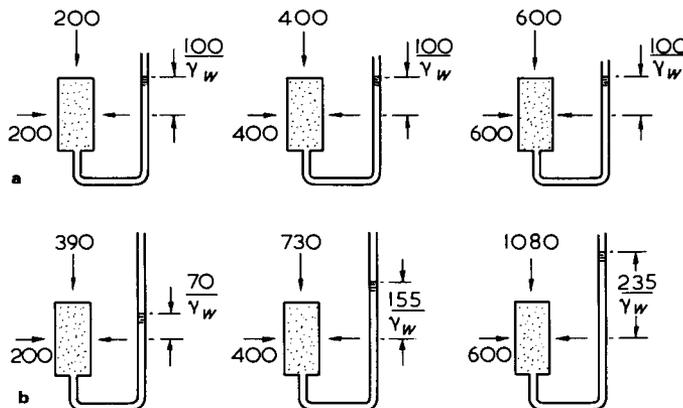
Fig.2.10 Stress diagrams for the consolidated-undrained test. (a) application of cell pressure. Drainage to back pressure of  $100 \text{ kN/m}^2$ ; (b) application of axial load to failure, undrained
