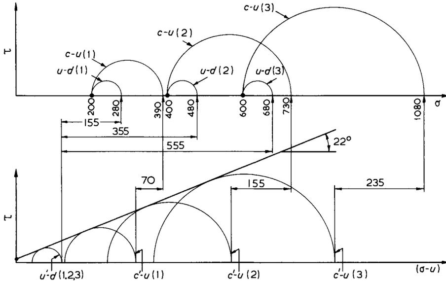
Fig.2.9 Typical undrained (u-d) and consolidated undrained (c-u) triaxial compression test Mohr's circles in terms of total stress and effective stress
