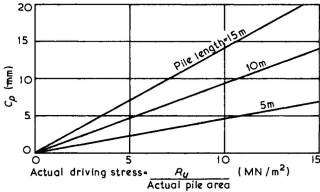
Fig. 6.12 Determination of temporary elastic compression  $C_p$ , for timber piles, after BSP Pocket Book (1969)
