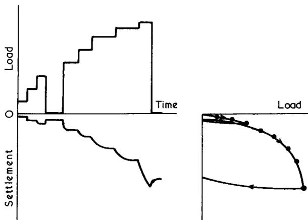
Fig.6.26 Results of a maintained load pile test
