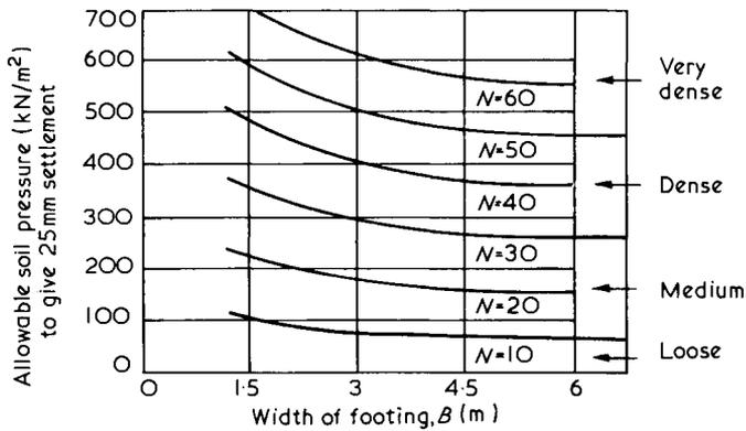
Fig.5.24 Correlation of allowable bearing pressure to give 25 mm settlement to SPT 'N' value, after Terzaghi and Peck (1948)
