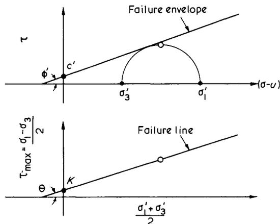
Fig.2.14 Stress-path representation of top point of Mohr's circle at failure
