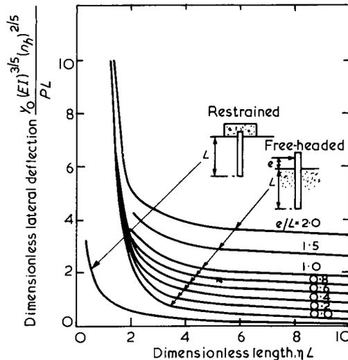
Fig. 6.25 Lateral deflections at ground surface for piles in granular soils, after Broms (1965)
