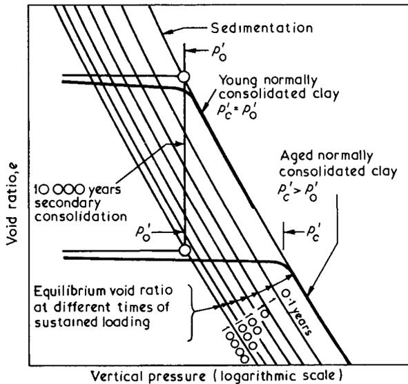
Fig.5.13 Relationships between voids ratio–log effective pressure–time, after Bjerrum (1967)
