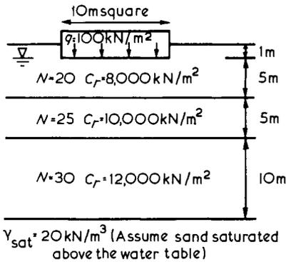
Fig.5.33 Example of settlement calculations
