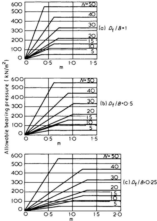
Fig. 5.26 Correlation of allowable bearing pressure to give 25 mm settlement to SPT 'N' value, after Peck, Hanson and Thornburn (1974)
