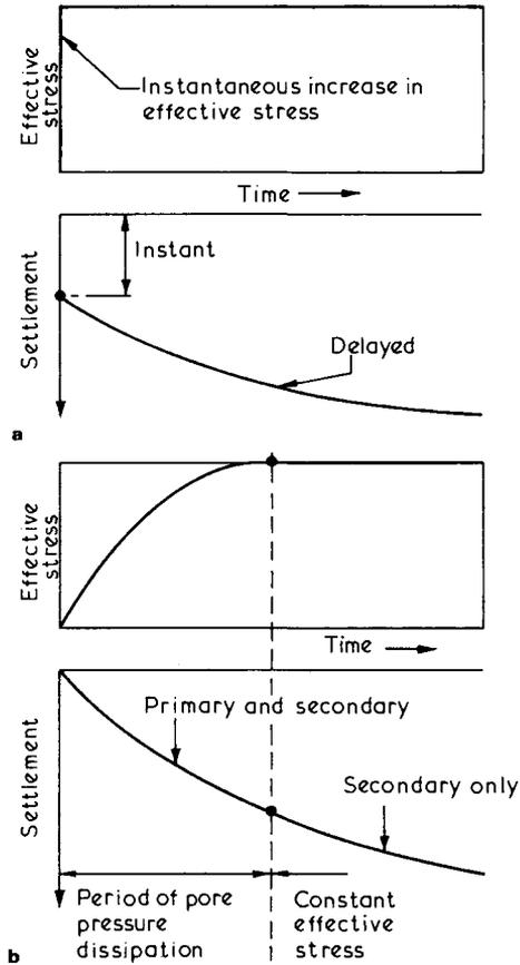
Fig.5.12 Instant and delayed compression, after Bjerrum (1967)
