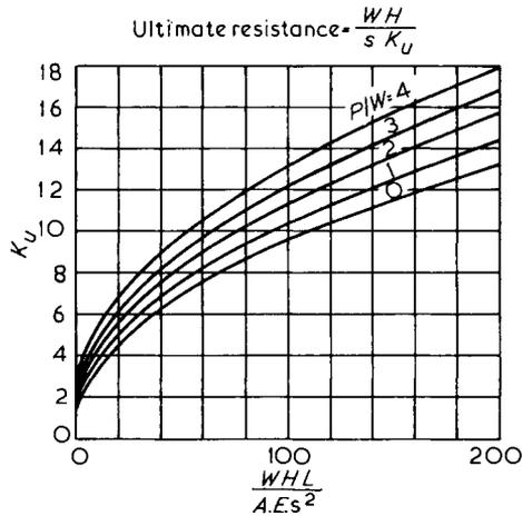
Fig.6.7 Design chart for the Janbu pile driving formula
