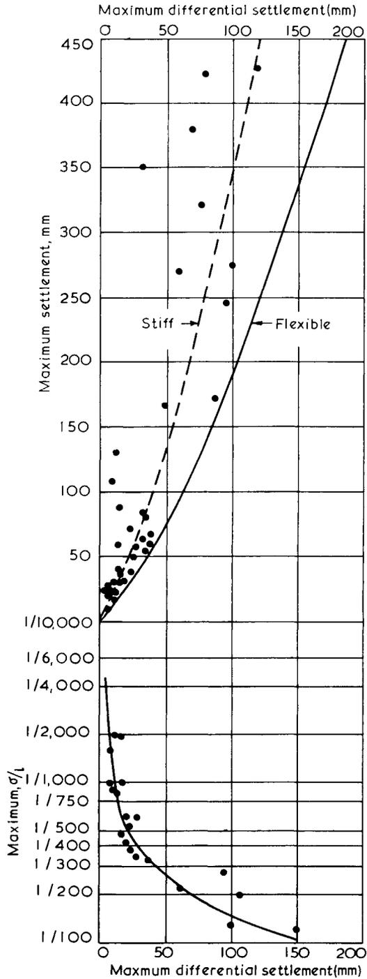
Fig.5.35 Relationship between maximum settlement, maximum differential settlement and maximum angular distortion for clays, after Bjerrum (1963a)
