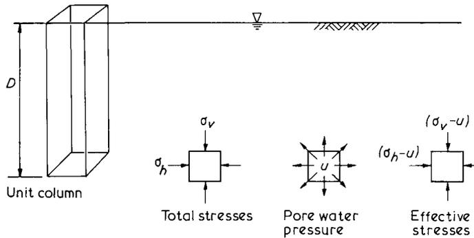
Fig.1.2 'At rest' in situ stresses due to self-weight of soil
