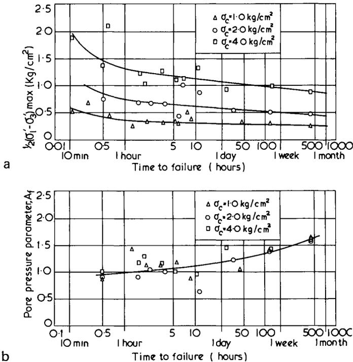
Fig.2.23 The effect of time to failure on undrained shear strength and pore pressure generation, after Bjerrum, Simons and Torblaa (1958); (a) undrained shear strength plotted against time to failure; (b) pore pressure parameter  $A_v$  plotted against time to failure
