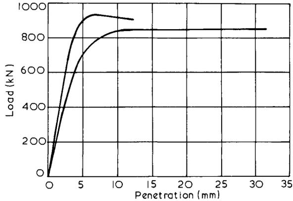
Fig.6.27 Load settlement curve for a friction pile
