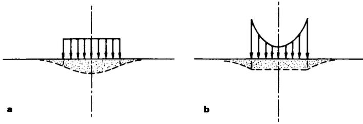
Fig.3.2 Settlements and contact stresses for uniformly loaded circular areas resting on a deep wide homogeneous isotropic elastic solid. (a) flexible footings; (b) rigid footings
