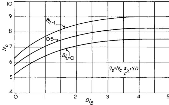
Fig.4.4 Bearing capacity factor,  $N_c$ , for undrained analysis, after Skempton (1951)
