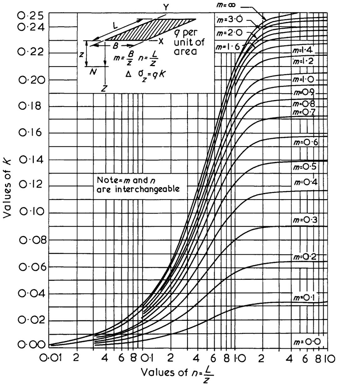
Fig.3.4 Influence coefficients for the increase in vertical stress under the corner of a uniformly loaded flexible rectangular footing, after Fadum (1948)
