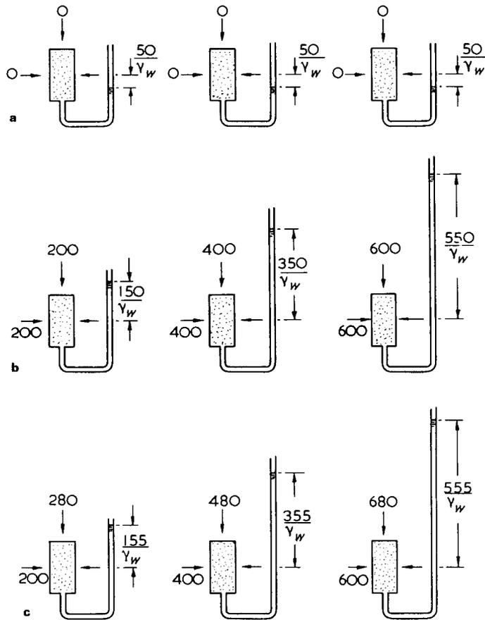
Fig.2.8 Stress diagrams for the undrained test. (a) total stresses and pore pressures after removal from ground; (b) application of cell pressure, undrained; (c) application of axial load to failure, undrained
