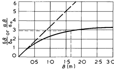
Fig. 5.32 Relationship between settlement ratio and foundation width, after Alpan (1964)
