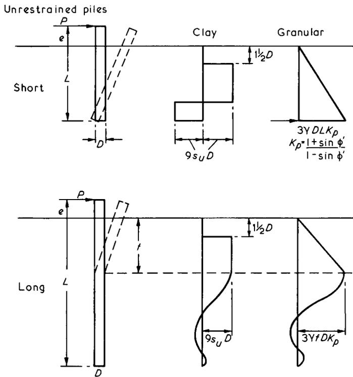
Fig.6.18 Failure mechanisms for short and long unrestrained piles, after Broms (1965)
