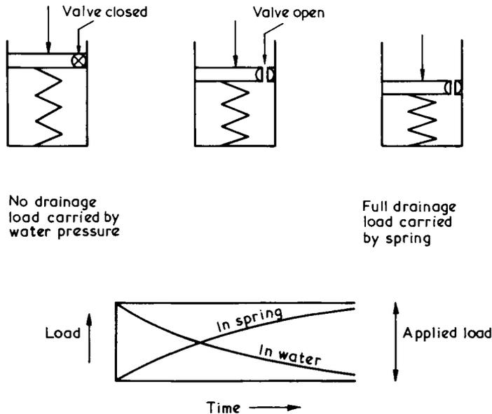
Fig.5.1 Piston and spring analogy
