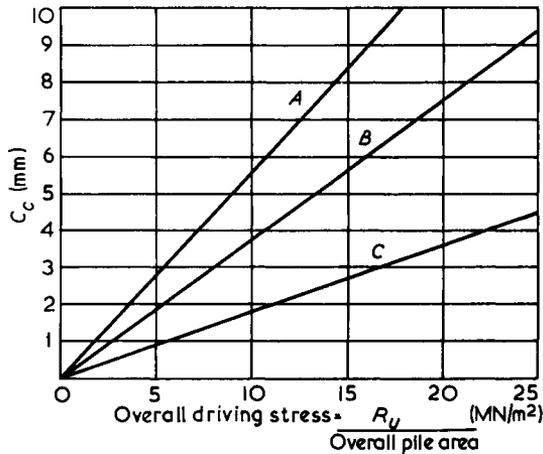
Fig.6.9 Determination of temporary elastic compression  $C_c$ , after BSP Pocket Book (1969)
