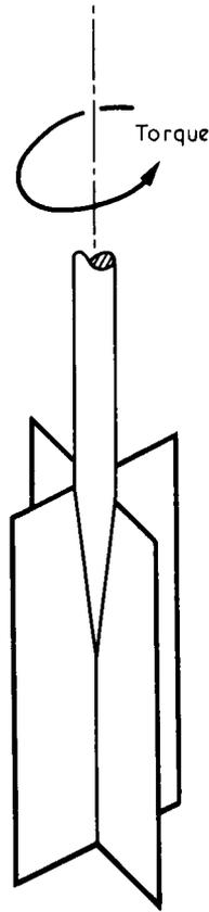
Fig.2.18 Representation of the shear vane
