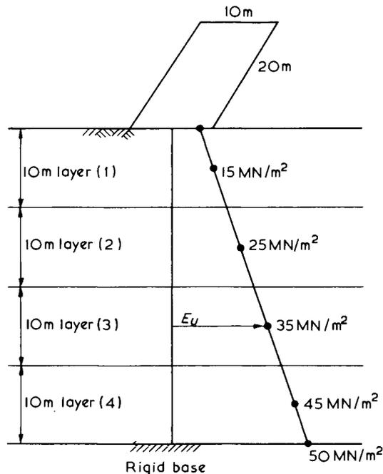
Fig.3.10 Layering of soil profile beneath rectangular area uniformly loaded with intensity 50 kN/m<sup>2</sup>
