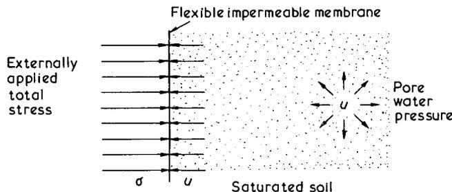
Fig. 1.1 Intuitive soil model demonstrating the nature of effective stress
