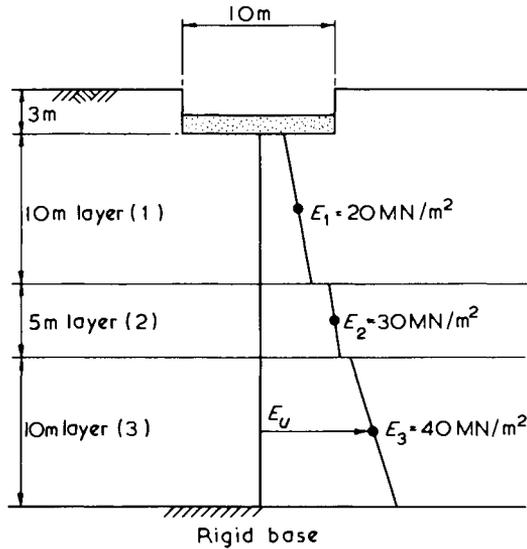
Fig.3.7 Rectangular footing, 10 m × 40 m, uniformly loaded with net intensity 50 kN/m<sup>2</sup>
