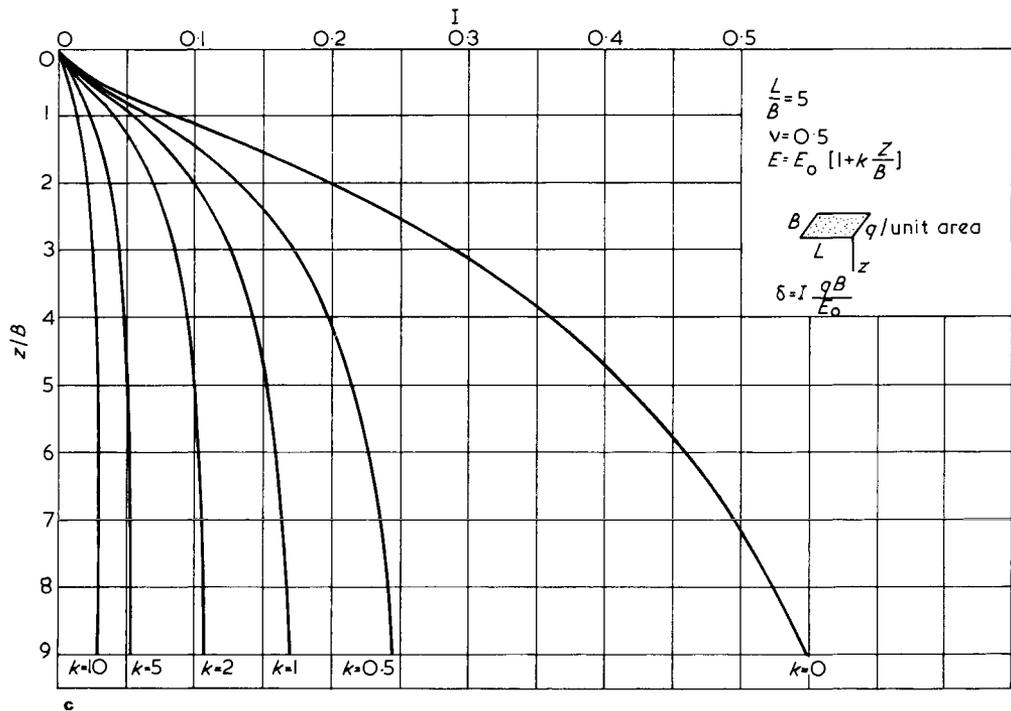
Fig.3.8 Influence coefficients for immediate settlement of the corner of a flexible uniformly loaded rectangle on the surface of a saturated clay with Young's modulus increasing linearly with depth, after Butler (1975); (a) length to breadth ratio  $L/B = 1$ ; (b) length to breadth ratio  $L/B = 2$ ; (c) length to breadth ratio  $L/B = 5$
