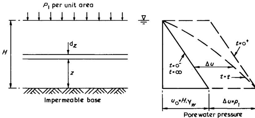
Fig.5.2 Key figure for one-dimensional consolidation
