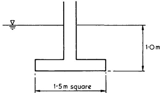
Fig.4.7 Example of short term and long term bearing capacity calculations
