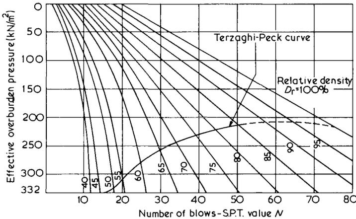
Fig.5.29 Correction factor for effective overburden pressure, after Alpan (1964)
