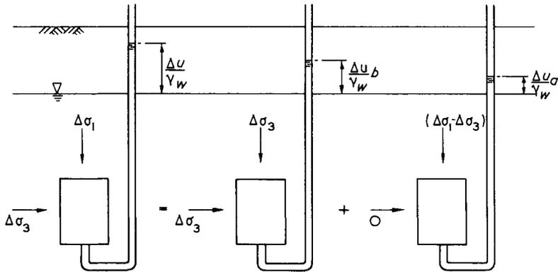
Fig. 1.4 Components of excess pore pressure generated by a loading increment ( $\Delta\sigma_1 > \Delta\sigma_2 = \Delta\sigma_3$ )
