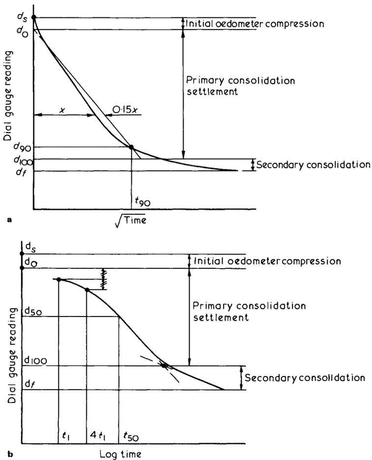
Fig.5.6 Determination of the coefficient of consolidation,  $c_v$ ; (a) square root of time method,  $c_v = T_{90} \cdot H^2/t_{90}$ ,  $H^2/t_{90} = 0.212 H^2/t_{90}$  ( $H$  = sample thickness); (b) logarithm of time method,  $c_v = T_{50} \cdot H^2/t_{50}$ ,  $H^2/t_{50} = 0.0492 H^2/t_{50}$  ( $H$  = sample thickness)
