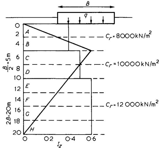
Fig.5.34 Determination of Schmertmann's influence factor
