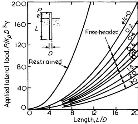
Fig. 6.23 Ultimate lateral resistance for short piles in granular soils, after Broms (1965)
