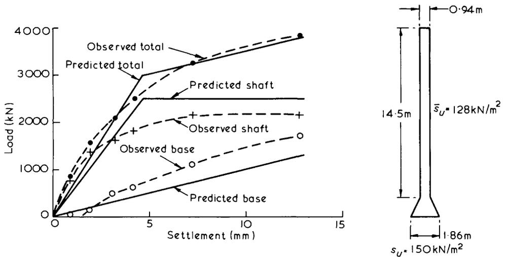
Fig 6.5 Predicted load settlement relationship for a bored pile in London clay, after Burland and Cooke (1974)
