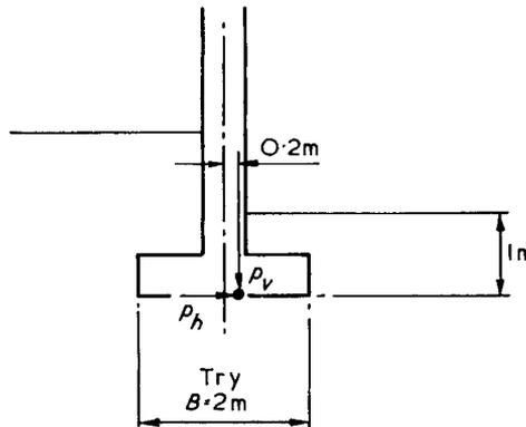
Fig.4.8 Example of bearing capacity calculations for inclined and eccentric loading
