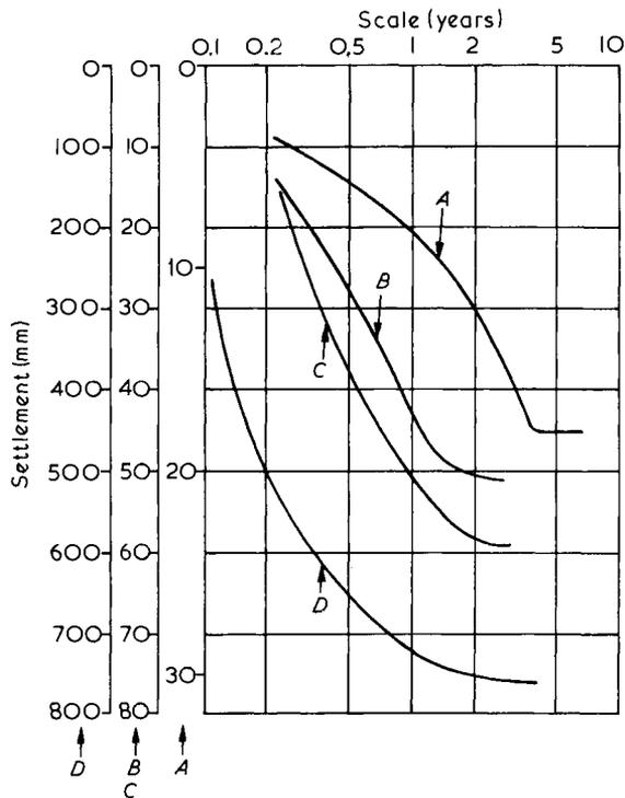
Fig. 5.16 Settlement-log time curves indicating terminating settlement, after Simons (1974).
