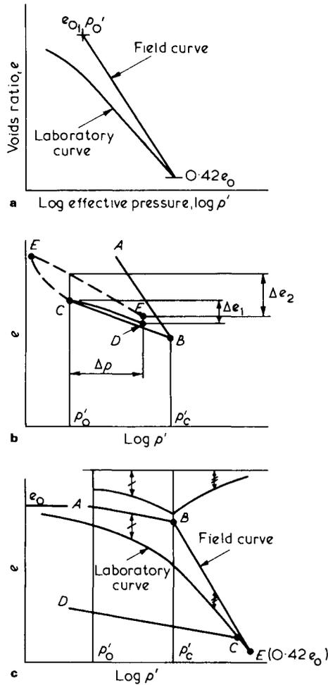
Fig.5.8 Correction of voids ratio--log effective pressure curve for sample disturbance, after Schmertmann (1953)
