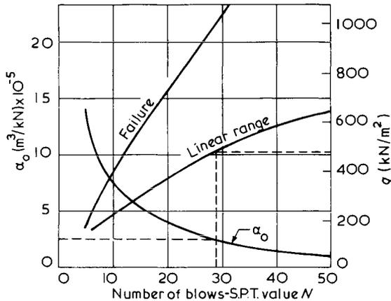
Fig.5.30 Determination of  $\alpha_o$ , for low SPT ' $N$ ' values, after Alpan (1964)
