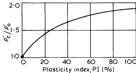
Fig.5.14 Relationship between  $p'_c/p'_o$  and plasticity index, after Bjerrum (1967)
