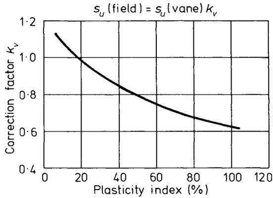
Fig. 2.22 Vane strength correction factor for soft clays (after Bjerrum, 1973)
