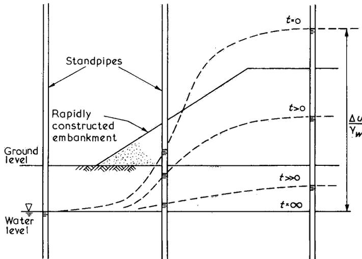
Fig. 1.3 Pore pressure response of a saturated clay to rapid local loading
