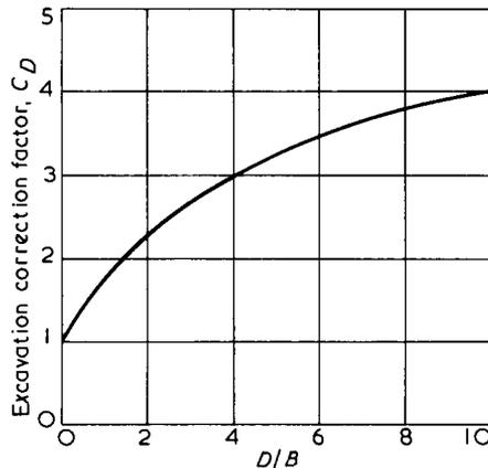
Fig.5.27 Excavation correction factor,  $C_D$ , after Parry (1971)
