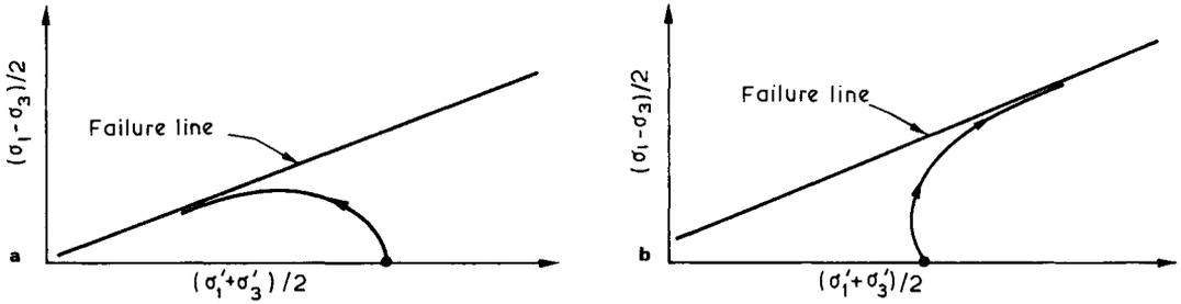
Fig.2.15 Typical effective stress paths for undrained triaxial compression tests on (a) loose sand/soft clay; (b) dense sand/stiff clay
