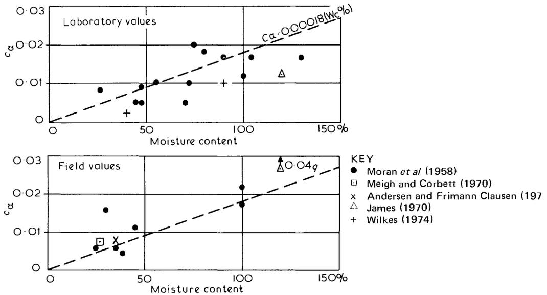
Fig. 5.15 Values of  $c_\alpha$ , the coefficient of secondary consolidation plotted against moisture content, after Simons (1974)
