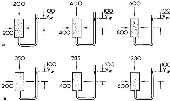
Fig. 2.11 Stress diagrams for drained test. (a) application of cell pressure. Drainage to back pressure of  $100 \text{ kN/m}^2$ ; (b) application of axial load to failure. Drainage to back pressure of  $100 \text{ kN/m}^2$
