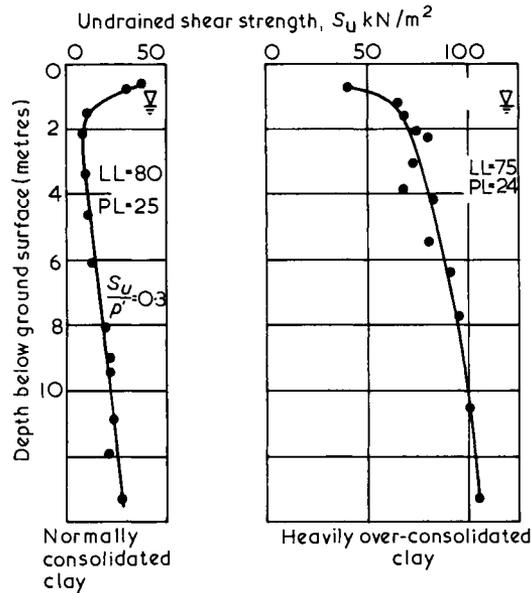
Fig.2.16 Typical variations of undrained shear strength with depth, after Bishop and Henkel (1962)
