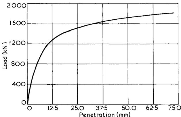
Fig.6.28 Load settlement curve for an end bearing pile
