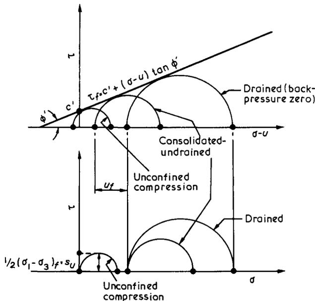
Fig.2.7 Correlation between axial compression tests
