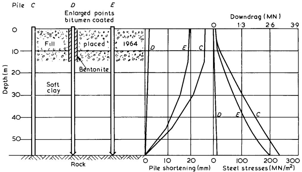
Fig. 6.14 Examples of the effects of negative skin friction on the behaviour of piles, after Bjerrum, Johannessen and Eide (1969)
