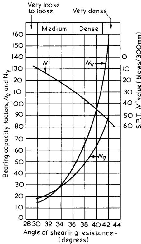
Fig.5.23 Relationship between SPT 'N' value and  $\phi'$ ,  $N_q$  and  $N_\gamma$ , after Peck, Hanson and Thornburn (1974)
