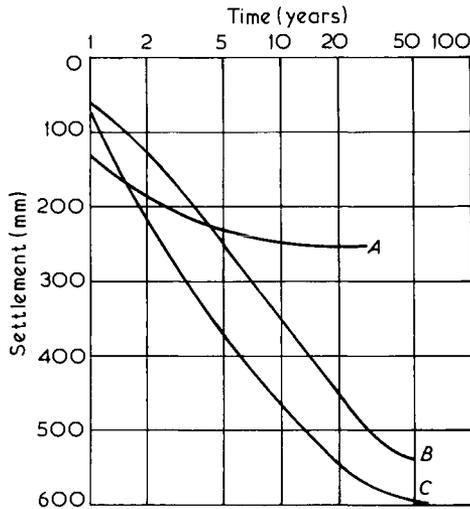
Fig.5.18 Settlement–log time curves for three structures in Chicago, after Skempton, Peck and MacDonald (1955)
