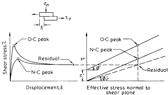
Fig.2.5 Relation of peak shear strengths to residual shear strengths as measured in the direct shear box for over-consolidated (O-C) and normally-consolidated (N-C) clays
