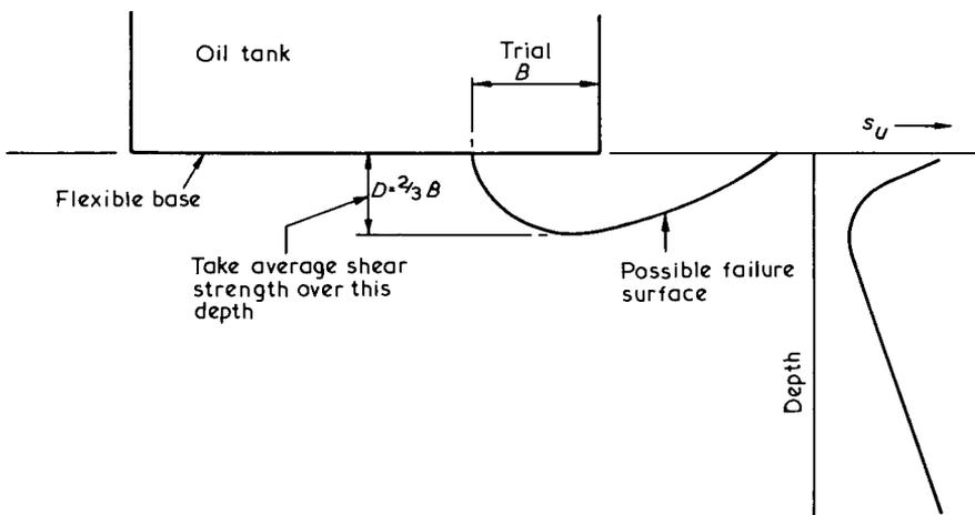
Fig.4.6 Bearing capacity calculations for an oil tank, after Bjerrum and Øverland (1957)
