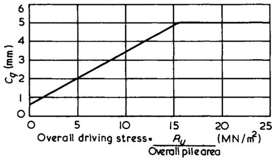
Fig. 6.13 Determination of temporary elastic compression  $C_q$ , after BSP Pocket Book (1969)
