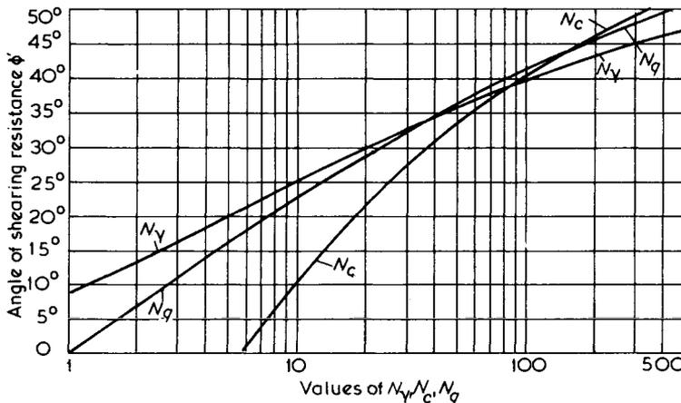
Fig.4.2 Bearing capacity factors,  $N_c$ ,  $N_q$ ,  $N_\gamma$ , after Terzaghi (1943)
