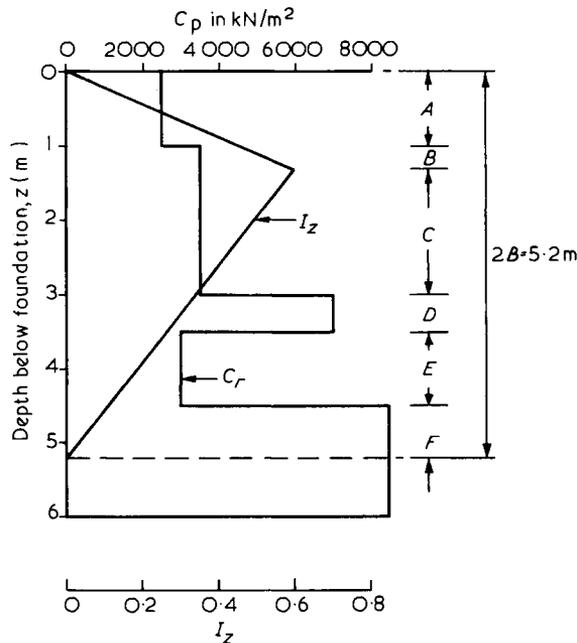
Fig.5.22 Example of settlement calculation following Schmertmann (1970)
