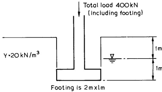
Fig.4.1 Example of gross and net pressures
