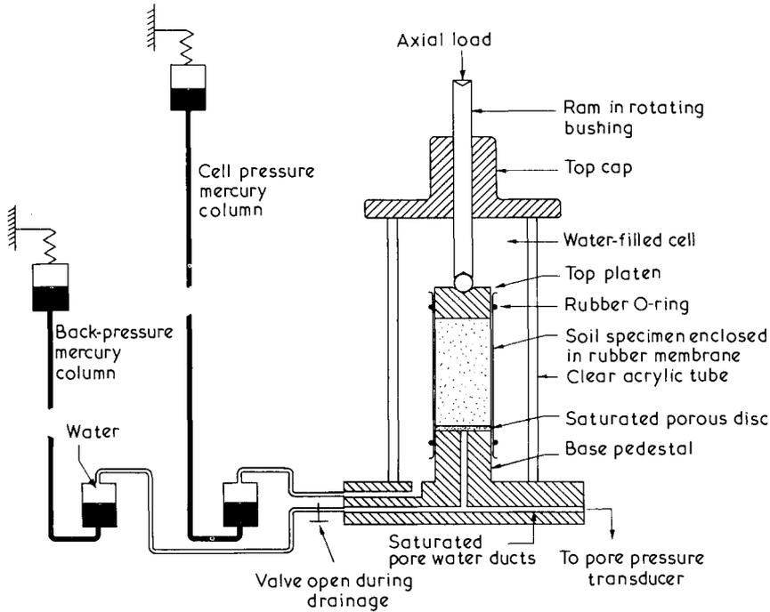
Fig.2.6 Typical set-up for triaxial compression tests
