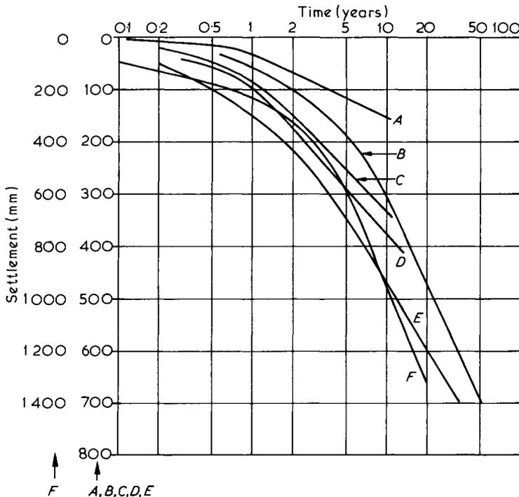
Fig. 5.17 Settlement-log time curves indicating non-terminating settlement, after Simons (1974)
