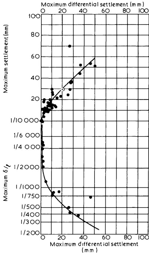
Fig.5.36 Relationship between maximum settlement, maximum differential settlement and maximum angular distortion for sands, after Bjerrum (1963a)
