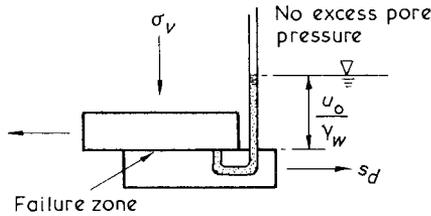
Fig.2.4 Stresses at drained failure in the direct shear box
