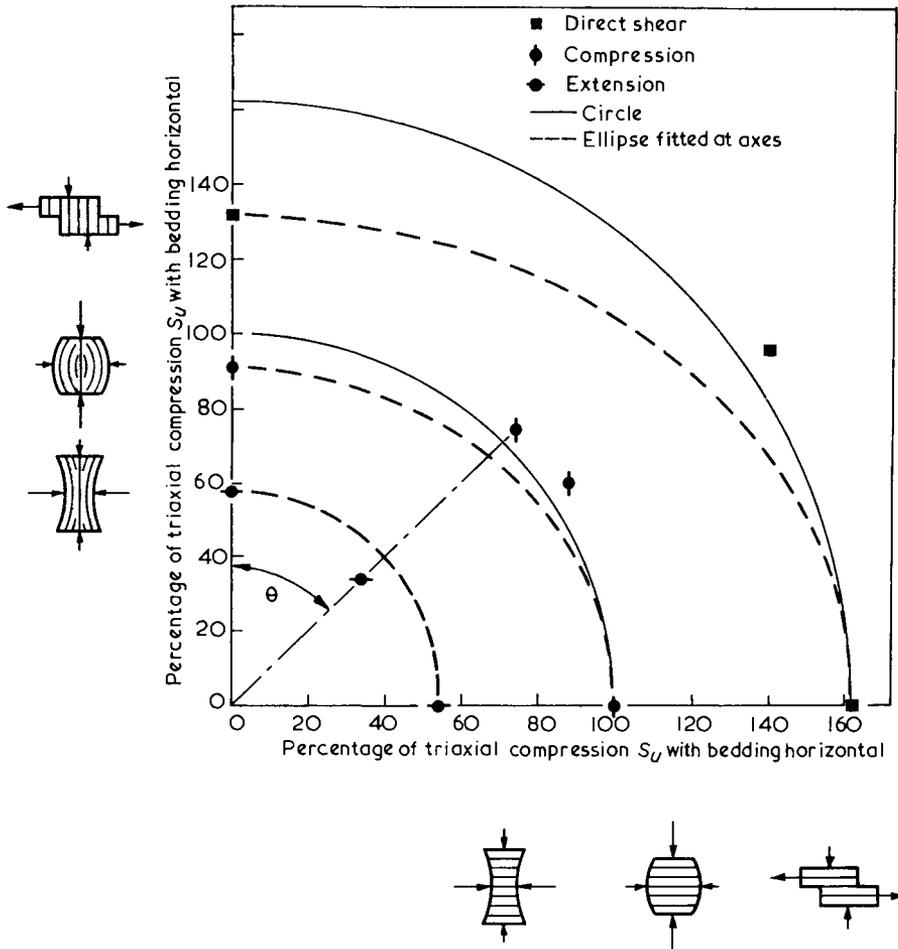
Fig.2.21 Polar diagram showing the variation in undrained shear strength with test type and specimen orientation for a soft clay from Kings Lynn, Norfolk, after Madhloom (1974)
