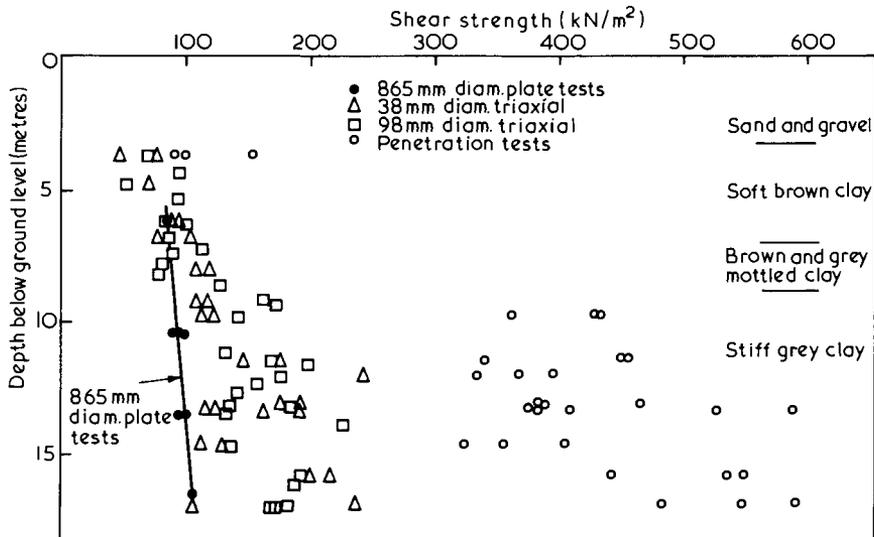
Fig.2.19 Comparison of undrained shear strengths estimated from 865 mm diameter plate tests and triaxial tests on 38 mm and 98 mm diameter specimens in London clay at Chelsea, after Marsland (1971(a))
