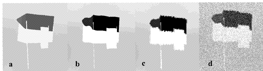
Fig. 9. Complete process of simulating the sonar image: a) an image obtained by ray-tracing, c) simulating the changing speed of a ship, d) simulating the changing course and side tilt, d) resulting image with noise added
