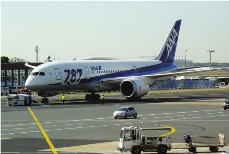
Fig. 1 Boeing 787 with composite airframe
