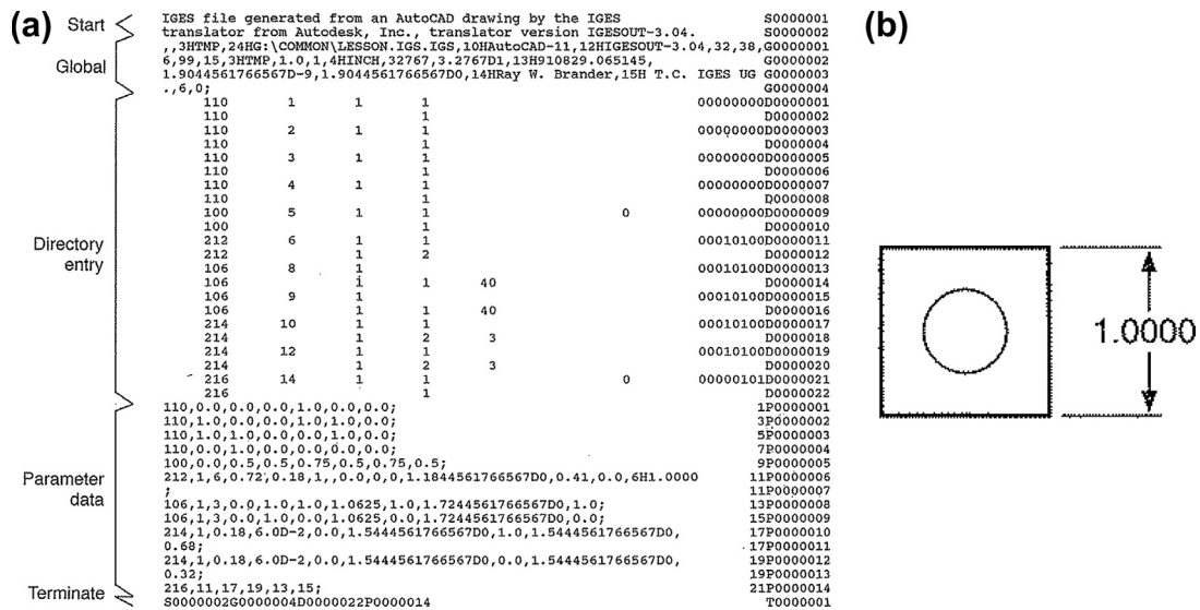
FIGURE A.1 Anatomy of a Sample IGES File. (a) IGES File with Sections Labeled, and (b) Equivalent Graphics (Stokes, 1995).
