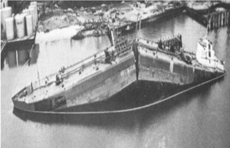
Fig. 2.1 An oil tanker that fractured in a brittle manner by crack propagation around its girth (Callister 1997, 4e) (This material is reproduced with permission of John Wiley & Sons, Inc.)
