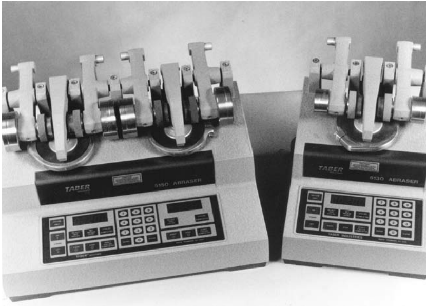
Fig. 13 Abrasion tester. (Courtesy Taber Industries)
