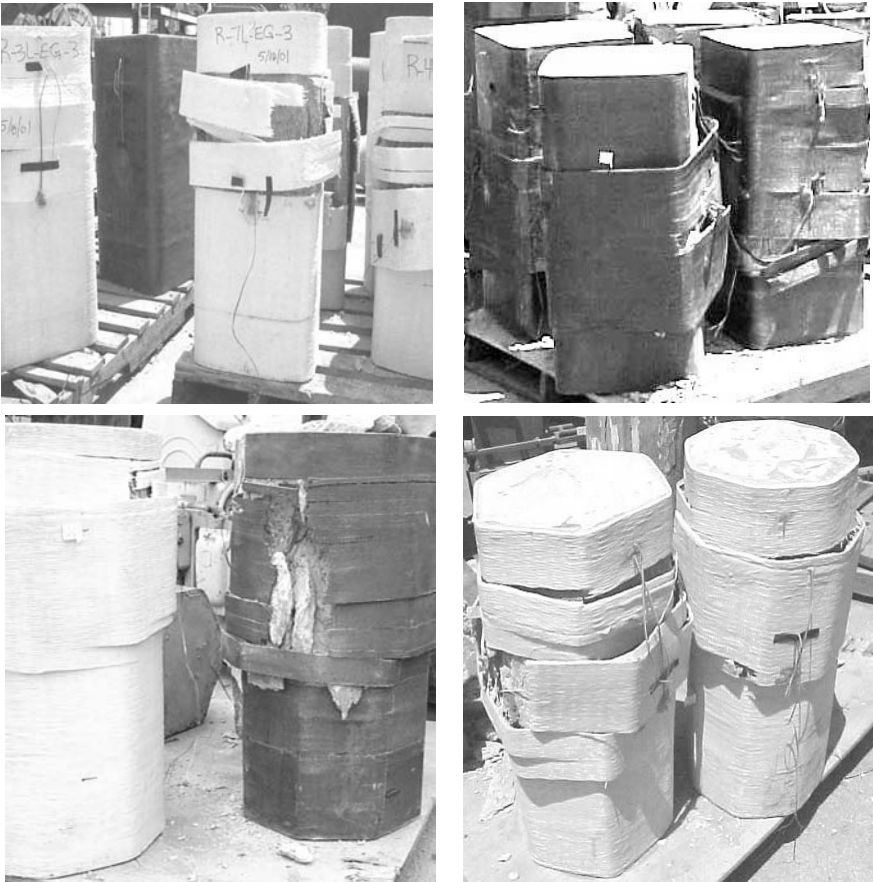
Fig. 30 Samples of reinforced and unreinforced column specimens (Youssef, 2001).
