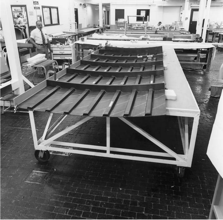
Fig. 4 Co-cured fuselage skin panel with integral stiffeners and frames.
