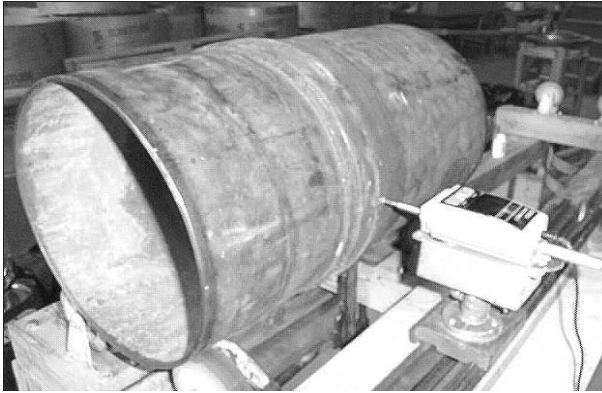
Fig. 13 Seismic strengthening of steel pipe joints using polymer composites. [Courtesy of Professor O'Rourke, Cornell University (Tutuncu, 2001)]
