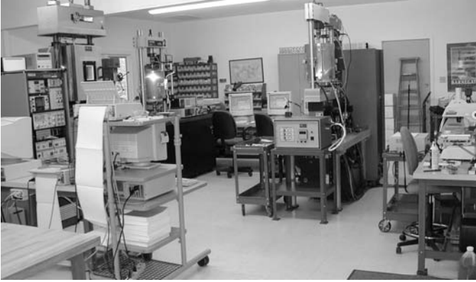
Fig. 1 Typical material test lab containing numerous servohydraulic test frames. (Courtesy of Fracture Technology Associates)
