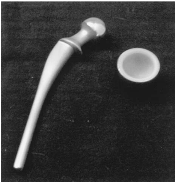
Fig. 2 Example of total hip implant, including femoral and acetabular components.
