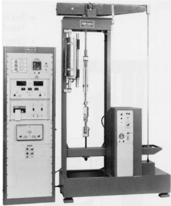
Fig. 5 Typical test setup for tensile creep testing. (Courtesy Applied Test Systems Inc.)
