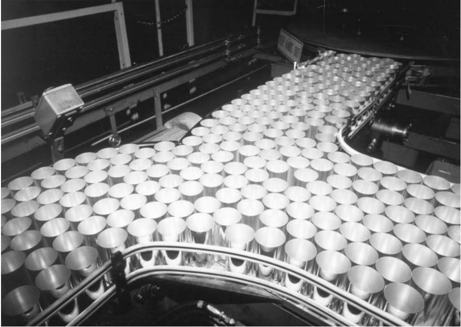
Fig. 7 Bodies of most beverage cans are alloy 3004, the ends are 5182, making it the largest volume alloy combination in the industry.
