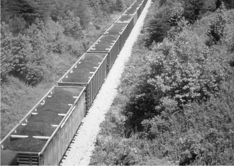
Fig. 10 Alloy 5454 has been widely used for railcar body construction where heavy loads, such as coal, and potentially high temperatures, may be involved.
