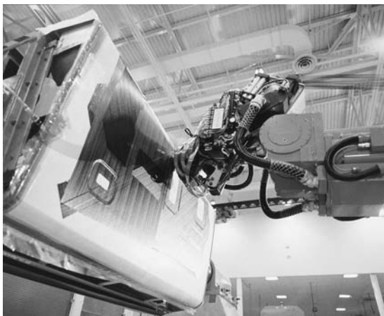
Fig. 19 Large tape laying machine. Both the tape laying head and the tooling are manipulated to form a large aircraft fuselage component. (Photograph of the Viper tape layer courtesy of Cincinnati Machine Co., OH)
