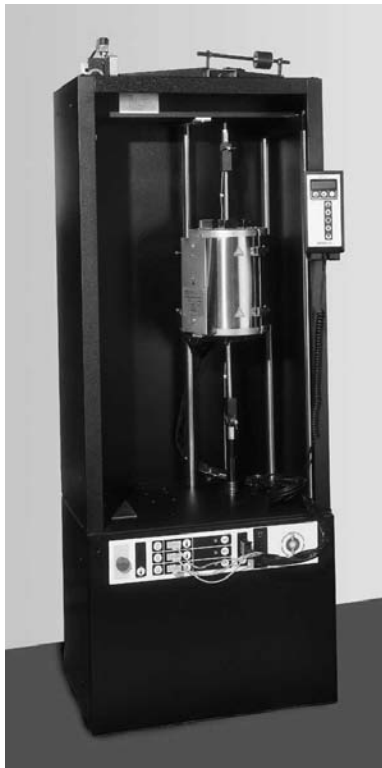
Fig. 7 Loading frame to apply static (or extremely slow cyclic) load conditions. (Courtesy of the Instron Corporation)
