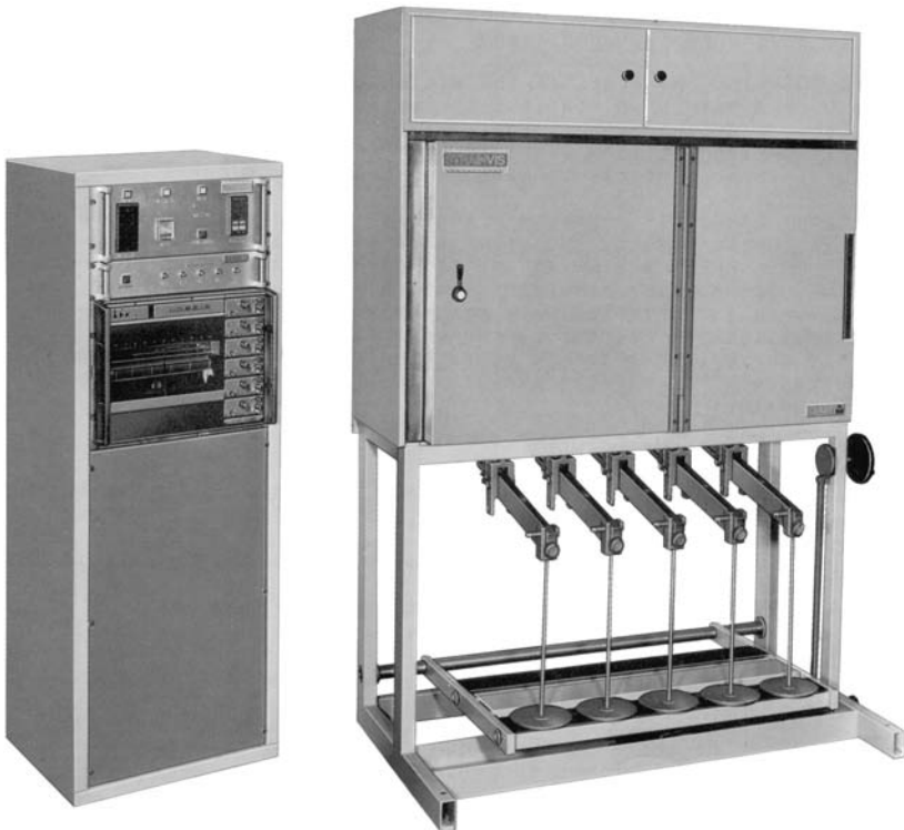
Fig. 6 Flexural creep testing. (Courtesy Ceast U.S.A. Inc.)
