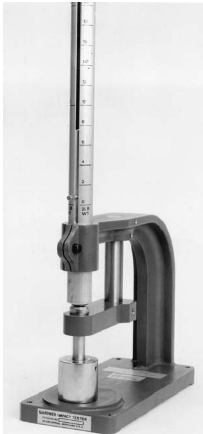
Fig. 9 Drop impact tester. (Courtesy Byk-Gardner USA)
