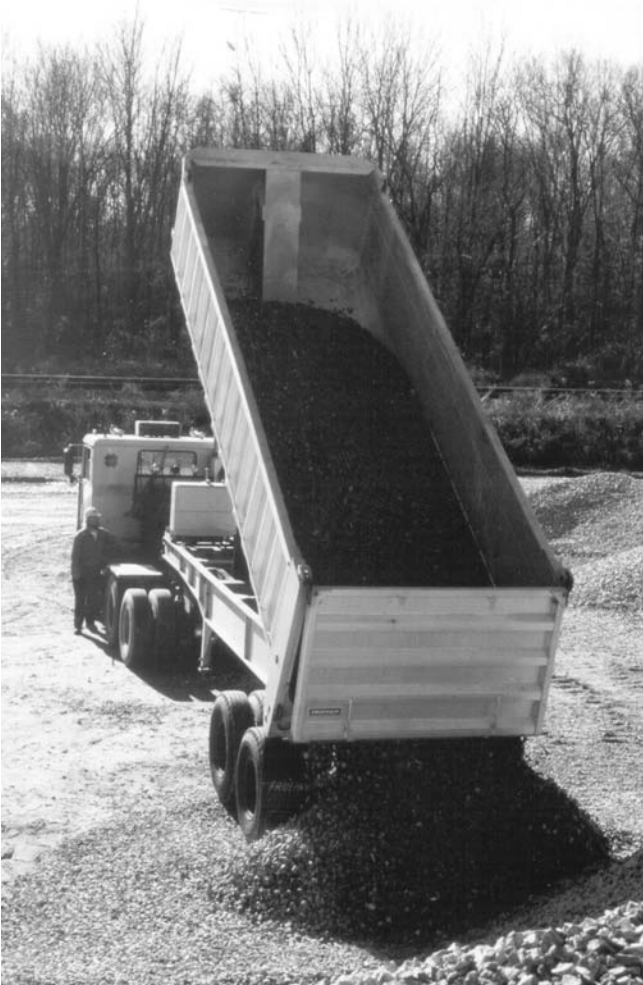
Fig. 4 Heavy dump and tank trucks and trailer trucks employ high-strength 2xxx or 6xxx extrusions for their structural members and tough 5xxx alloy sheet and plate for their load-carrying components.
