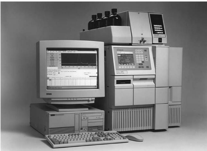
Fig. 4 GPC equipment. (Courtesy Waters Corporation)
