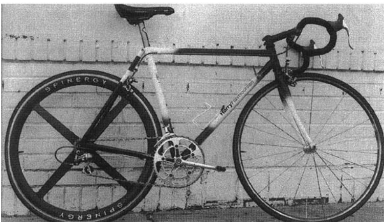
Fig. 10 Road bicycle made by Harry Havnoonian with a mix of materials using adhesive bonding for joints, investment-cast stainless steel lugs, Ti-3Al-2.5V head tube, SiC-fiber-reinforced aluminum alloy front triangle, CRFP rear triangle, and CFRP rear wheel.
