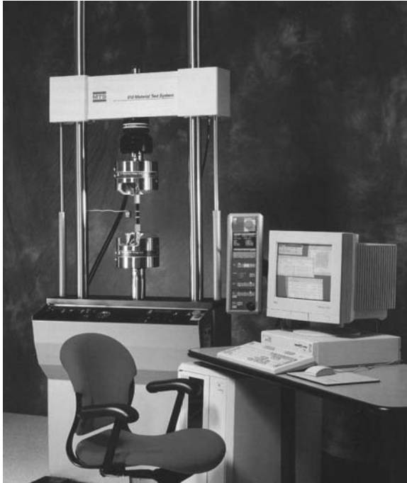
Fig. 2 Servohydraulic test frame and digital controller. (Courtesy of MTS Corporation)
