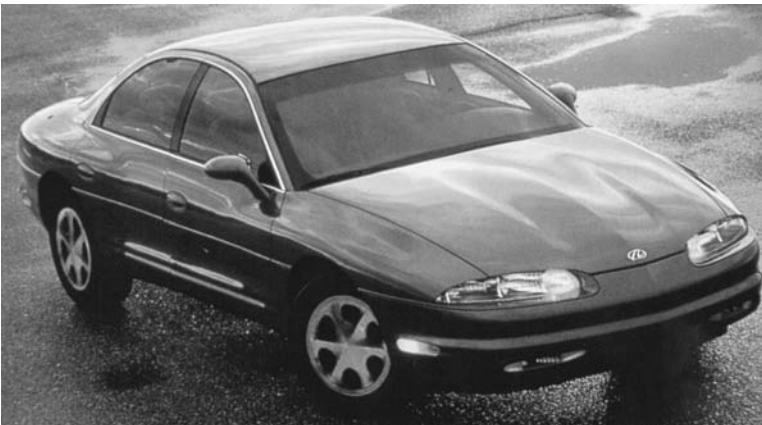
Fig. 13 Automotive structures are likely to employ increasing amounts of 5754-O formed sheet for parts such as internal door stiffeners or (a) the entire body in white; (b) external body panels are more likely to be higher strength 6111-T4.
