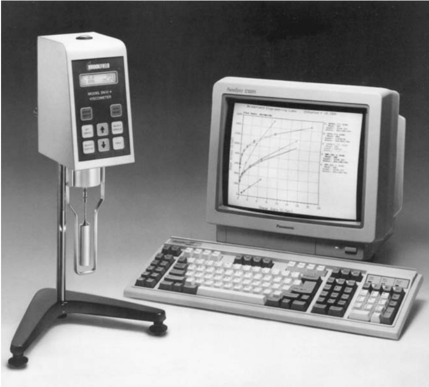
Fig. 3 Digital programmable viscometer. (Courtesy Brookfield Engineering Laboratories)
