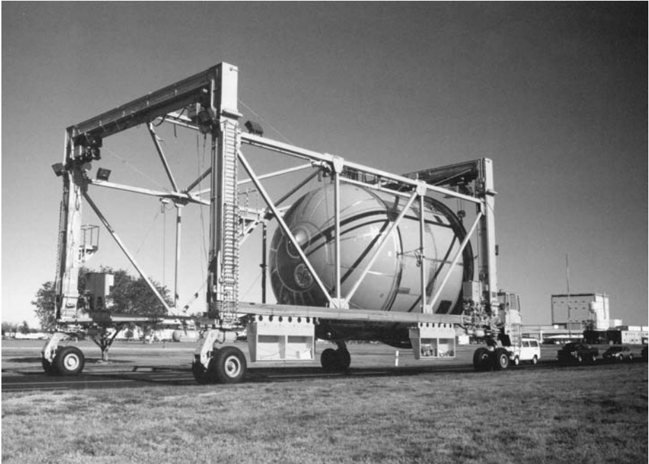
Fig. 5 Fuel tanks and booster rockets such as those of the Space Shuttle are 2xxx alloys, originally 2219 and 2419, now Al–Li “Weldalite” alloy 2195.
