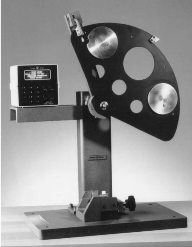
Fig. 8 Pendulum impact tester. (Courtesy Tinius Olsen Company)
