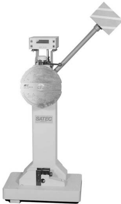
Fig. 9 Example of a pendulum impact machine. (Courtesy of the Instron Corporation)
