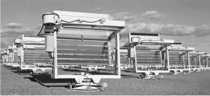
Fig. 23 Accelerated outdoor weathering testers. (Courtesy Atlas Electric Devices Company)
