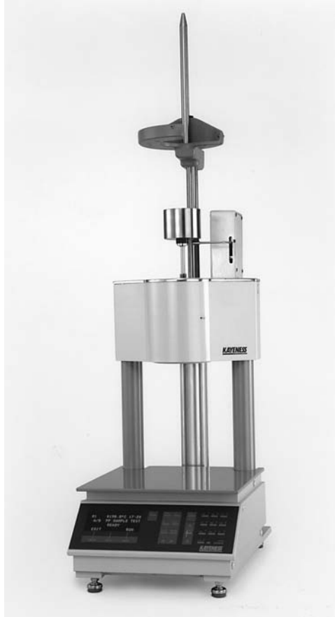
Fig. 2 Melt indexer. (Courtesy Dynisco-Kayeness Polymer Test Systems)
