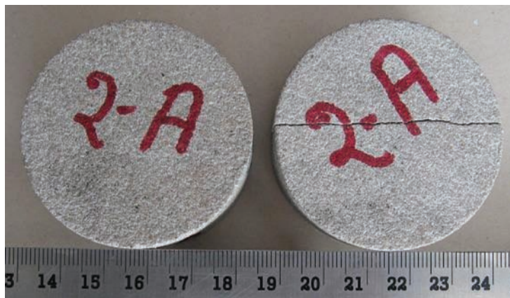
Figure 9. Typical virgin and tested rock samples (under 0.01 GPa/s loading)
