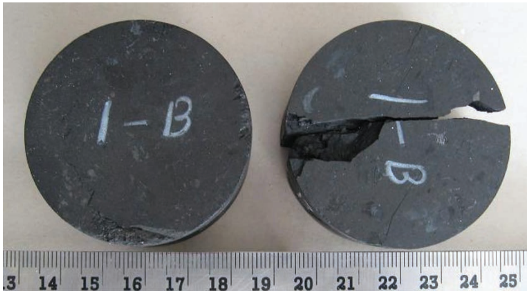
Figure 5. Typical virgin and tested coal samples (under 237 GPa/s loading rate)
