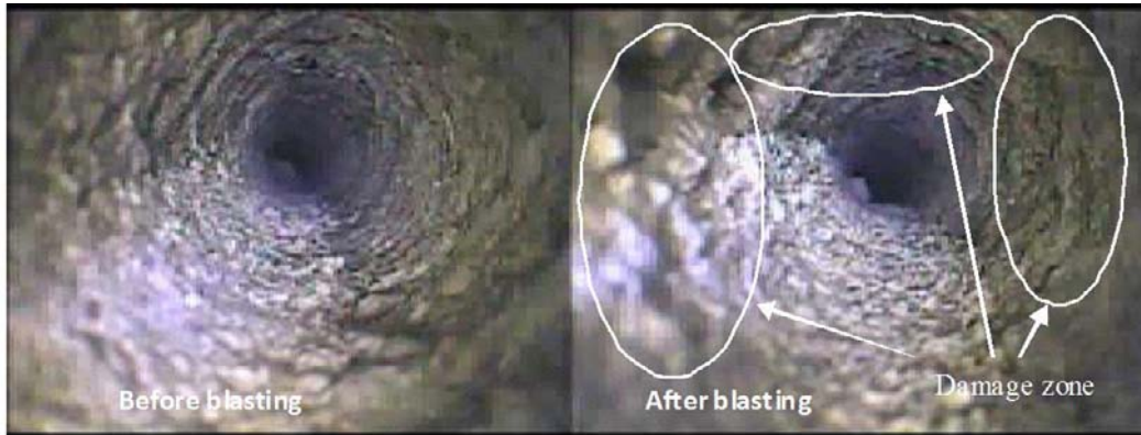
Figure 15. Images of intact and disturbed rock mass with obtuse joint orientations captured by borehole camera
