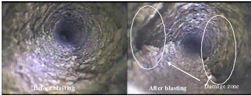
Figure 19. Borehole camera images of intact and disturbed rock mass with obtuse angle joint orientations
