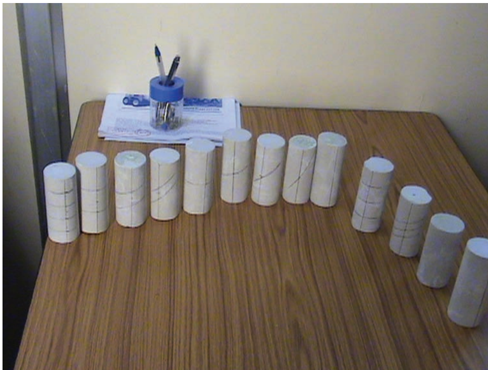
Figure 4. POP-cement mix specimens with marks representing the position of joints
