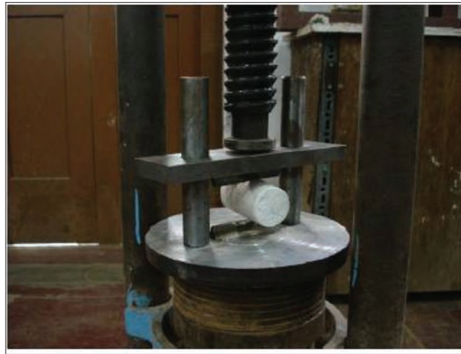
Figure 1. Creating joints in the POP specimen
