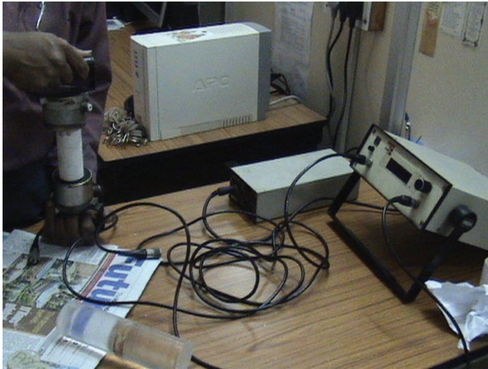
Figures 5. Measurement of V_p of POP specimen
