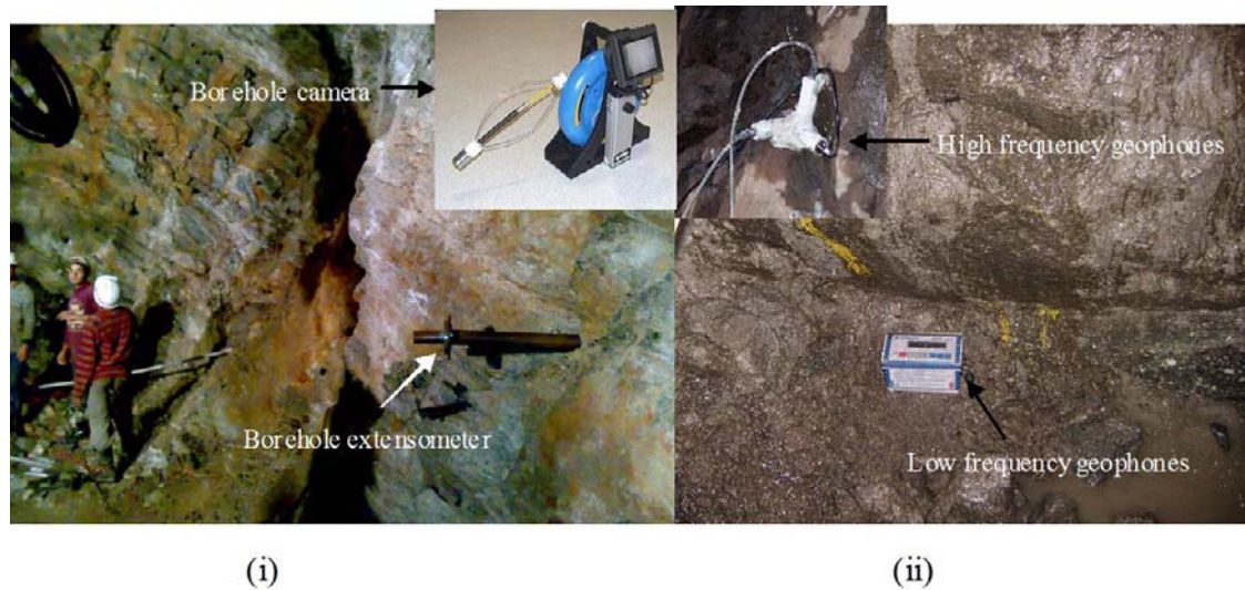
Figure 7. The installation of (i) borehole extensometer and (ii) geophones
