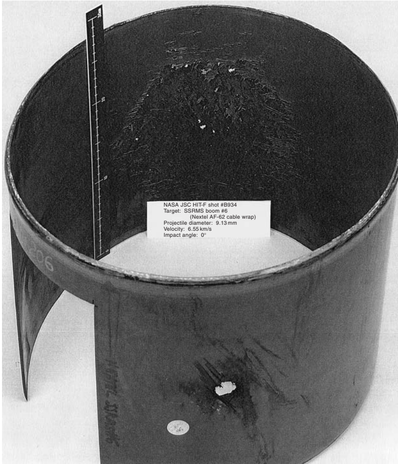
9.11 Photograph of crater, front face spallation and debris plume damage to rear wall due to hypervelocity impact on graphite/PEEK cylinder.
