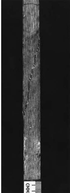
5.25 Compression failure with a kink shear band in a 14 mm thick S-glass/phenolic CAI panel.
