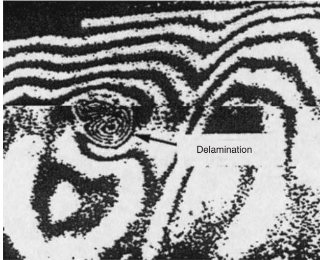
2.25 Shearographic fringe pattern of a filament wound composite cylinder containing a delamination. (After Hung 78 .)
