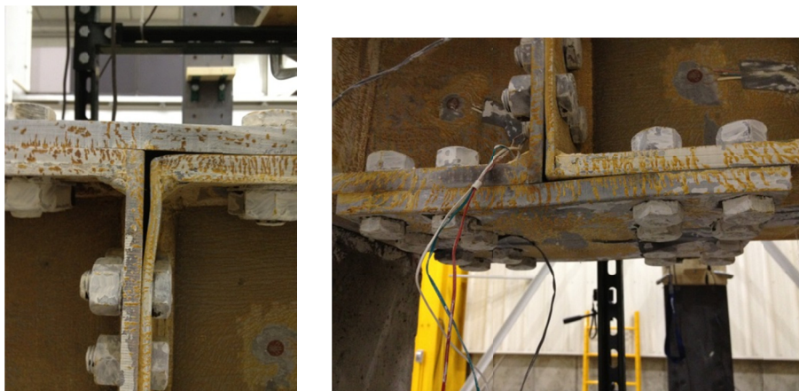
Fig. 11 – Damage noticed in plate components at the end of Test 2
