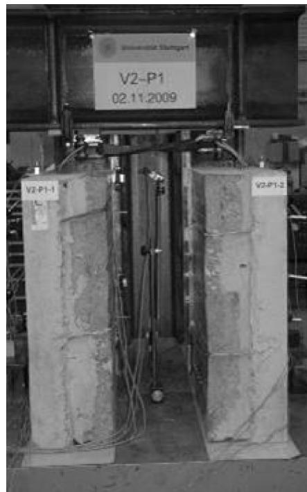
Fig. 12 – Push-out test at Stuttgart
