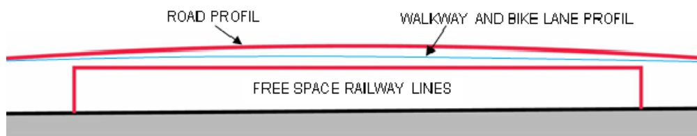
Fig. 8 - Profile constraints and shape of the bridge
