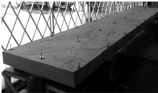
Figure 5. B2 specimen in situ with accelerometers
