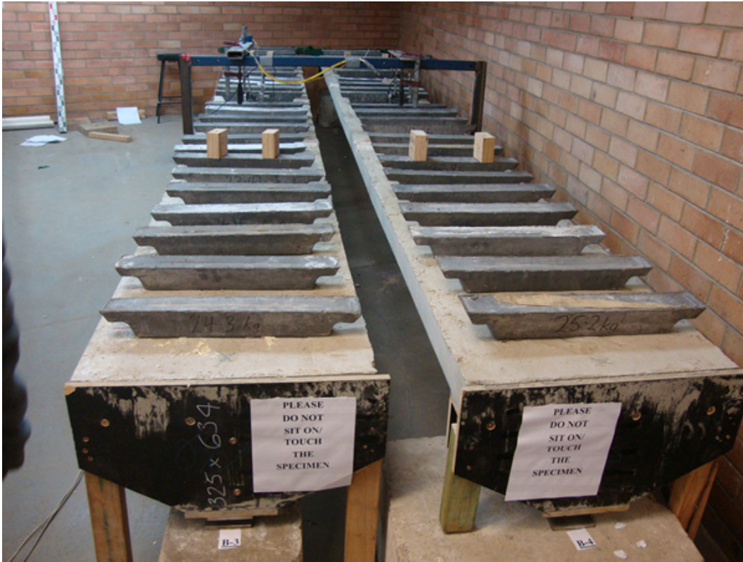
Figure 5. Beams under quasi-permanent loads (lead bars).
