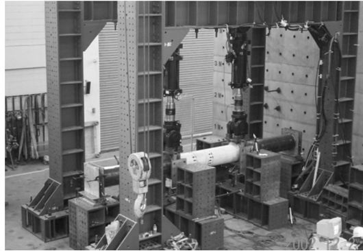
Figure 2. 4-Points bending test on CFT.
