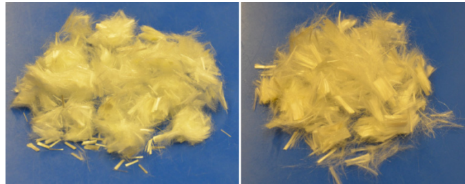
Figure 1. PVA fibres; 6 mm fibres (left) 12 mm fibres (right).
