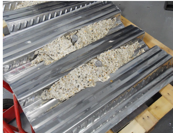
Figure 11. Failed specimen - decking
