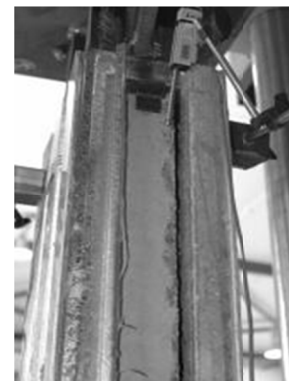
Figure 11. Linear potentiometer dropped
