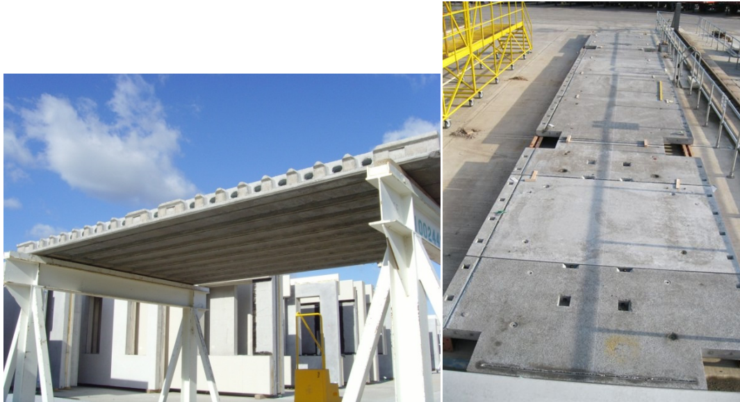
Fig. 13 - Manufacturing trials demonstrating quality of finish (left) and connectivity (right)
