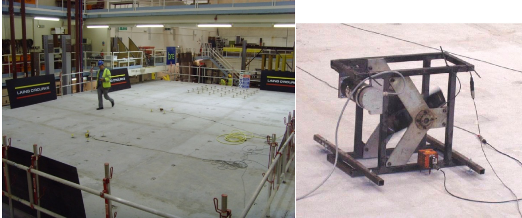
Fig. 11 - Dynamic testing under 'pacing' load (left), rotary shaker (right)
