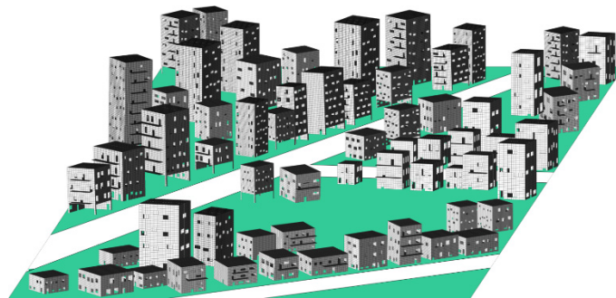
Figure 3. A regional portfolio of 3D FE-models for masonry buildings simulated with the SBP-Tool. This can be combined with any seismic input, e.g. wave propagation models
