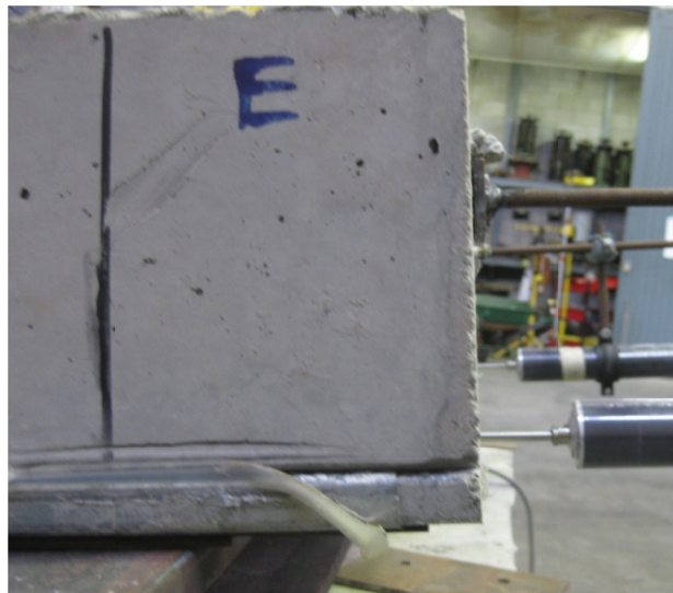
Figure 12. Final end slip at eastern end support of Slab S2 ( S = 25 mm).
