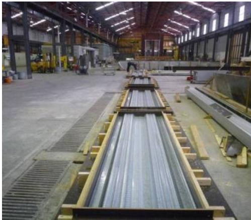
Figure 7: Formwork and slab immediately after casting.
