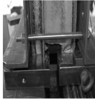
Figure 9. Local buckling of the sheeting
