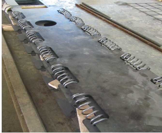
Figure 13. Web plate with the helically reinforced connector for use in the slab rib
