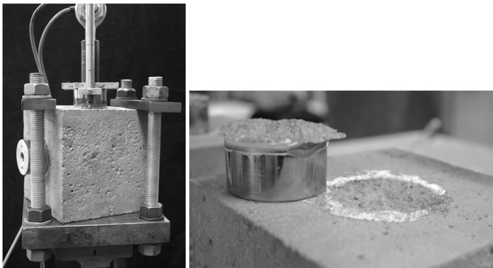
Figure 14. typical test set-up and results of the unaged Pull-Out tests
