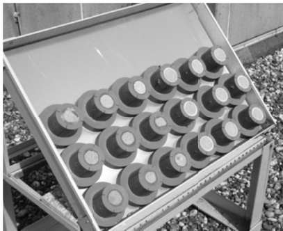
Figure 6. natural ageing of the specimens
