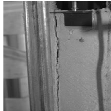
Figure 7. Initiation of slip from one side
