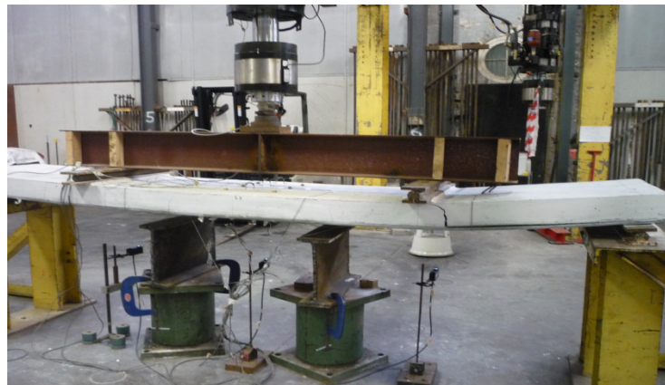
Figure 13: Typical slab failure.
