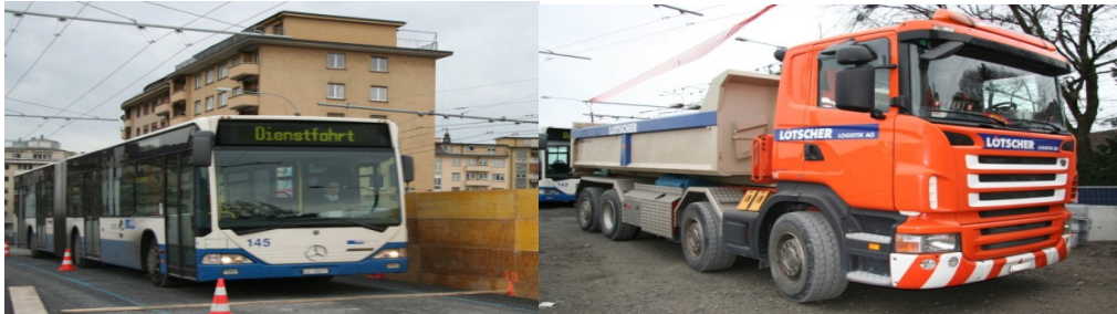
Fig. 23 - Two of the vehicles used for the dynamic load tests. Tests with crossing a 25 and a 50 mm-plank were also performed
