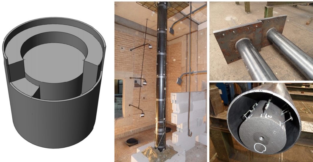
Figure 1. Concrete-filled CHS column with steel core.
