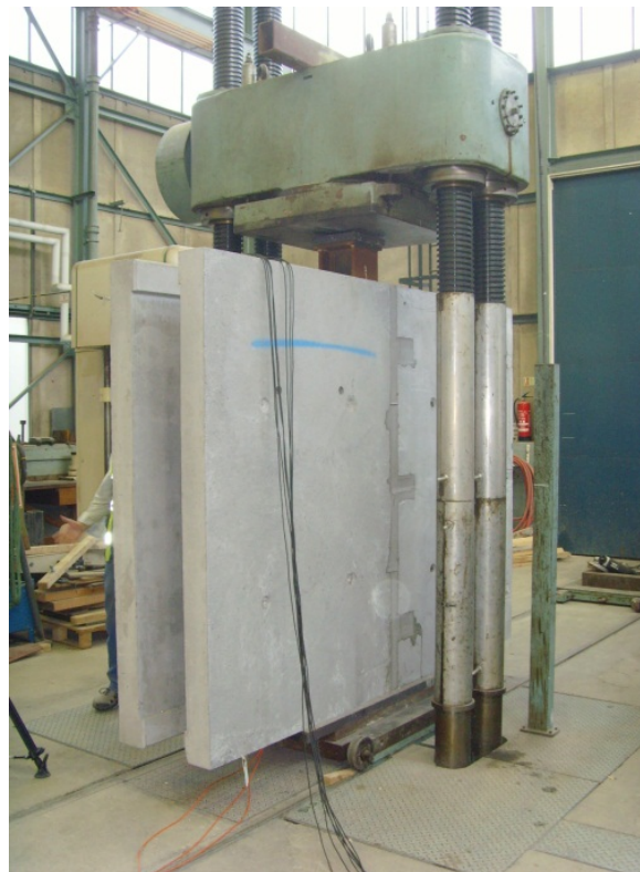
Fig. 4 - Photo of connection shear strength test at BRE
