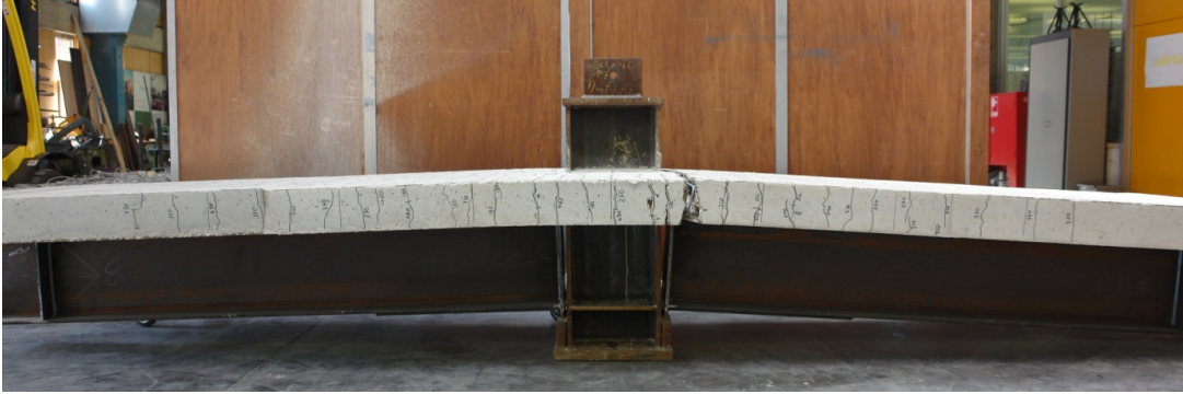
Fig. 11 – Side elevation of failed test specimen (Test A-5)
