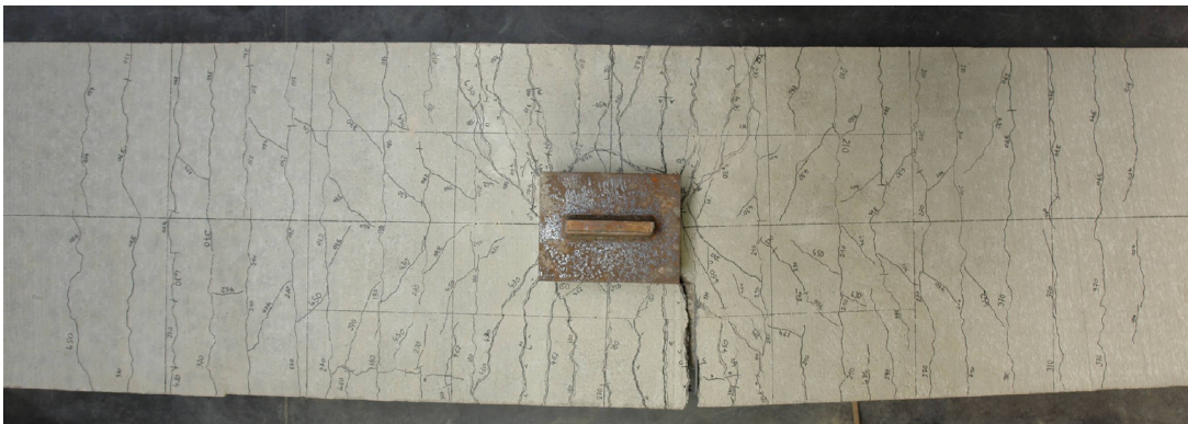
Fig. 12 – Top view on failed test specimen (Test A-5)
