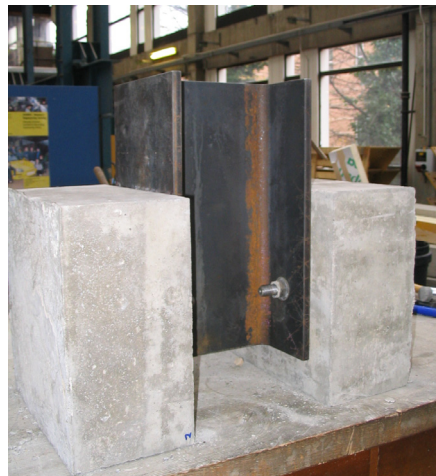
Figure 2. Push test specimen
