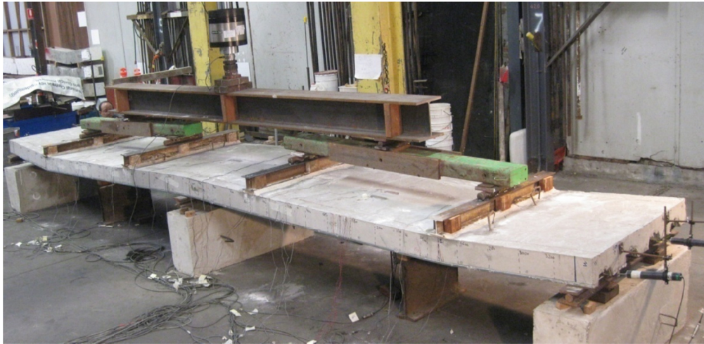
Figure 13. Final deflected shape of slab S1.
