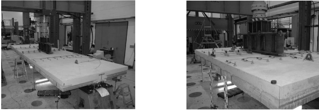
Fig. 4 – Bending (left photo) and shear (right photo) beam tests at Stuttgart
