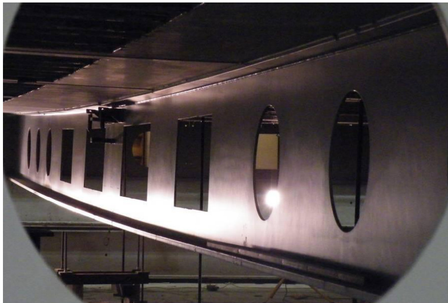
Fig. 10 - Beam deflection under 'ultimate' design load
