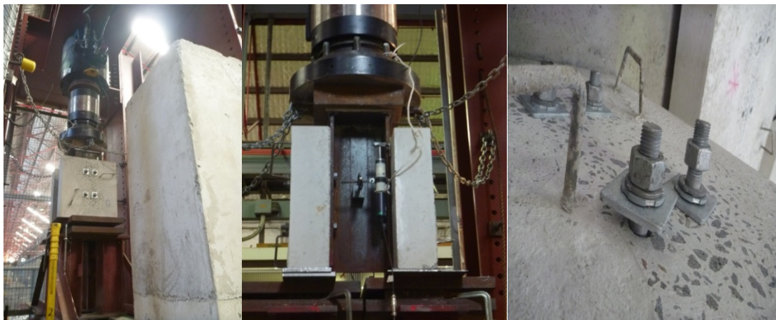
Figure. 8. Test set up and failure mode for push tests 008 and 009
