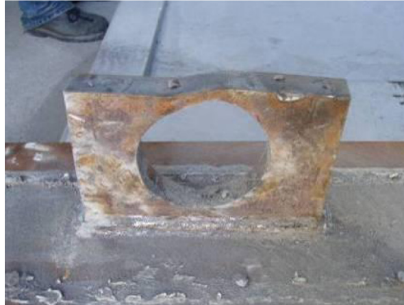
Fig. 5 - Post-test examination of shear connection plate
