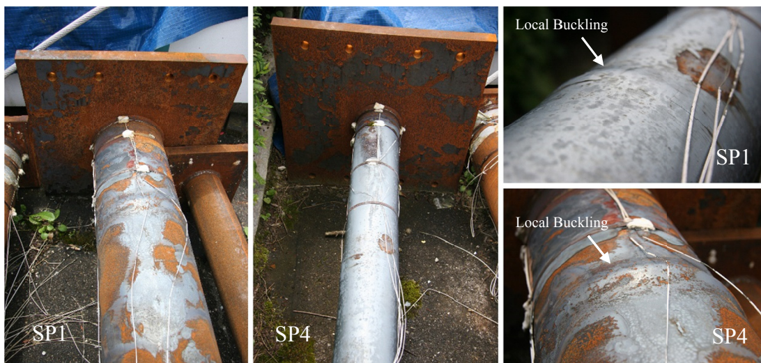
Figure 7. Specimens 1 and 4 after testing with details of buckled tube.
