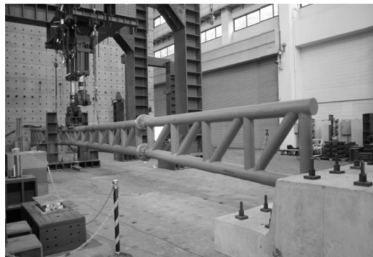
Figure 3. Test of the single CFT truss girder.
