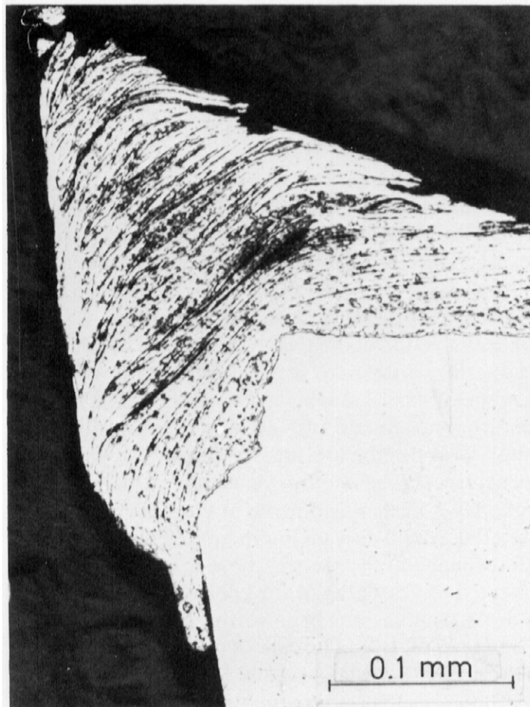
FIGURE 6.20 Section through cutting edge of high speed steel tool after cutting steel at relatively low speed, showing attrition wear (After Wright and Trent 12 ).
