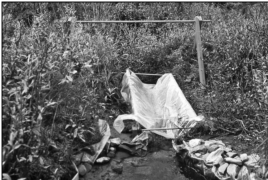
Figure E.1 Volumetric gauging at low flows on a small Alaskan stream. Plastic sheets collect the flow and divert it into a trough. Flow from the trough is collected in a bucket of known volume and the time it takes to fill is recorded (photo by author).
