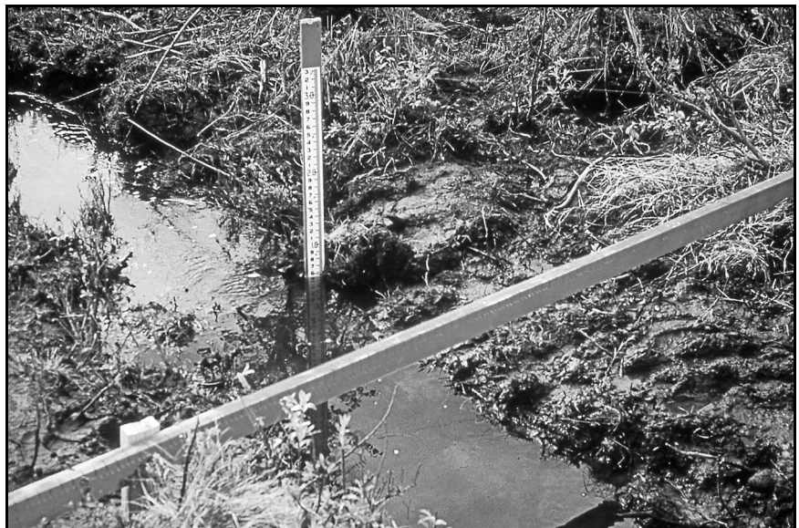
Figure E.13 Staff gauge installed on a small stream (photo by author).
