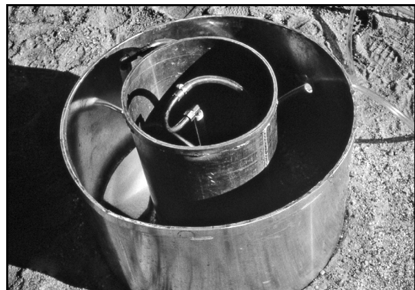
Figure 8.14 A double-ring infiltrometer connected to an apparatus that maintains a constant water level in each ring (photo by author).
