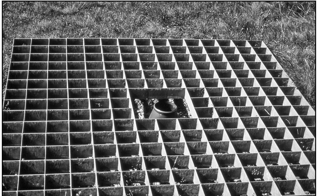
Figure 4.17 Rain gauge with orifice at ground level and surrounded by plastic “egg-crate” structure to eliminate in-splashing (photo by author).
