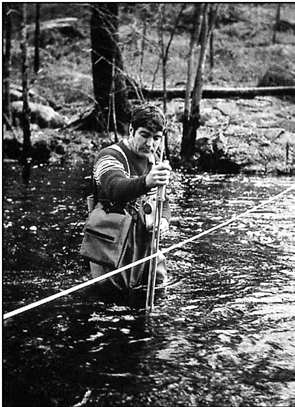
Figure E.3 Velocity-area stream gauging using a wading rod. The tape marking the cross section is visible just in front of the observer (photo by J. V. Z. Dingman).
