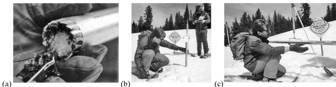
Figure 5.9 Measuring snow depth and water equivalent via a snow tube. (a) Teeth for securing a soil plug at the base of the snow tube. (b) Snow tube is pushed through snowpack to ground to measure depth and capture core. (c) Water equivalent is determined by weighing the tube and snow and subtracting the weight of tube (US Natural Resources Conservation Service, n.d.).
