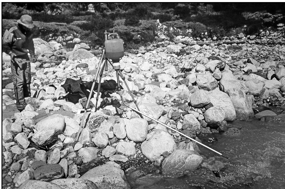
Figure E.8 Injection of dye for dilution gauging in a highly turbulent Himalayan stream, where velocity-area gauging is not feasible (photo courtesy of Richard Pendleton).
