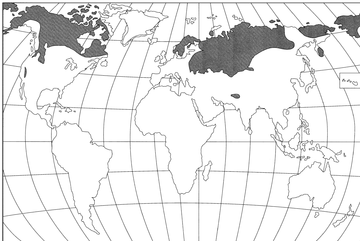
Figure 5.3 Regions in which more than half the annual runoff is derived from snowmelt [L'vovich (1974). World Water Resources and Their Future . Trans. by R. L. Nace, with permission of the American Geophysical Union].
