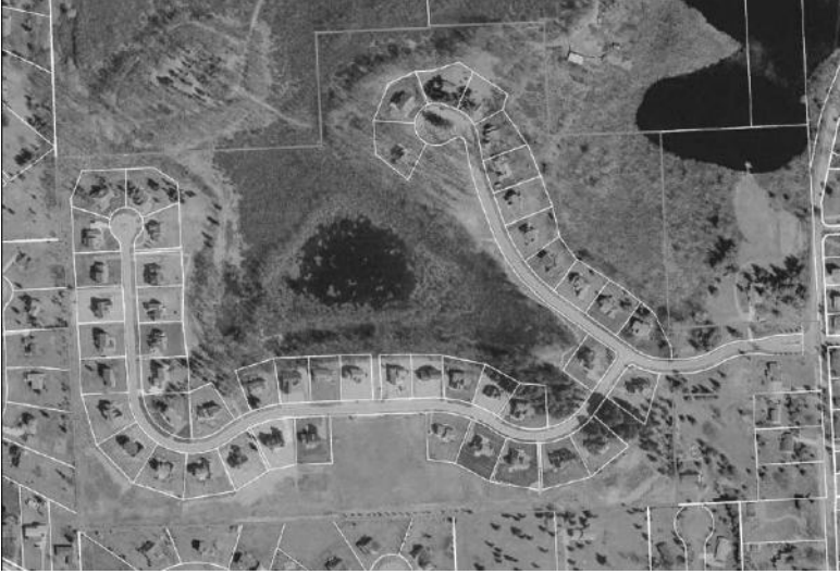
FIGURE 4.3 Solitude Point (Hamburg, Michigan). Overall density: 1 unit per acre; average lot size: 0.5 acres; open space use: wetlands, paths; percentage of open space: 50%. (See color insert after page 136.)
