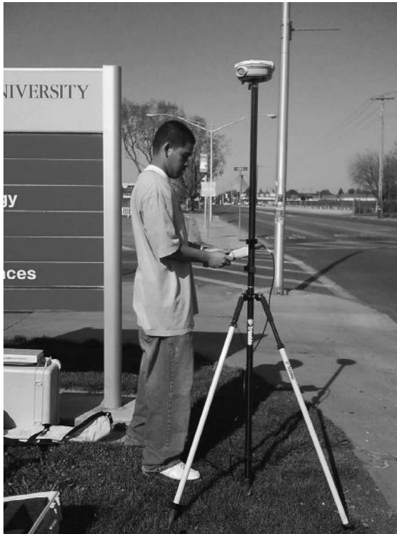
FIGURE 7.4 GPS survey set up. (See color insert after page 136.)
