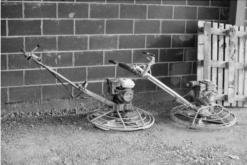
Fig. 5.32. These power trowels are used to improve the quality of the surface of the concrete. They are used when the concrete has gained sufficient strength to support their weight and the weight of the operator, but before the concrete is fully hard. In this case, concrete mixed at 9a.m. was power trowelled at 1p.m.
