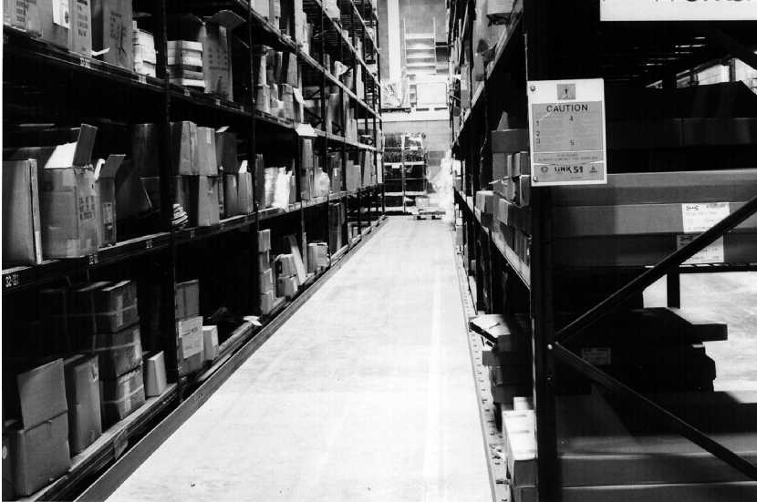
Fig. 3.6. 1.2 m wide storage racking system. There are two fixing feet per bay (except at the end) where the whole load is transmitted to the floor
