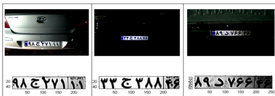
Fig. 7. Examples of extraction license plate using the proposed algorithm in images which have been taken in night time
