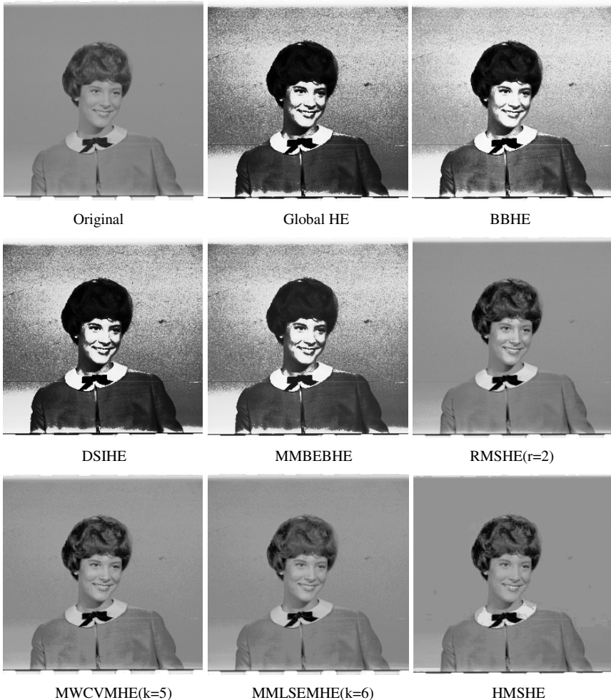
Fig. 3. Enhancement of the girl image based on Global HE, BBHE, DSIHE, MMBEBHE, RMSHE( r=2 ), MWCVMHE( k=5 ), MMLSEMHE( k=6 ), and HMSHE(proposed) methods
