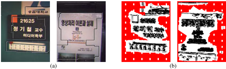
Fig. 7. Text detection examples using MLPs with CAMShift: (a) a scene text image with marked text regions and (b) its corresponding filtered images (TPI).
