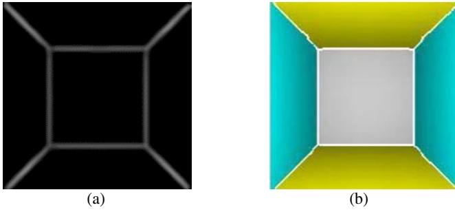
Fig. 3. (a) Soft J-image at scale 2 of the synthetic image. (b) Corresponding segmentation result.
