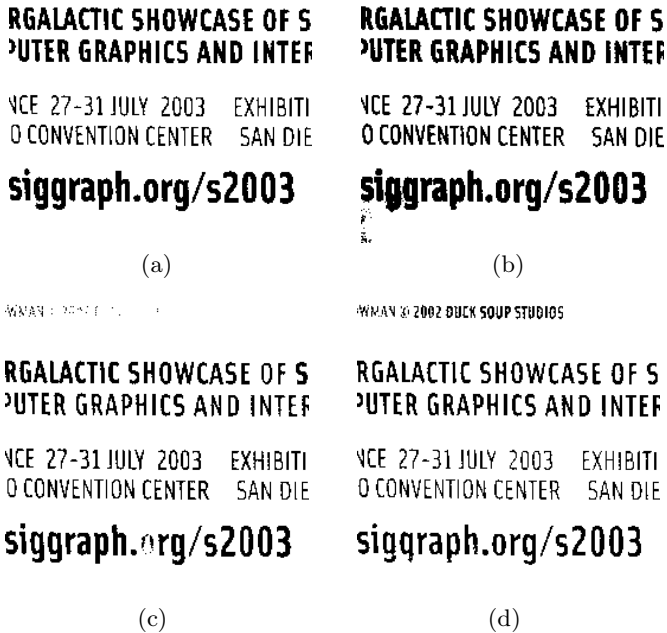
Fig. 6. Binarization results for test image 2: (a) Otsu's method, (b) Liu and Srihari's method, (c) Kim et al.'s method, and (d) proposed method.
