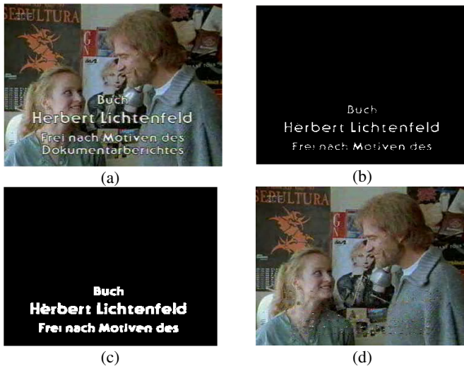
Fig. 5. Results of detection, removal, and restoration for texts: (a) Input image, (b) Extracted text regions before expanding, (c) Text region after expanding, (d) Restoration of removed region.
