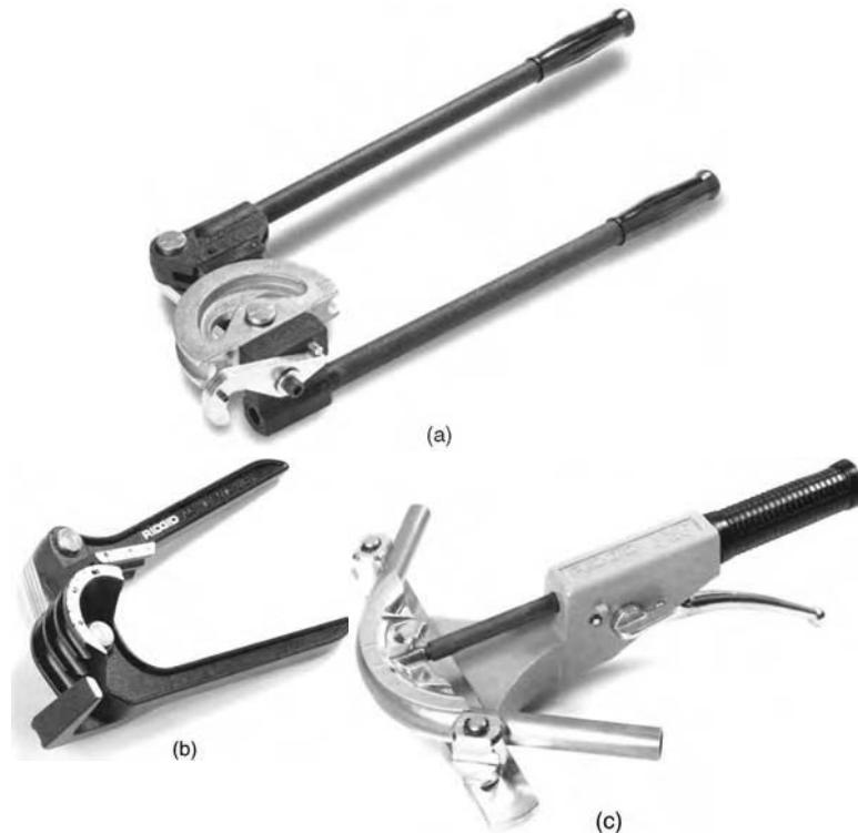
Figure 3.14 (a), (b), (c) Examples of hand held bending machines (Reproduced with permission of Ridgid Tool)
