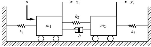
**EXAMPLE 3–4** Obtain the transfer functions  $X_1(s)/U(s)$  and  $X_2(s)/U(s)$  of the mechanical system shown in Figure 3–4.
