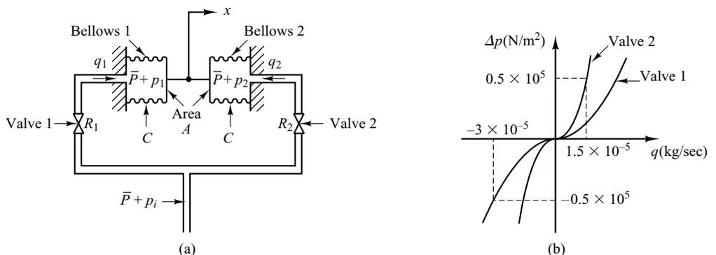
Defining the displacement of the midpoint of the rod that connects two bellows as  $x$ , find the transfer function  $X(s)/P_i(s)$ . Assume that the expansion process is isothermal and that the temperature of the entire system stays at 30°C. Assume also that the polytropic exponent  $n$  is 1.
