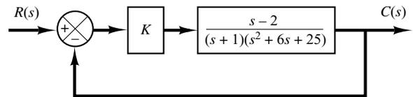
**Figure 5-79** Closed-loop system.
