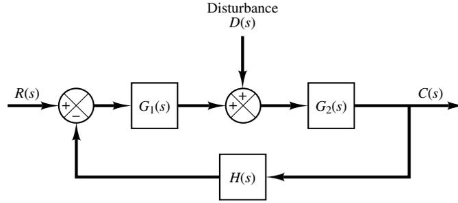
**Closed-Loop System Subjected to a Disturbance.** Figure 2–11 shows a closed-loop system subjected to a disturbance. When two inputs (the reference input and disturbance) are present in a linear time-invariant system, each input can be treated independently of the other; and the outputs corresponding to each input alone can be added to give the complete output. The way each input is introduced into the system is shown at the summing point by either a plus or minus sign.
