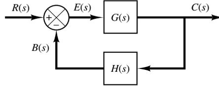
the output of the plant. The output of the sensor is compared with the system input, and the actuating error signal is generated.) In the present example, the feedback signal that is fed back to the summing point for comparison with the input is  $B(s) = H(s)C(s)$ .
