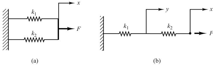
**EXAMPLE 3-1** Let us obtain the equivalent spring constants for the systems shown in Figures 3-1(a) and (b), respectively.
