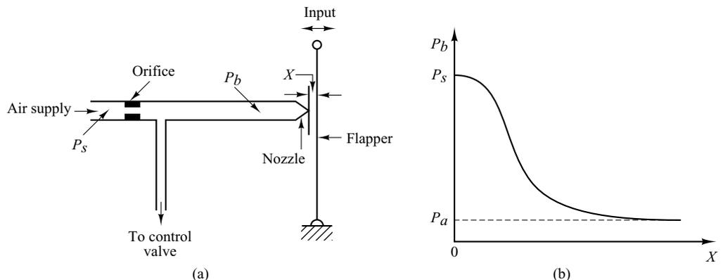
**Pneumatic Relays.** In practice, in a pneumatic controller, a nozzle-flapper amplifier acts as the first-stage amplifier and a pneumatic relay as the second-stage amplifier. The pneumatic relay is capable of handling a large quantity of airflow.
