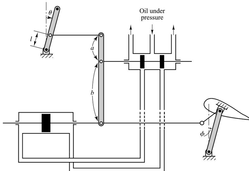
**Figure 4-51** Aircraft elevator control system.
