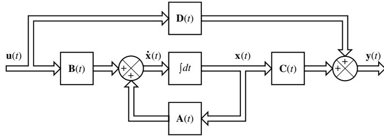
the operating state are discussed in Section 2-7.) A block diagram representation of Equations (2-12) and (2-13) is shown in Figure 2-14.
