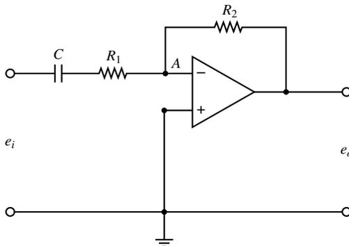
**Figure 3-39** Operational-amplifier circuit.
