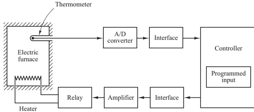
to a digital temperature by an A/D converter. The digital temperature is fed to a controller through an interface. This digital temperature is compared with the programmed input temperature, and if there is any discrepancy (error), the controller sends out a signal to the heater, through an interface, amplifier, and relay, to bring the furnace temperature to a desired value.
