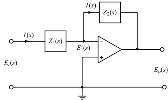
**Impedance Approach to Obtaining Transfer Functions.** Consider the op-amp circuit shown in Figure 3–17. Similar to the case of electrical circuits we discussed earlier, the impedance approach can be applied to op-amp circuits to obtain their transfer functions. For the circuit shown in Figure 3–17, we have
