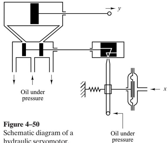
**Figure 4-50** Schematic diagram of a hydraulic servomotor.
