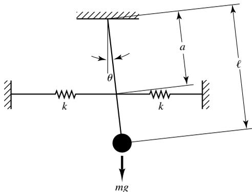
**Figure 3-33** Spring-loaded pendulum system.
