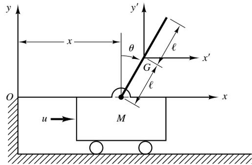
**Figure 3-34** Inverted-pendulum system.
