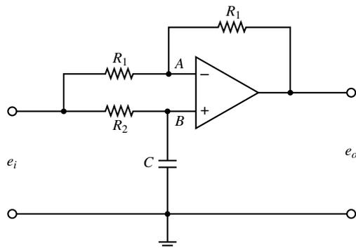
**A–3–6.** Obtain the transfer function  $E_o(s)/E_i(s)$  of the op-amp circuit shown in Figure 3–26.
