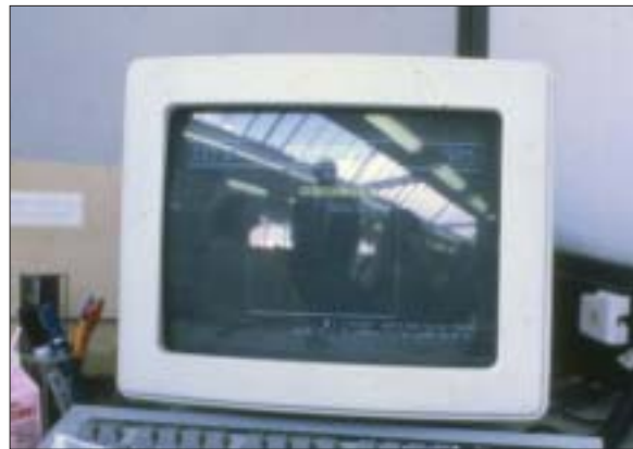
Figure 26 Severe reflections of a rooflight on a screen with no anti-reflection treatment
