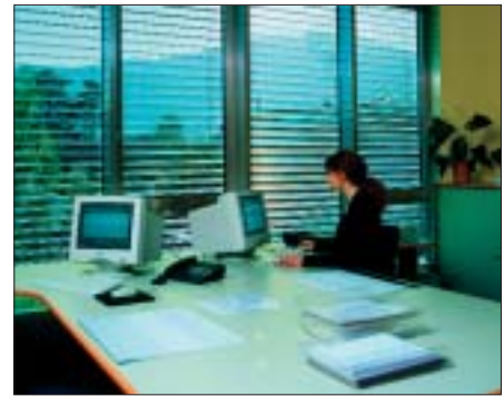
Figure 42 Screen user in front of window with blinds down maintaining view but avoiding glare
