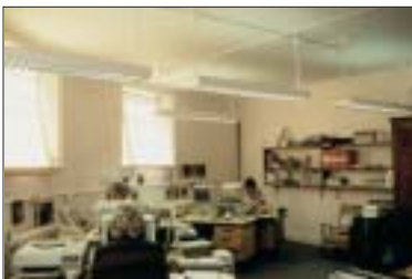
Figure 43 Sun hitting blinds can be reflected on screen
