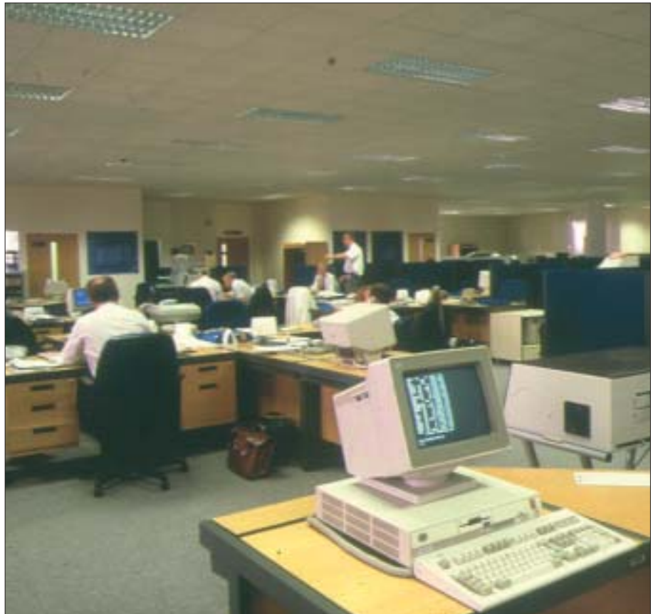
Figure 20 Dark ceiling due to low working plane and carpet reflectance
