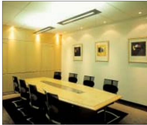
Figure 45 Meeting room showing use of downlights. The bright flash of the downlights close to the end wall may be distracting
