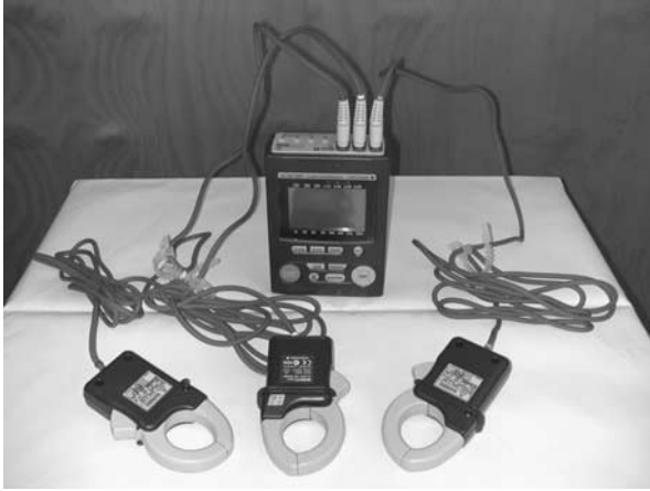
13.12 Electrical power measurement logger (reproduced by courtesy of Mobile Architecture and Built Environment Laboratory, Deakin University, Geelong).
