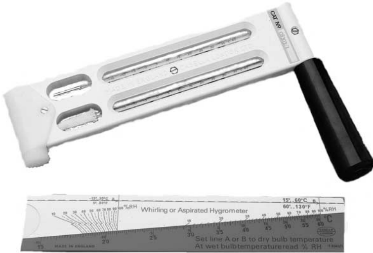
1.4 Sling psychrometer or whirling hygrometer (reproduced by courtesy of Casella CEL Ltd).
