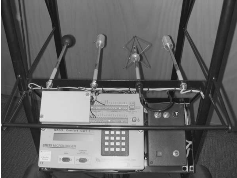
1.3 Thermal comfort data logger (reproduced by courtesy of Mobile Architecture and Built Environment Laboratory, Deakin University, Geelong).
