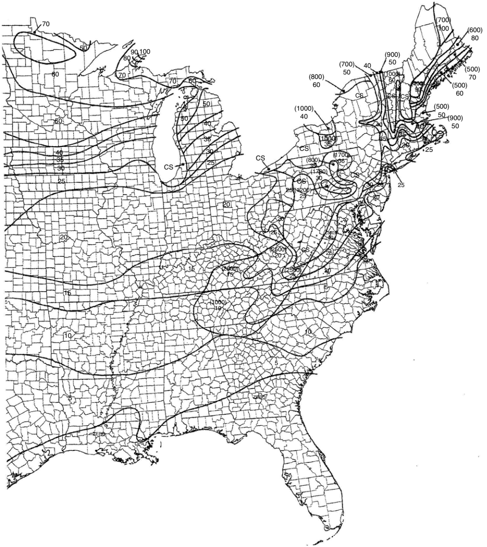
FIGURE 11.4 Basic snowfall in eastern United States ( Source: From ASCE; used with permission. )
