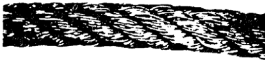
Rope subjected to drum crushing. Note the distortion of the individual wires and displacement from their original position. This is usually caused by the rope scrubbing on itself.
