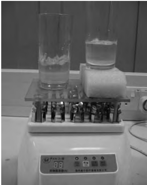
Figure 18.7 Altering structural frequency using base isolation.
