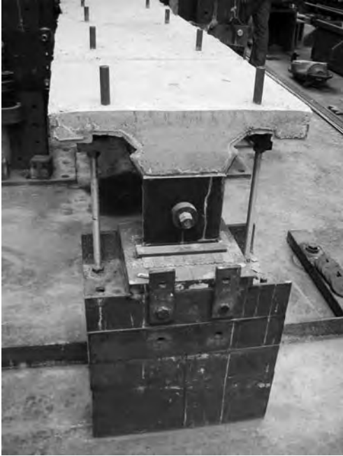
Figure 11.9 An eccentrically post-tensioned beam.
