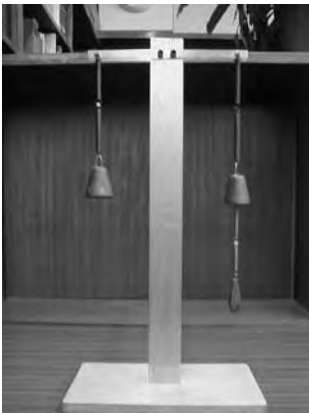
Figure 18.5 Comparison of vibration with and without a tuned mass damper.
