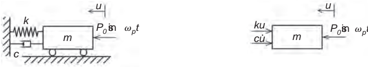
(a) A SDOF system subject to a harmonic load (b) Free-body diagram
