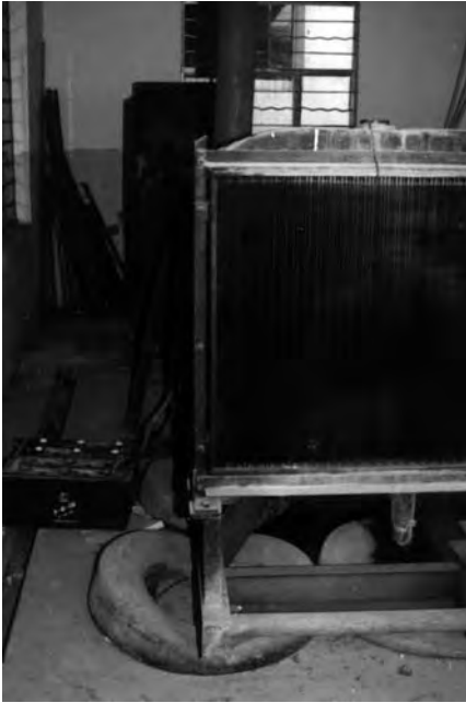
Figure 18.8 Tyres used for base isolation (courtesy of Professor B. Zhuang, Zhejiang University, China).
