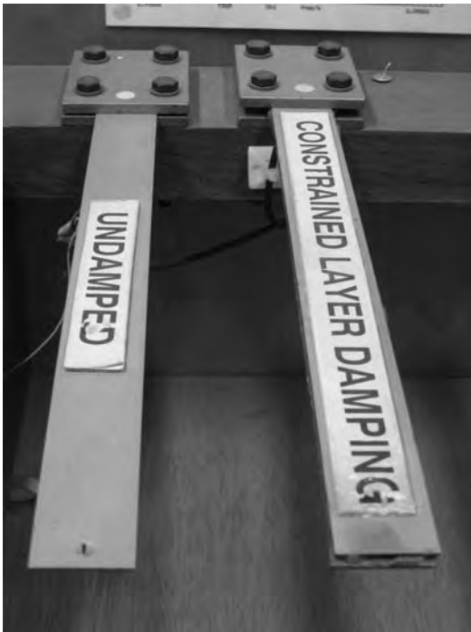
Figure 15.10 Demonstration of an overcritically-damped system.
