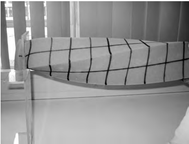
Figure 5.5 Effect of torsion.
