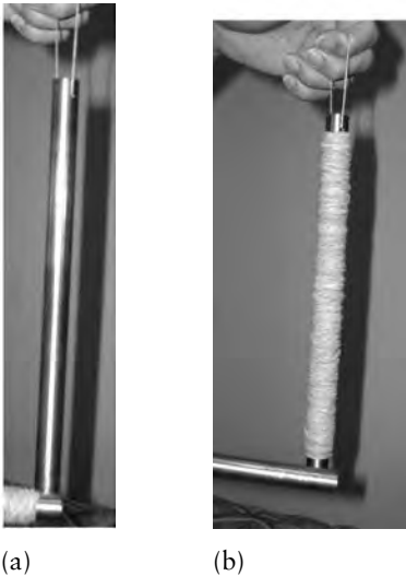
Figure 17.3 Effect of damping on sound transmission.
