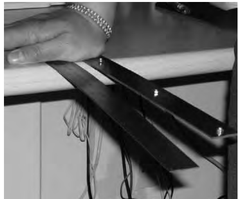
(b) The double ruler stops vibration more quickly than the single ruler
