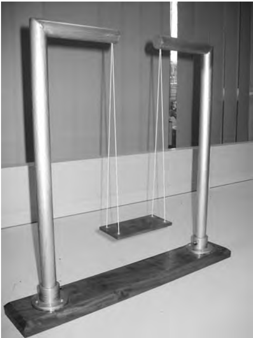
Figure 14.5 A model of a translational suspended system and a rotational suspended system.
