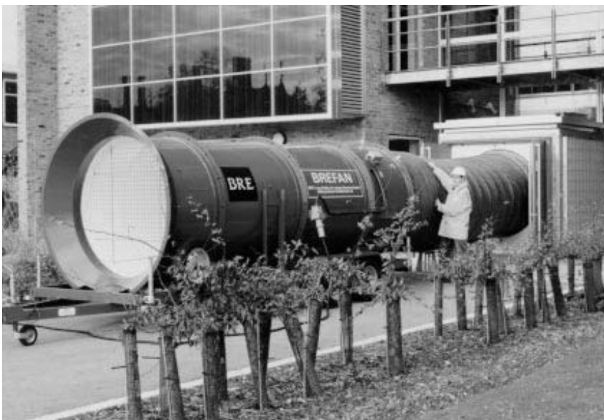
Figure 3.14 Apparatus for measuring air leakage rates for an entire building (BREFAN)
