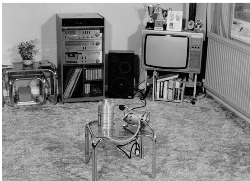
Figure 2.51 Monitoring biological particles, including airborne bacteria, fungi and house dust mites in a domestic environment
