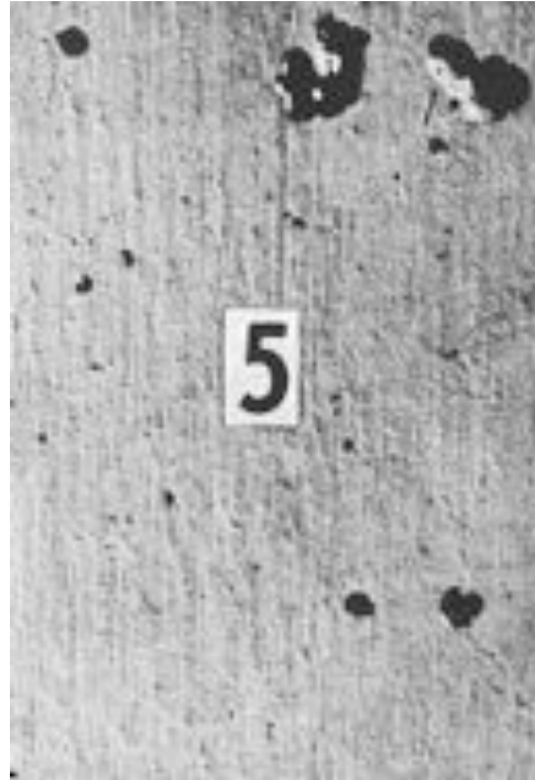
Fig. 3-1. Table to classify concrete surface, reported by the Commission W 29 of CIB. Courtesy of CIB.
