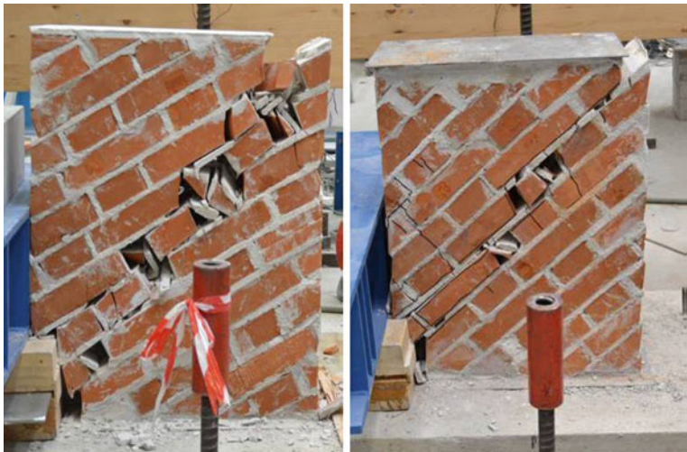
Fig. 1.42 Specimens M22 ( \theta = 22.5^\circ ) and M45 ( \theta = 45^\circ ) at failure (Facconi et al. 2014)
