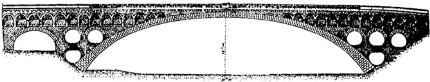
Fig. 3.9 The Plauen bridge (1903–1905) with 90 m span (from D'Agostino and Bellomo 2001)
