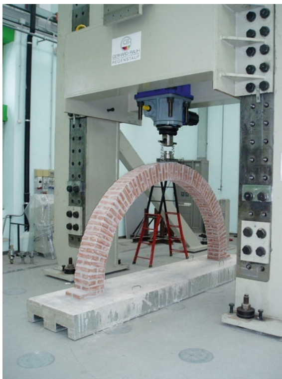
Fig. 3.53 The masonry arch during a test
