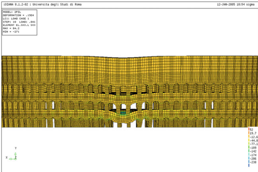
Fig. 7.39 Partial failure of the outer wall due to demolition of two piers (Como et al. 2006)
