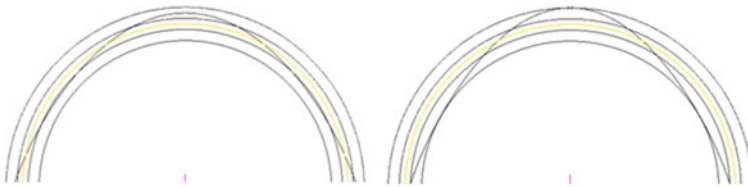
Fig. 2.5 Pressure lines in the elastic no tension arch at its initial state, with fixed springings, and near the mechanism state, just after the thrust drop (private communication by N. Zani, Department of Constructions, Univ. of Florence, Italy, July Zani 2011)
