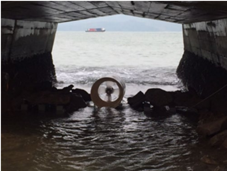
Figure E9.6.1 Micro Marine Turbine Prototype Demonstration in Hong Kong Gold Coast. © Sino
