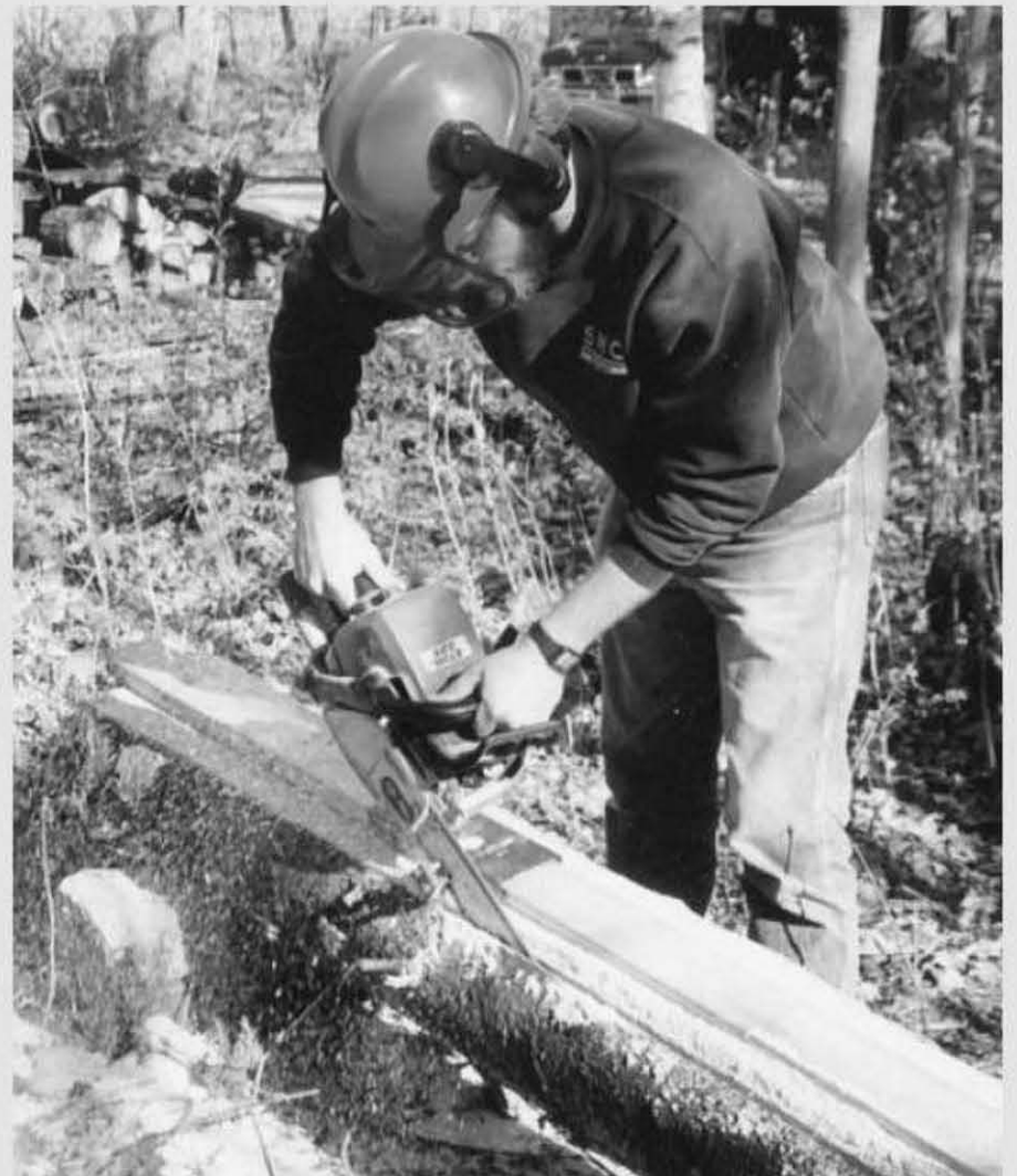
Fig. 3.3b: Doug Kerr cuts a slab off a fir log with the Beam Machine.
