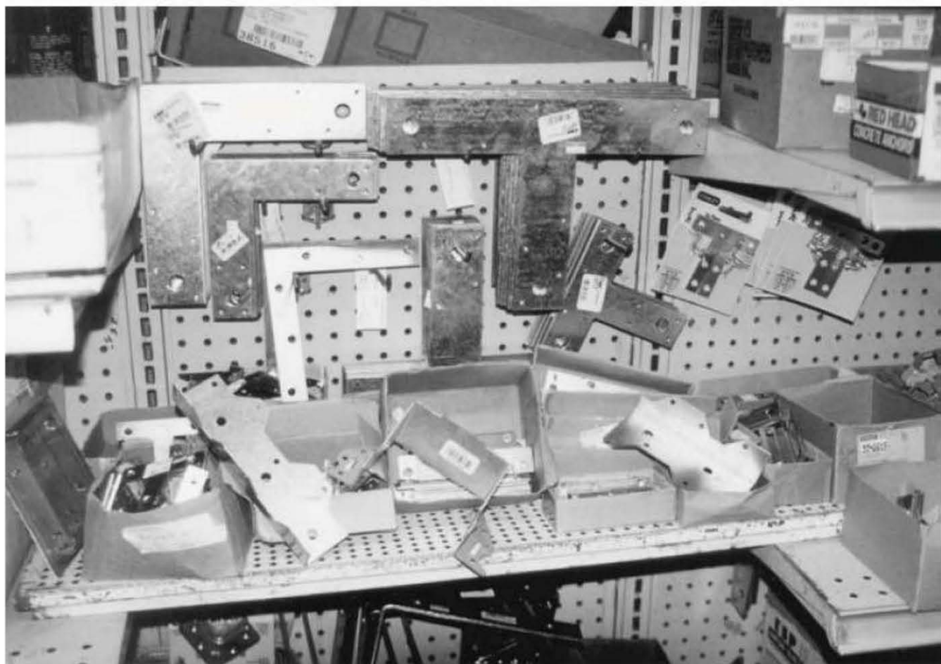
Fig. 4.12: There is a great little hardware store in Pahoehoe, Hawaii, with quite a selection of metal connectors. Practically all new construction in Hawaii makes use of these connectors, because of severe expected wind loads.
