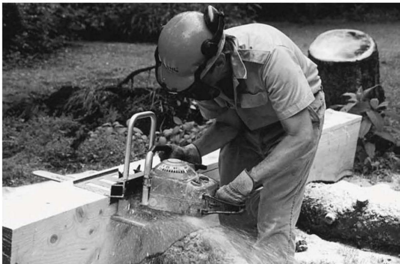
Fig. 3.4: Richard Freudenberger tests the Logosol Timber Jig portable chainsaw mini-mill. Photo by Don Osby, reproduced by permission of BackHome Magazine, No. 66, p. 48.
