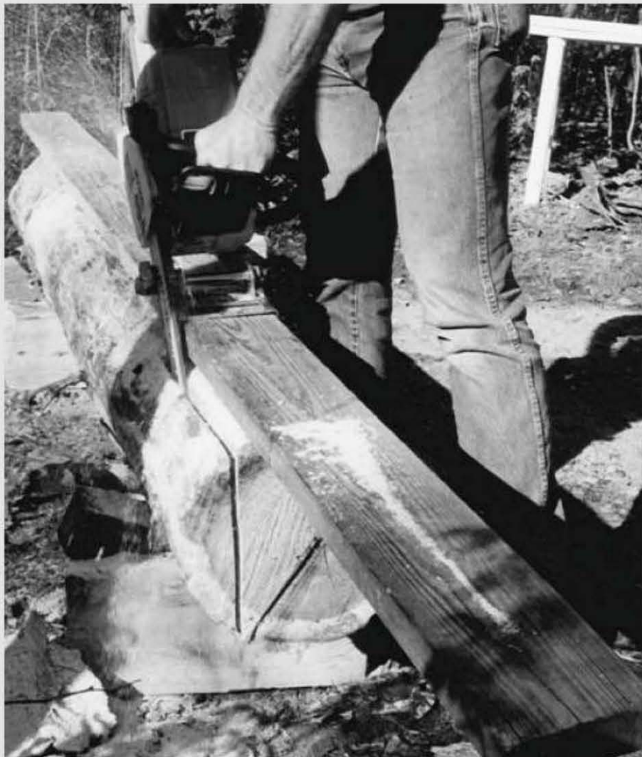
Fig. 3.3a: The Granberg Mini-Mill uses a wide two-by-six trackway for improved stability.
