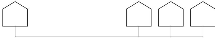
16.02 Shared infrastructure, such as roads and utilities, reduces the impact of new construction.
