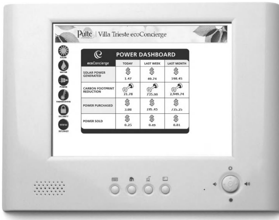
Figure 4-6 Every home has an ecoConcierge unit, which tracks the home’s energy use and offers comparisons to average use in the community. Image © 2009, In2 Networks, Inc. In2 Solar Dashboard, www.in2networks.com .
