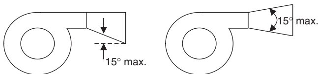
Figure 6.7 Fan discharge transitions.
