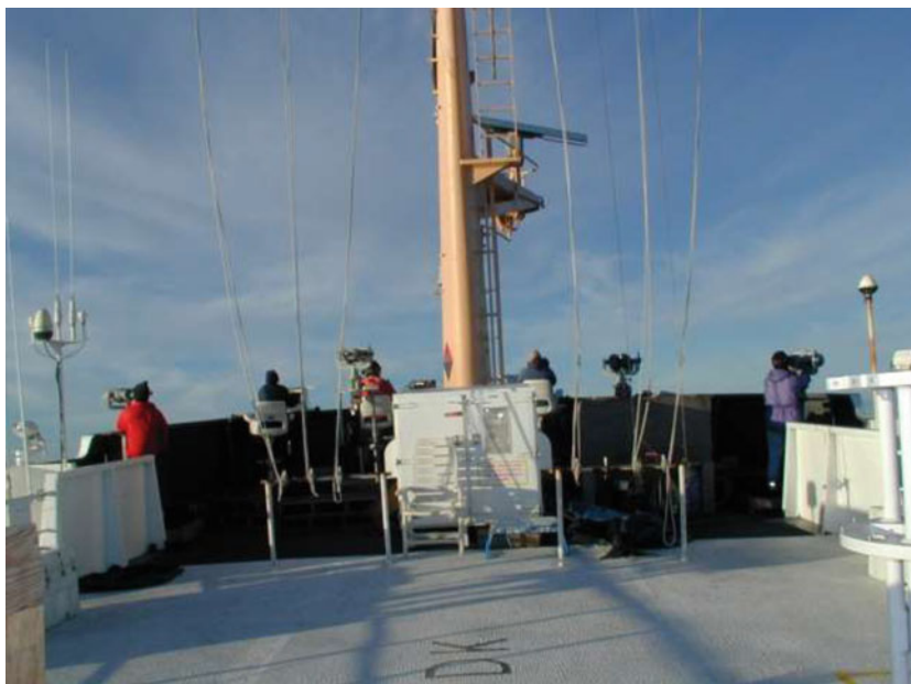
Fig. 10.4 Flying bridge setup on the NOAA ship David Starr Jordan during a survey off the California, Oregon and Washington coasts. There were three rotating marine mammal observers and one seabird observer. The inner tripod-mounted binoculars were used by the centre marine mammal observer during chases and the seabird observer for flock counts. Tripod-mounted binoculars with 25 \times or 30 \times magnification have a narrow field of view, and so are unsuited to surveys of cetaceans that occur singly or in small groups that do not give many sighting cues, but they are very effective for detecting schools of dolphins at great distances. Photo: courtesy SWFSC/NOAA
