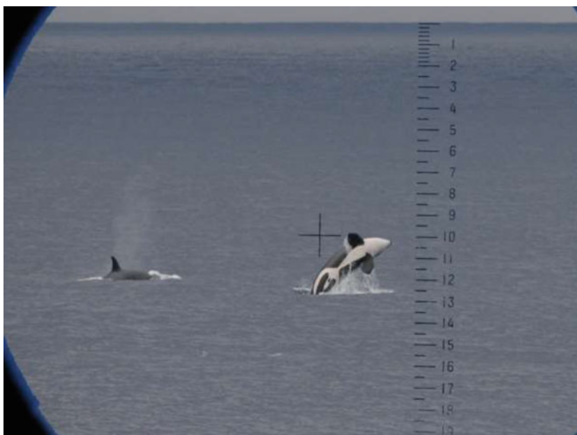
Fig. 10.5 View through large tripod-mounted binoculars. Lining up the 0 reticle reading with the horizon enables conversion of the reticle reading of the sighting to a distance from the observer (which requires knowing the height of the observer above sea level). Image constructed from two photos for illustrative purposes. Photo: Cornelia Oedekoven
