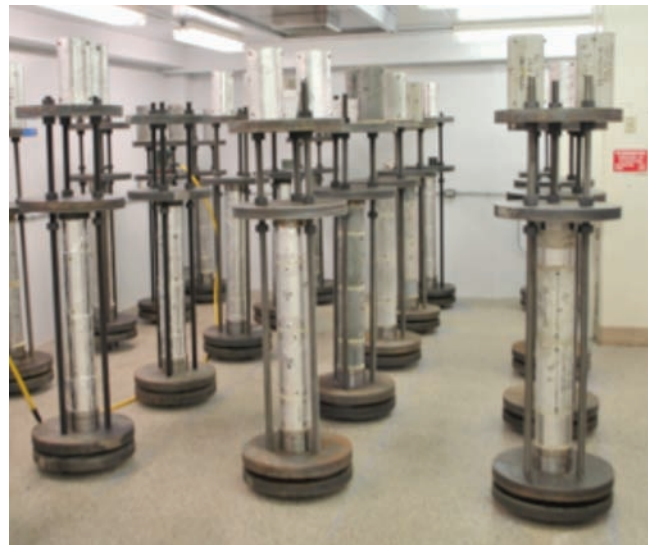
Figure 10-28. ASTM C512 creep test frames loaded with both sealed and unsealed specimens.
