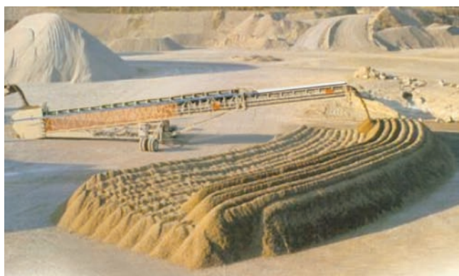
Figure 6-25. Stockpile of aggregate at a ready mix plant.
