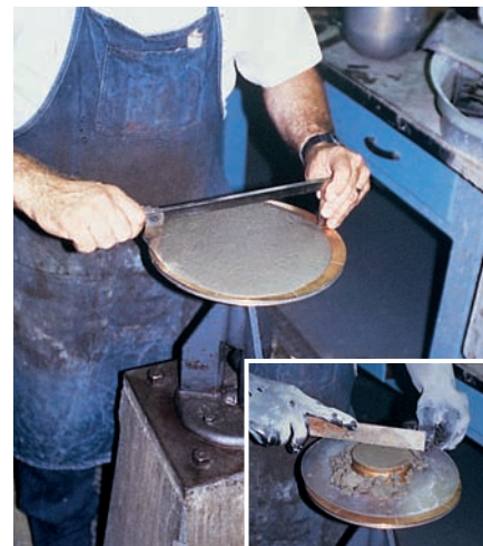
Figure 3-42. Consistency test for mortar using the flow table. The mortar is placed in a small brass mold centered on the table (inset). For skin safety the technician wears protective gloves while handling the mortar. After the mold is removed and the table undergoes a succession of drops, the diameter of the pat is measured to determine consistency.
