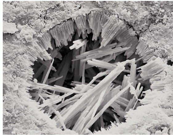
Figure 11-36. White secondary ettringite deposits in void. Field width 64 \mu\text{m} .
