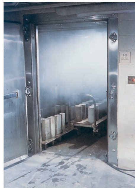
Figure 18-12. Controlled moist curing in the laboratory for standard test specimens at a relative humidity of 95% to 100% and temperature of 23 \pm 2^\circ\text{C} ( 73.5 \pm 3.5^\circ\text{F} ) (ASTM C511 or AASHTO M 201).
