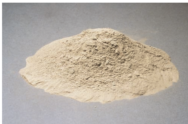
Figure 4-2. Fly ash, a byproduct of the combustion of pulverized coal in electric power generating plants, has been used in concrete since the 1930s.
