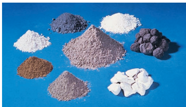
Figure 3-21. Blended cements use a combination of portland cement or clinker and gypsum blended or interground with pozzolans, slag, or fly ash. Shown is blended cement (center) surrounded by (right and clockwise) clinker, gypsum, portland cement, fly ash, slag, silica fume, and calcined clay.
