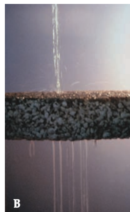
Figure 2-7. a) Pervious concrete allows for infiltration of water, reducing runoff from the site (Courtesy of B. Banka). b) Side view of water percolating through pervious concrete.
