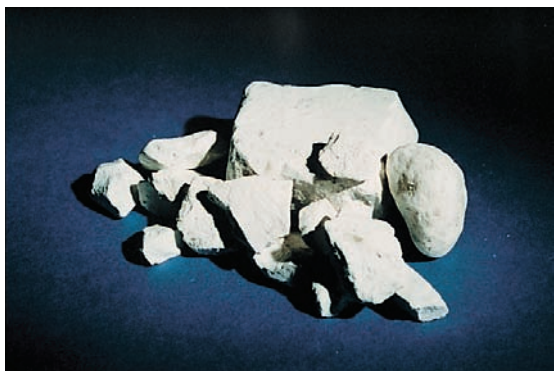
Figure 3-10. Gypsum, a source of sulfate, is interground with portland clinker to form portland cement. It helps control setting, drying shrinkage properties, and strength development.
