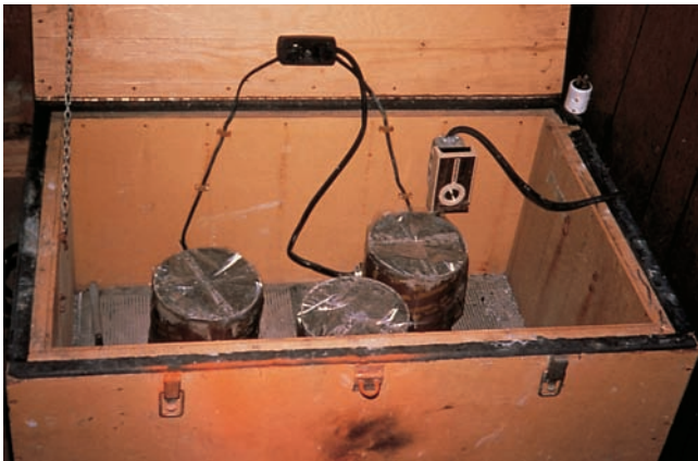
Figure 17-15. Insulated curing box with thermostat for curing test cylinders. Heat is supplied by electric rubber heating mats on the bottom. A wide variety of designs are possible for curing boxes.
