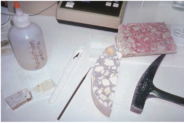
Figure 11-26. The depth of carbonation is determined by wetting a freshly fractured surface of concrete with phenolphthalein solution.
