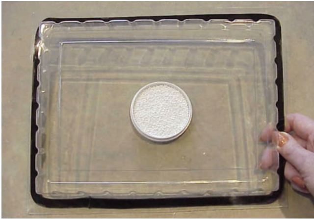
Figure 14-7. Moisture vapor emission rate is determined according to ASTM F1869 using commercially available calcium chloride kits that absorb moisture from a specific test area over a known length of time.
