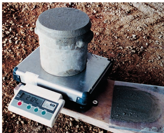
Figure 18-4. Fresh concrete is measured in a container of known volume to determine density (unit weight).
