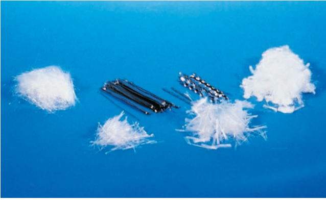
Figure 8-13. Steel, glass, synthetic and natural fibers with different lengths and shapes can be used in concrete.
