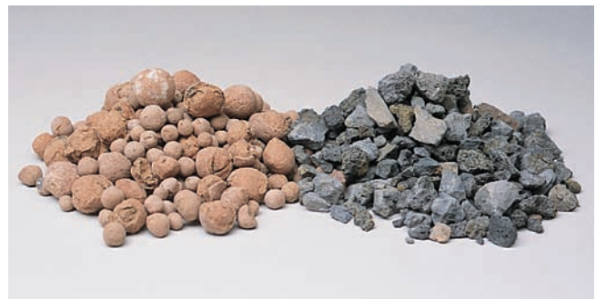
Figure 6-3. Lightweight aggregate. Expanded clay (left) and expanded shale (right).
