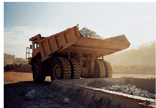
Figure 3-6. Quarry rock is trucked to the primary crusher.
