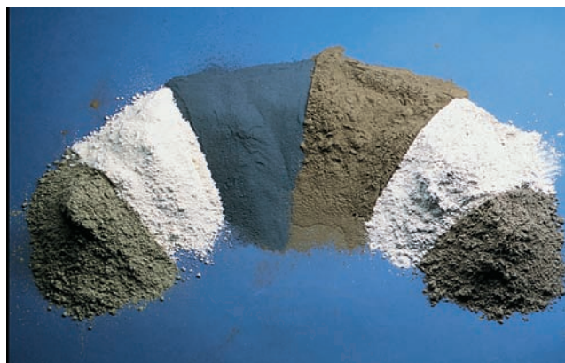
Figure 4-1. Supplementary cementitious materials. From left to right, fly ash (Class C), metakaolin (calcined clay), silica fume, fly ash (Class F), slag cement, and calcined shale.
