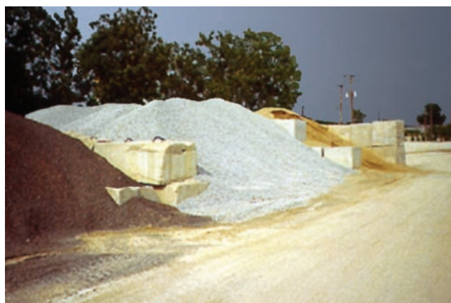
Figure 6-26. Bulkheads or dividers should be used to avoid contamination of aggregate stockpiles.
