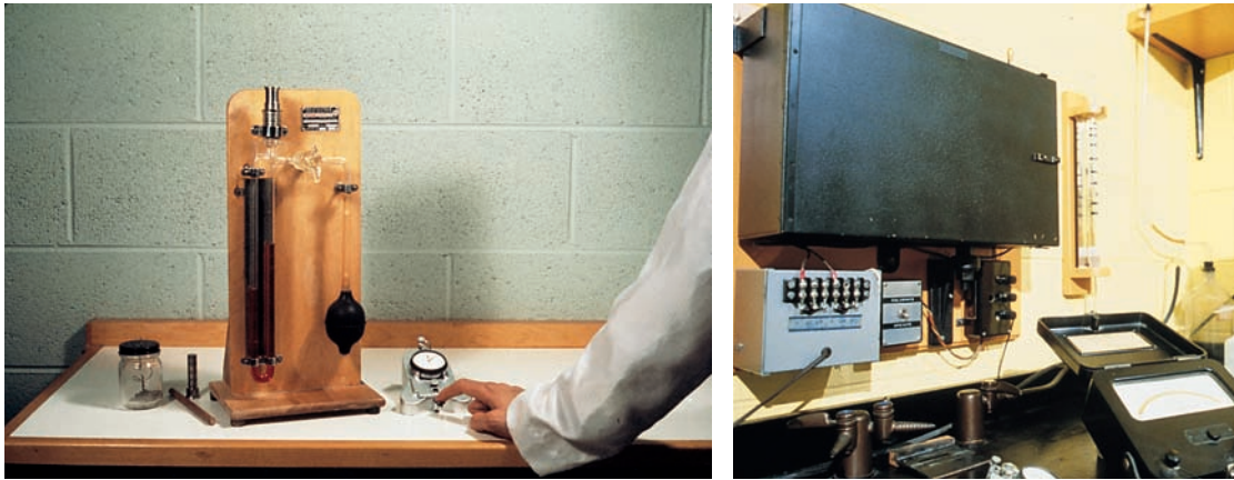
Figure 3-37. Blaine test apparatus (left) and Wagner turbidimeter (right) for determining the fineness of cement.
