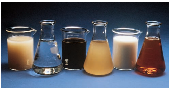
Figure 7-1. Liquid admixtures, from far left to right: antiwashout admixture, shrinkage reducer, water reducer, foaming agent, corrosion inhibitor, and air-entraining admixture.
