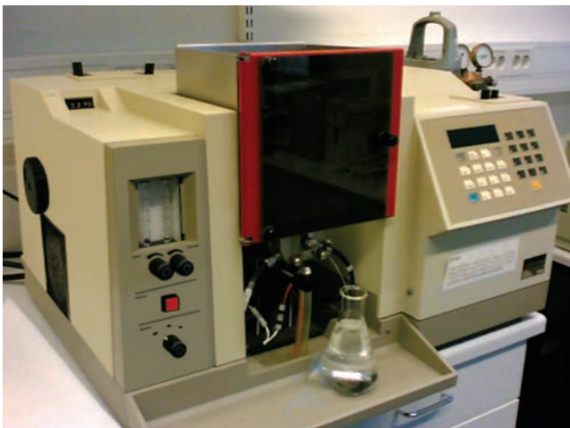
Figure 5-2. An atomic absorption spectrophotometer can be used to detect concentration of elements in the laboratory analysis of water.
