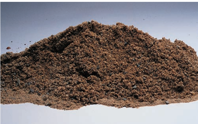
Figure 6-1. Fine aggregate (sand).
