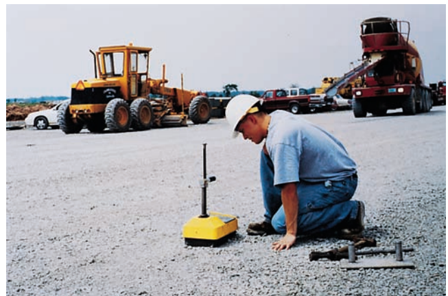
Figure 14-4. Nuclear gauges containing radioactive sources used to measure soil density and moisture can determine if a subbase has been adequately compacted.
