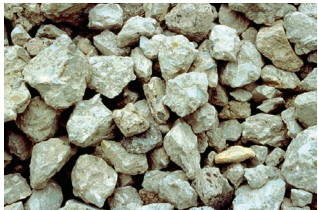
Figure 2-12. Concrete from demolished structures can be recycled and is commonly reused as fill or road base.
