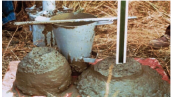
Figure 7-7. High-range water reducers, also known as superplasticizers, produce flowing concrete with slumps greater than 150 mm (6 in.).
