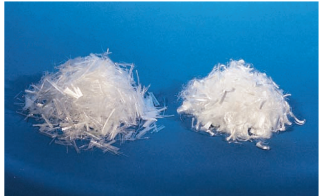
Figure 8-19. Polypropylene fibers are produced either as (left) fine fibrils with rectangular cross section or (right) cylindrical monofilament.
