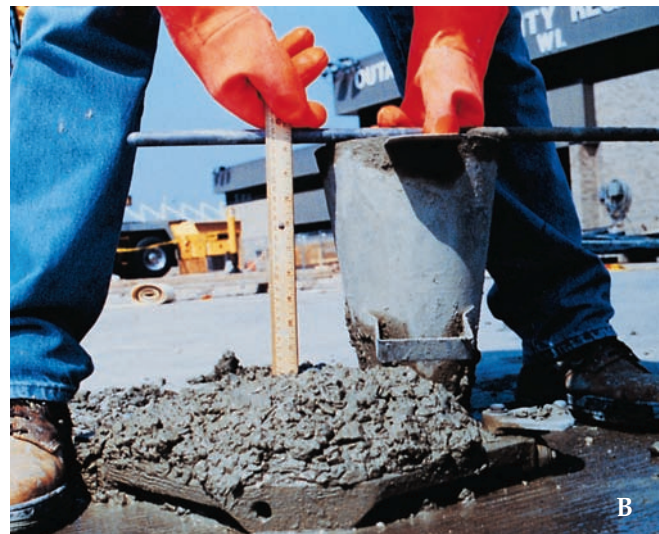
Figure 18-2. Slump test for consistency of concrete. Figure A illustrates lower slump, Figure B a higher slump.
