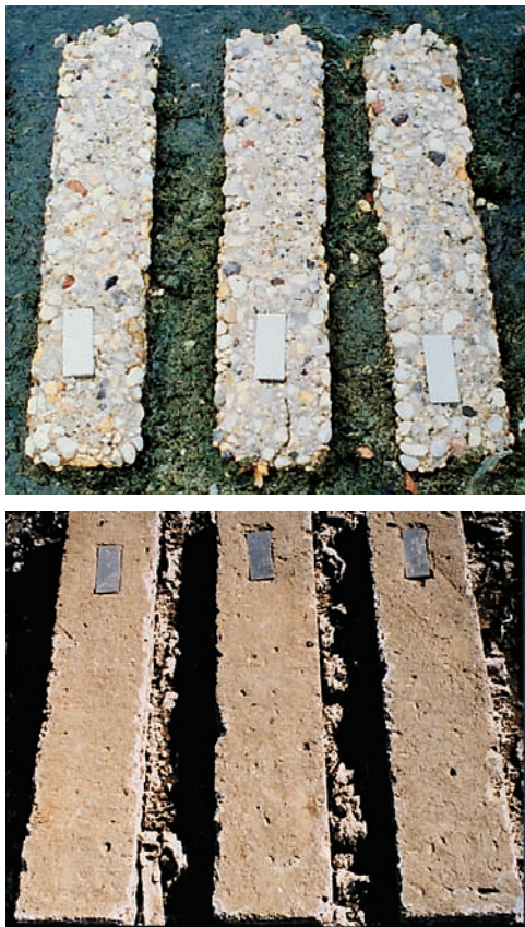
Figure 3-17. Specimens used in the outdoor sulfate test plot in Sacramento, California, are 150 x 150 x 760-mm (6 x 6 x 30-in.) beams. A comparison of ratings is illustrated: (top) a rating of 5 for 12-year old concretes made with Type V cement and a water-to-cement ratio of 0.65; and (bottom) a rating of 2 for 16-year old concretes made with Type V cement and a water-to-cement ratio of 0.37 (Stark 2002).
