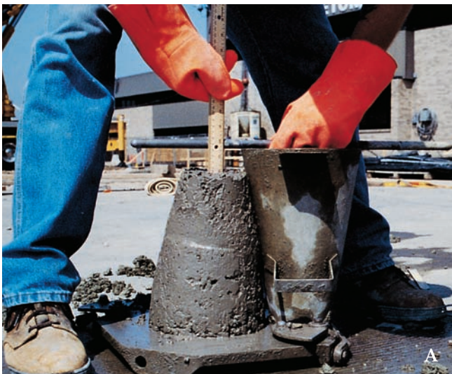
Figure 18-2. Slump test for consistency of concrete. Figure A illustrates lower slump, Figure B a higher slump.
