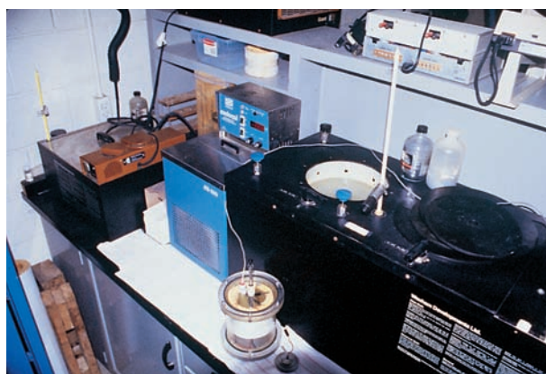
Figure 3-43. Heat of hydration can be determined by (left) ASTM C186 or by (right) a conduction calorimeter.
