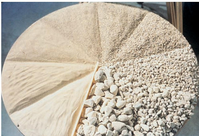
Figure 6-8. Range of particle sizes found in aggregate for use in concrete.
