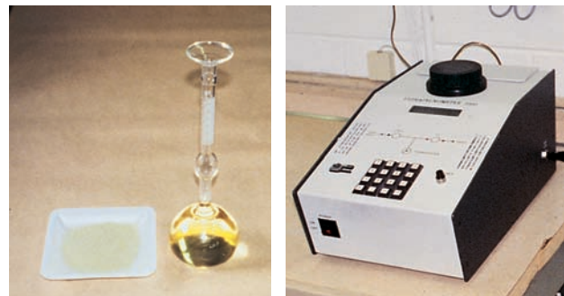
Figure 3-46. Density of cement can be determined by (left) using a Le Chatelier flask and kerosene or by (right) using a helium pycnometer.
