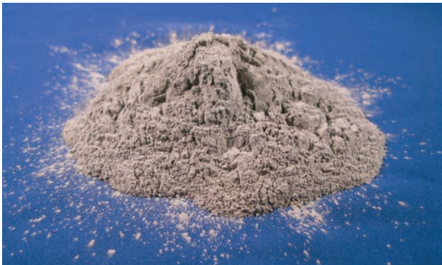
Figure 3-1. Portland cement is a fine powder that when mixed with water becomes the glue that holds aggregates together in concrete.
