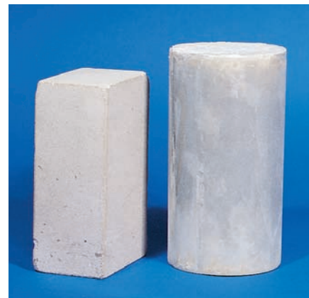
Figure 3-2. Isle of Portland quarry stone (after which portland cement was named) next to a cylinder of modern concrete.
