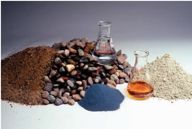
Figure 1-1. Concrete components: cement, water, coarse aggregate, fine aggregate, supplementary cementing materials, and chemical admixtures.
