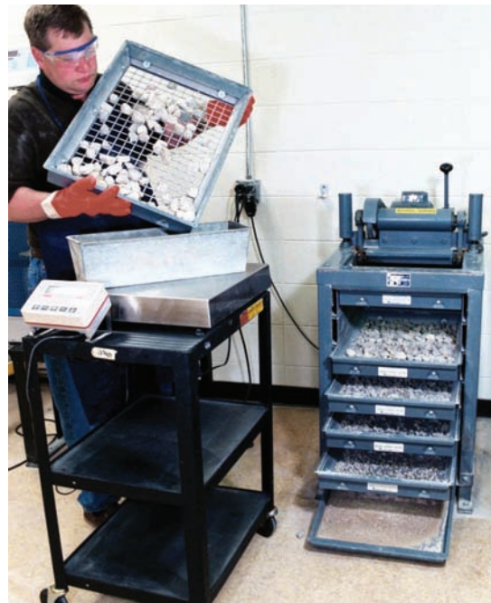
Figure 6-9. Making a sieve analysis test of coarse aggregate in a laboratory.
