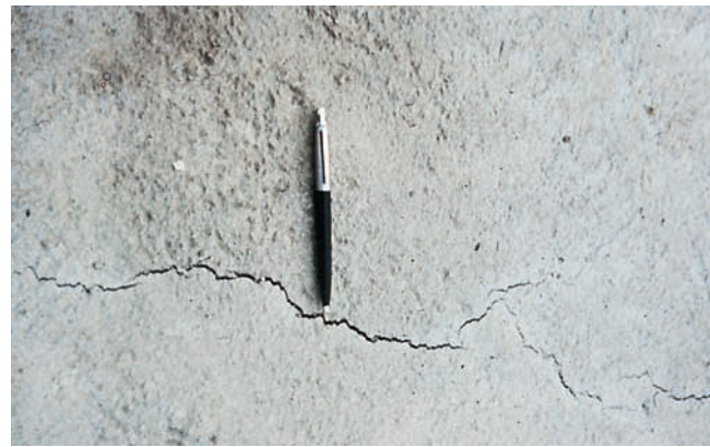
Figure 10-6. Plastic shrinkage cracks resemble tears in fresh concrete.
