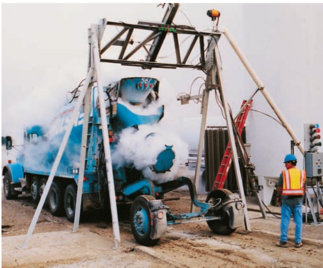
Figure 16-1. Liquid nitrogen added directly into a truck mixer at the ready mix plant is an effective method of reducing concrete temperature for mass concrete placements or during hot-weather concreting.
