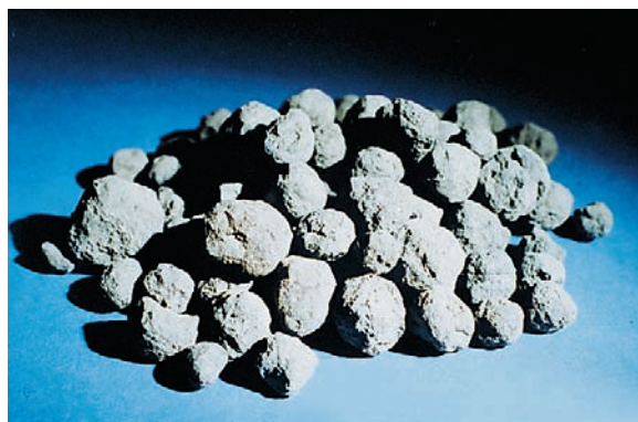
Figure 3-8. Portland cement clinker is formed by burning calcium and siliceous raw materials in a kiln. This particular clinker is about 20 mm (3/4 in.) in diameter.
