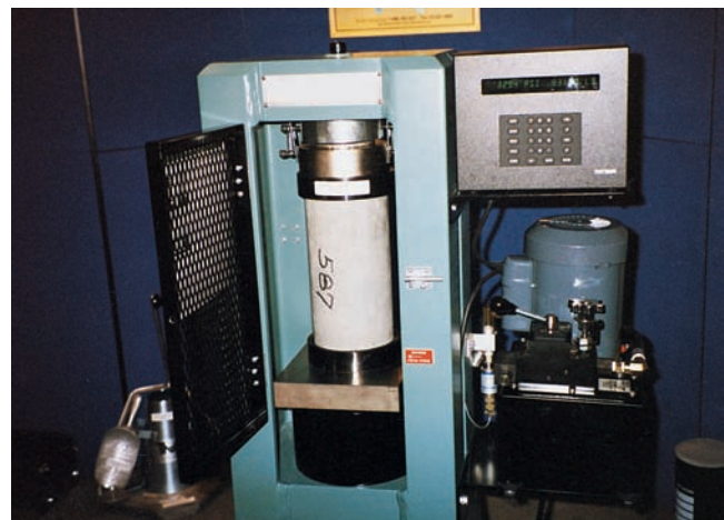
Figure 9-29. Testing a 150-mm x 300-mm (6-in. x 12-in.) concrete cylinder in compression. The load on the test cylinder is registered on the display.
