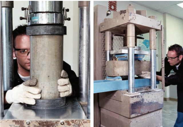
Figure 18-19. Testing hardened concrete specimens: (left) cylinder, (right) beam.
