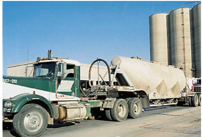
Figure 1-5. The majority of all cement is shipped to ready mixed concrete producers in cement trucks.
