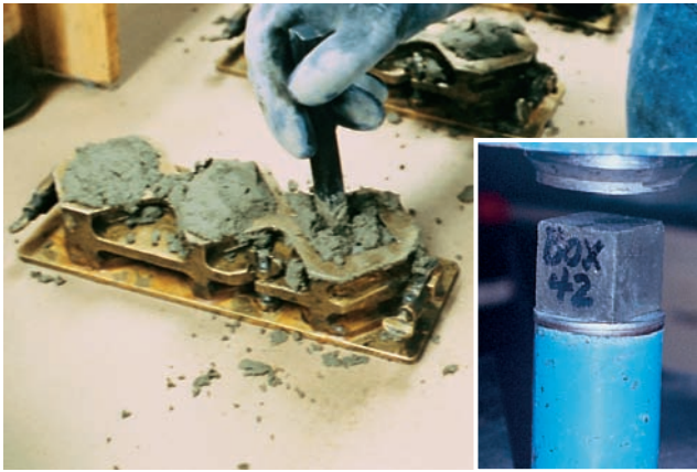
Figure 3-32. 50-mm (2-in.) mortar cubes are cast (left) and crushed (right) to determine strength characteristics of cement.
