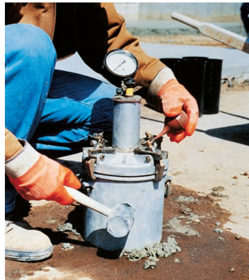
Figure 18-5. Pressure-type meter for determining air content.
