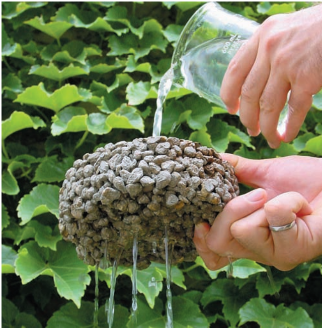
Figure 20-14. Pervious concrete's key characteristic is the open-pore structure that allows high rates of water transmission.
