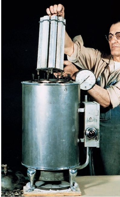
Figure 3-40. In the soundness test, 25-mm square bars are exposed to high temperature and pressure in the autoclave to determine the volume stability of the cement paste.
