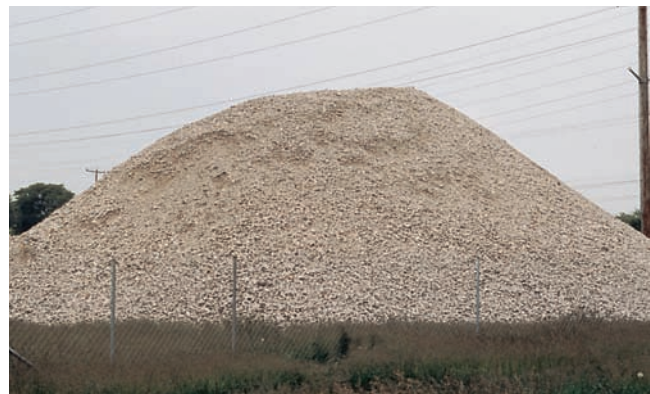
Figure 6-5. Stockpile of recycled-concrete aggregate.
