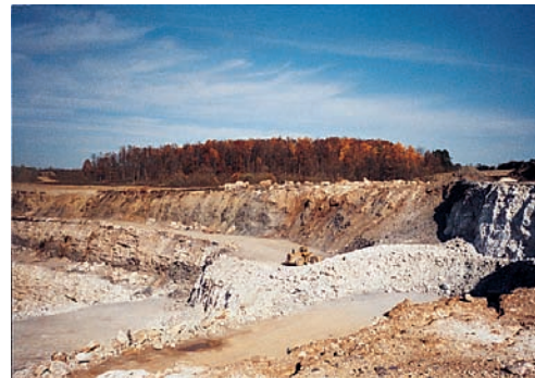
Figure 3-5. Limestone, a primary raw material providing calcium in making cement, is quarried near the cement plant.
