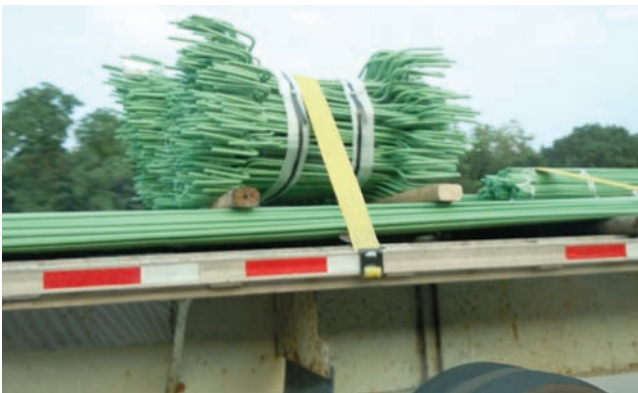
Figure 8-7. Shipping of epoxy-coated reinforcing bars.
