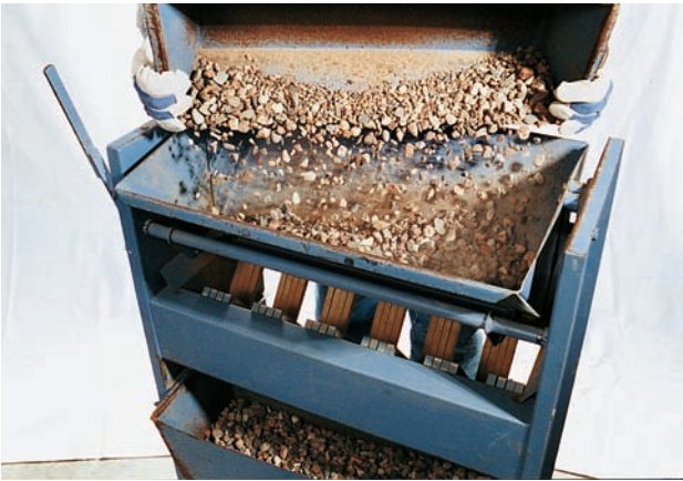
Figure 18-1. Sample splitter commonly used to reduce coarse aggregate samples.
