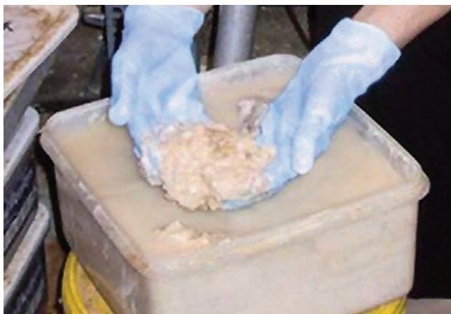
Figure 11-34. Thauwasite deterioration of concrete cubes (Courtesy of R.D. Hooton).
