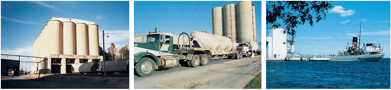
Figure 3-51. Portland cements are shipped from the plant silos to the user in bulk by (left to right) rail, truck, or water.
