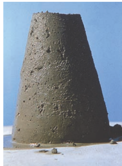
Figure 9-3. Concrete of a stiff consistency (low slump) is suitable for a paving or slip-form applications.
