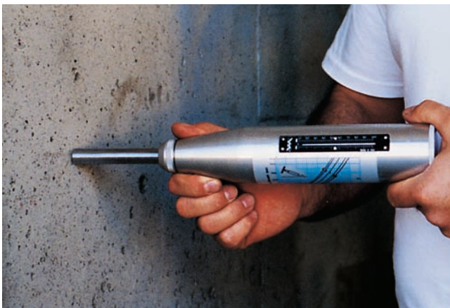
Figure 18-26. The rebound hammer gives an indication of the uniformity of concrete.
