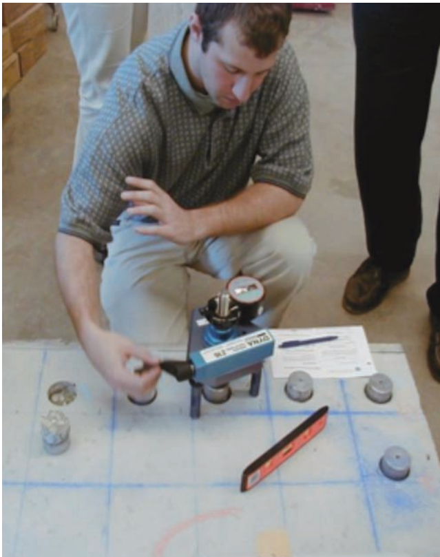
Figure 18-31. Demonstration of pull-off test to measure the strength of the concrete substrate before application of an overlay or repair material (photo courtesy of N. Carino).
