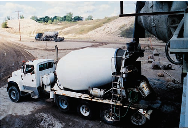
Figure 13-4. Central mixing in a stationary mixer of the tilting drum type with delivery by a truck mixer operating at agitating speed.
