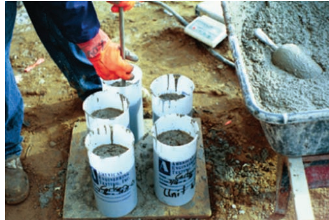
Figure 18-10. Preparing standard test specimens for compressive strength of concrete.
