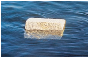
Figure 20-6. (top) Residential building constructed with autoclaved cellular concrete blocks. (bottom) Autoclaved cellular concrete block floating in water.
