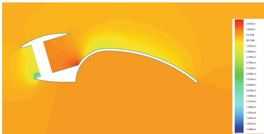
Fig. 17 Pressure contours in the flow field
